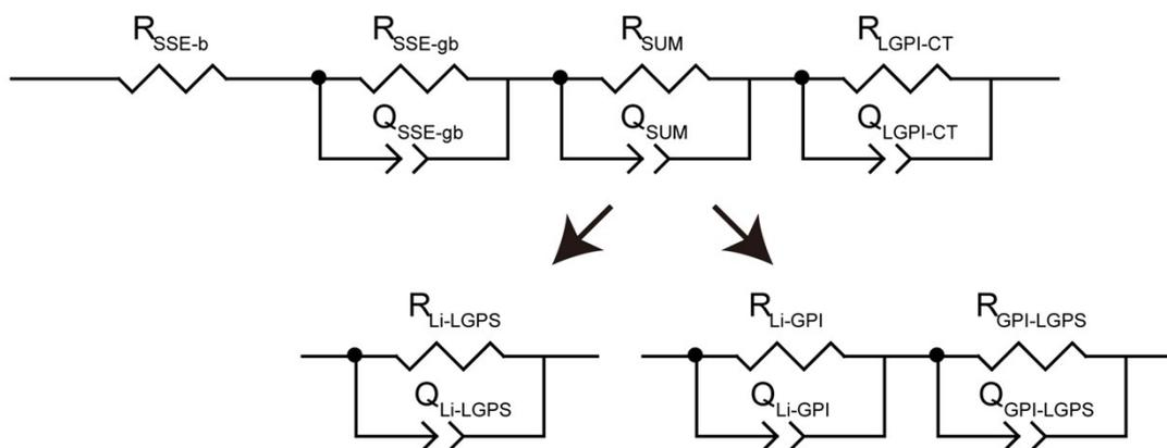
**Figure S6.** Detailed equivalent circuit of Figure 4c, d, where  $R_{SSE-b}$  is the bulk resistance,  $R_{SSE-gb}$  is the grain-boundary resistance of LGPS,  $R_{Li-LGPS}$ ,  $R_{Li-GPI}$ ,  $R_{GPI-LGPS}$  is the Li/LGPS, Li/GPI, GPI/LGPS interphase resistance, respectively.  $R_{LGPI-CT}$  is the electrochemical transfer polarization resistance of Li plating/stripping. Each constant phase element (CPE) describes the capacitance of the corresponding process.
