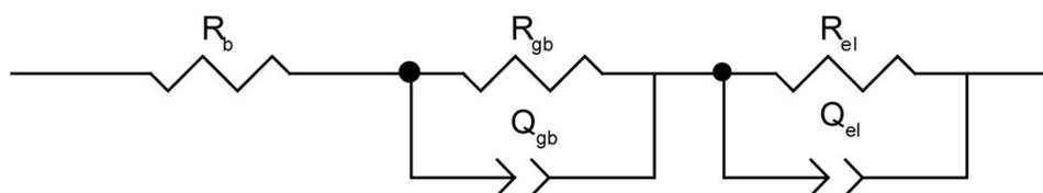
**Figure S2.** Detailed equivalent circuit of Figure 2b, where R<sub>b</sub> is the bulk resistance, R<sub>gb</sub> is the grain-boundary resistance of LGPS powder and R<sub>el</sub> is the resistance of blocking electrode. Each constant phase element (CPE) describes the capacitance of the corresponding process.
