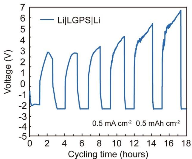
**Figure S4.** Galvanostatic Li plating/stripping overpotential profiles of symmetrical Li|LGPS|Li cells at current density of  $0.5 \text{ mA cm}^{-2}$  with a fixed capacity of  $0.5 \text{ mAh cm}^{-2}$  at room temperature.
