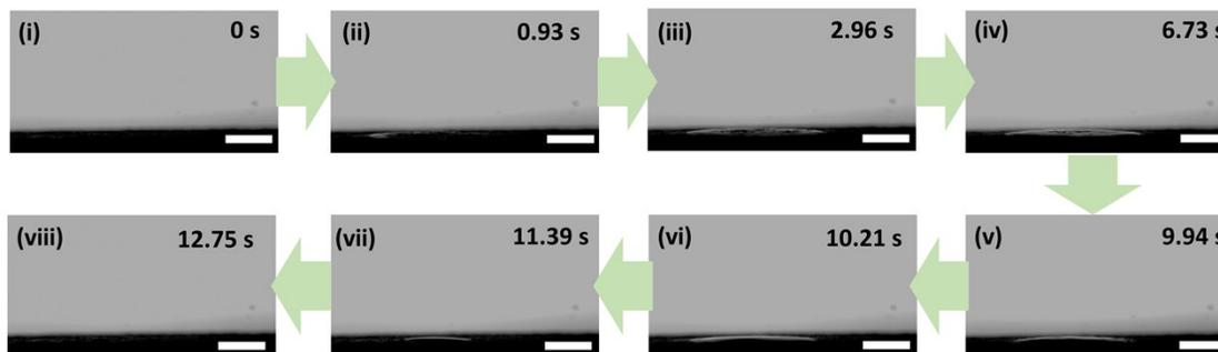
Figure S3. Magnet-responsiveness of ferrofluid on semi-infused adaptive surface: (i)-(iv) applying the magnet; (v)-(viii) withdrawing the magnet. Scale bar: 2 mm.
