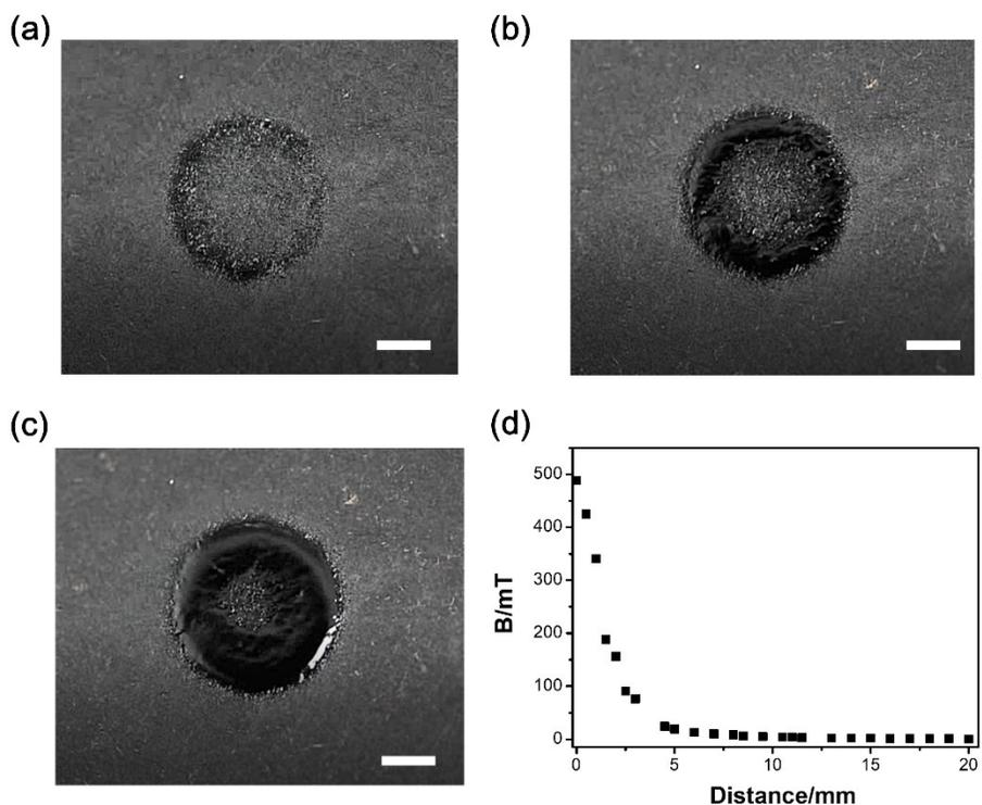
Figure S4. Accumulation of ferrofluid on semi-infused surface when applied with different magnetic fields. (a) Ferrofluid spot occurs on the adaptive surface with a magnetic intensity of 10 mT. (b) Ferrofluid begins to form a “basin” when magnetic intensity increases to 76 mT. (c) Ferrofluid “basin” expands as increasing the magnetic intensity (425 mT). (d) Relationship of the magnetic intensity to the distance between the magnet and the membrane. Scale bar in (a), (b) and (c) is 2 mm.
