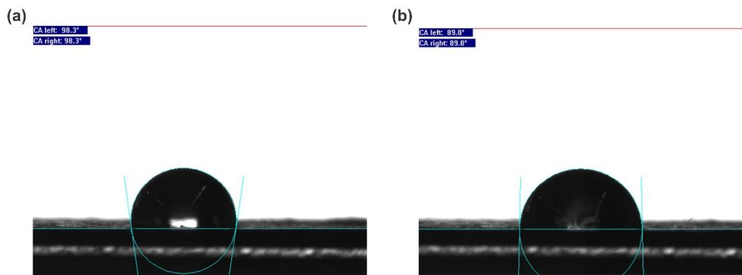
Figure S7. Water contact angle of water droplet on the flat semi-infused adaptive surface in the intact and processed state, respectively.
