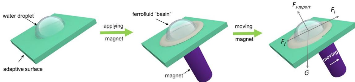
Figure S9. Force analysis of droplet manipulation on the tilted surface. When the applied magnet moved upwards, the droplet was subjected to force balance under gravity ( $G$ ), friction force ( $F_f$ ), support force ( $F_{support}$ ) and interfacial force ( $F_i$ ). The interfacial force leads the uphill of a droplet.
