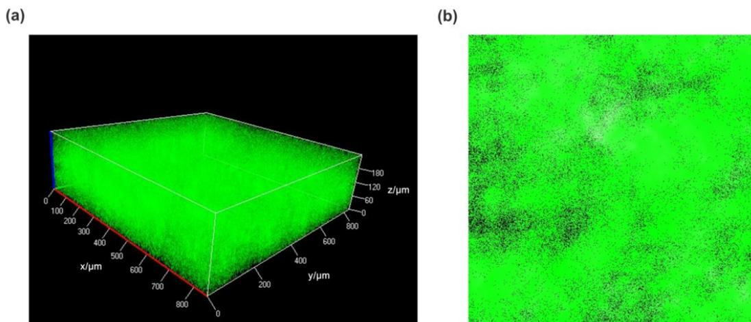
Figure S2. Confocal images of PDI-conjugated silicone oil dipped full-infused surface. (a) 3D stacked full-infused surface. (b) Top view.
