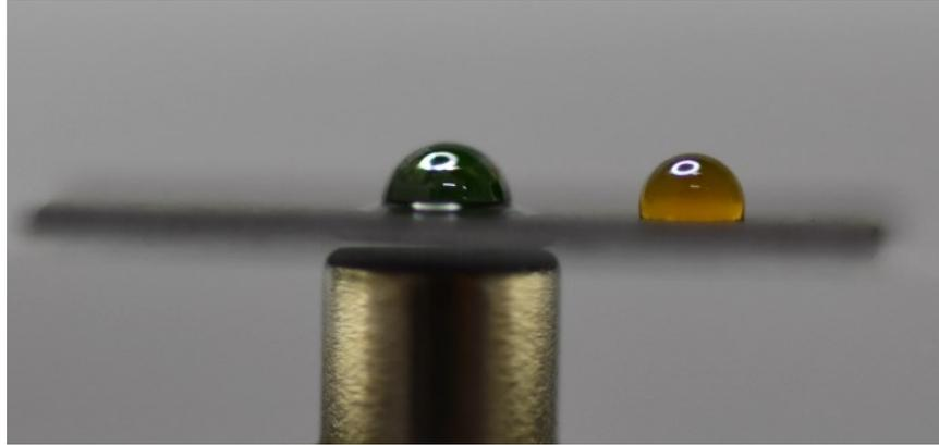
Figure S8. Droplets on semi-infused adaptive surface with and without magnetic field.
