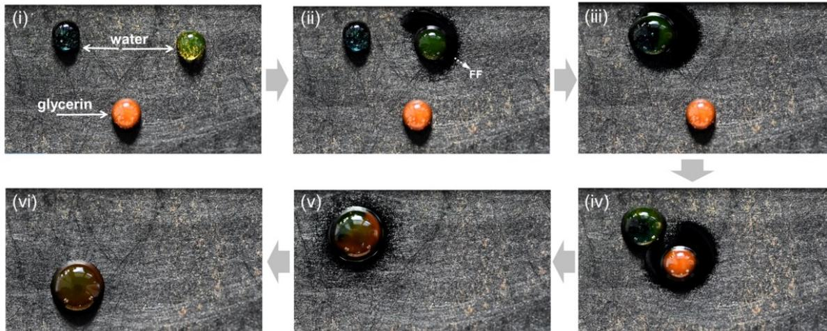
Figure S10. Droplet manipulation between water droplets and glycerin droplet. (i) Water and glycerin-based droplets pinned on the semi-infused adaptive surface. (ii) Yellow droplet was applied with a magnet and moved toward the blue one. (iii) Merging of blue and yellow water droplets. (iv) Glycerin-based droplet was applied with a magnet and moved toward the merged water droplet. (v) Droplet merging between water and glycerin droplets. (vi) Merged droplet after withdrawn the magnet.
