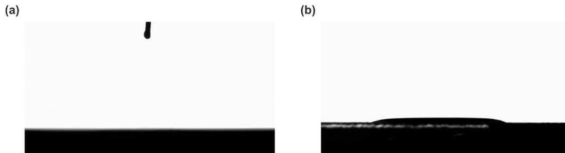
Figure S6. Ferrofluid-substrate angle of ferrofluid on flat PP membrane in the intact state (a) and (b) activated state (b).
