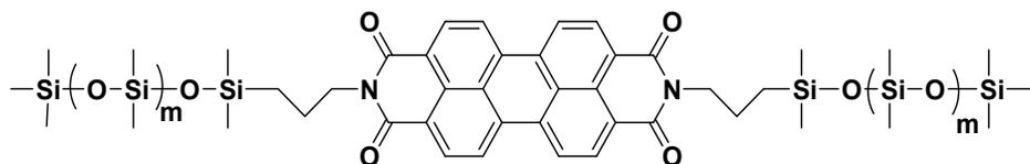
Figure S1. Structures of perylene diimide (PDI) conjugated silicone oil.
