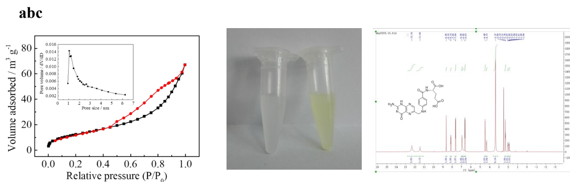
Figure S1 The \text{N}_2 adsorption-desorption isotherms of \text{CaCO}_3 with an inset showing the pore size distribution obtained by the BJH method (a). Images of \text{CaCO}_3 and \text{CaCO}_3@FA (b); ^1\text{H} NMR spectrum of FA in the supernate of \text{CaCO}_3@FA (c).
