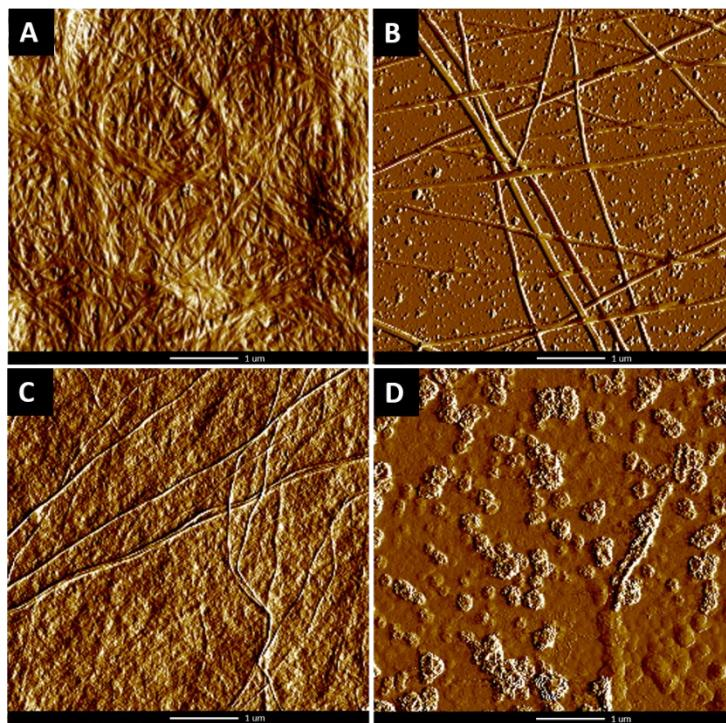
**Figure S4.** AFM images of 10mM Fmoc-FF hydrogels; A) 25 mM  $\text{CaCO}_3$ ; B) 25 mM  $\text{CaCO}_3$  prepared at 1/100 dilution in deionized water; C) 25 mM  $\text{Cs}_2\text{CO}_3$ ; D) 25 mM  $\text{Cs}_2\text{CO}_3$  prepared at 1/100 dilution in deionized water.
