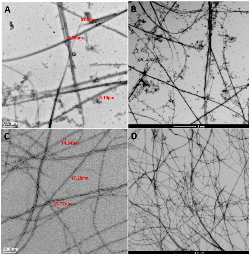
**Figure S3.** HR-TEM images; (A-B) 10 mM of Fmoc-FF and 25mM of  $\text{Na}_2\text{CO}_3$  hydrogels, (C-D); 10 mM of Fmoc-FF and 25mM of  $\text{CaCO}_3$  hydrogels.
