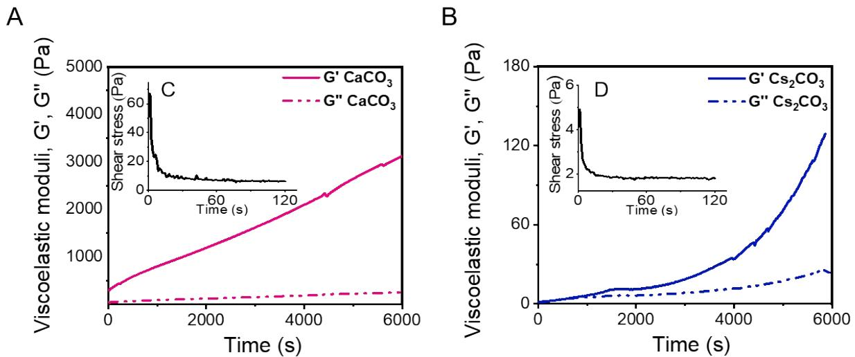
**Figure S9.** Self-healing of Fmoc-FF  $\text{Ca}^{2+}$  (10 mM) (A) and Fmoc-FF  $\text{Cs}^+$  (10 mM) (B). (A) and (B) show the evolution of the viscoelastic moduli after fracture of the hydrogels by 120 s of shearing at a constant shear rate of  $20 \text{ s}^{-1}$ . (C) and (D) show the evolution of the shear stress,  $\tau$ , during the shearing at constant shear rate -observe that the shear stress decreased strongly upon fracture of the hydrogels.
