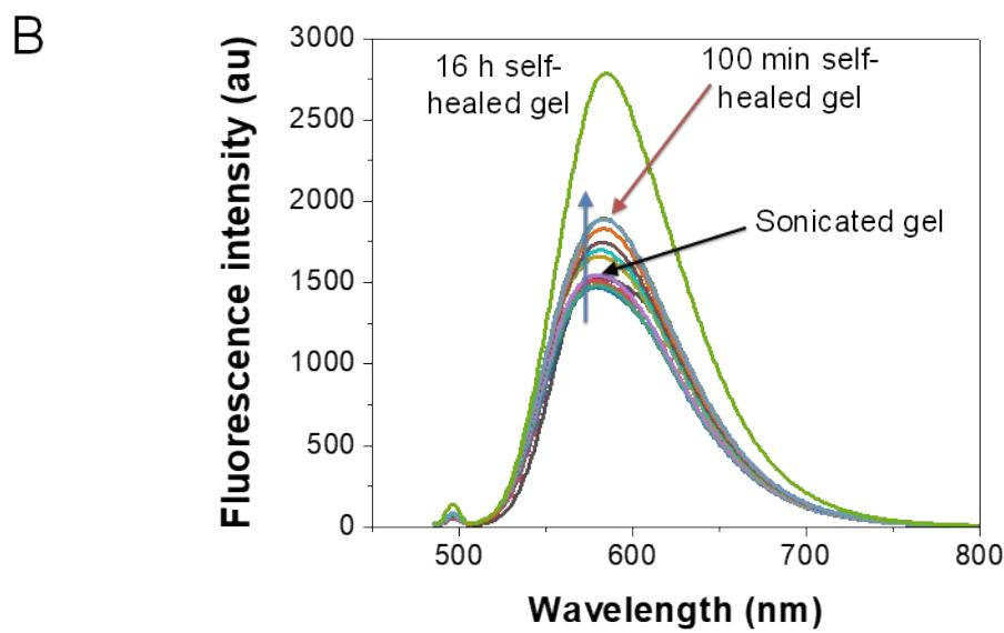
**Figure S8.** Time recovery of the emission spectra ( $\lambda_{\text{ex}} = 470 \text{ nm}$ ) of AQui in Fmoc-FF  $\text{Ca}^{2+}$  (A) and Fmoc-FF  $\text{Cs}^+$  (B) gels, after ultrasound treatment.
