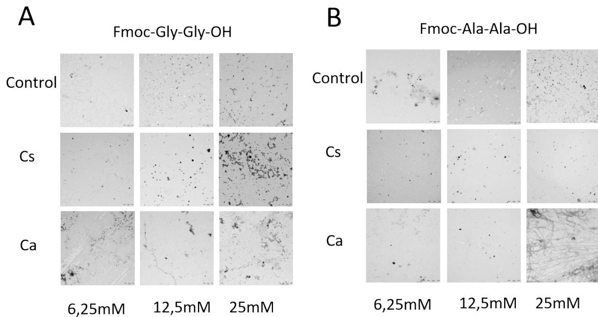
**Figure S5.** TEM images peptide hydrogels at different concentrations of peptide-salt: 2.5/6.25 mM, 5/12.5 mM and 10/25 mM; A) Fmoc-GG peptide with  $\text{Cs}_2\text{CO}_3$  and  $\text{CaCO}_3$  salts; B) Fmoc-AA with  $\text{Cs}_2\text{CO}_3$  and  $\text{CaCO}_3$  salt. In the case of Fmoc-GG the formation of fibers were not
