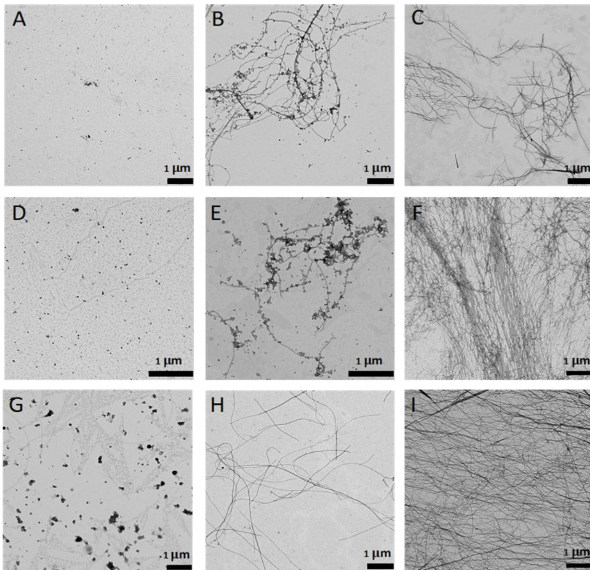
**Figure S1.** TEM Images of Fmoc-FF  $\text{Na}^+$  salt at 2.5 mM (A), 5 mM (B) and 10 mM (C); TEM images of Fmoc-FF  $\text{Cs}^+$  salt at 2.5 mM (D), 5 mM (E) and 10 mM (F); TEM images of Fmoc-FF  $\text{Ca}^{2+}$  salt at 2.5 mM (G), 5 mM (H) and 10 mM (I) peptide conc.
