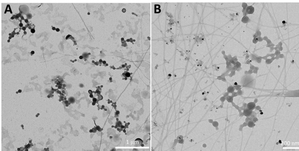
**Figure S2.** TEM images of liquid-liquid phase formed by Fmoc-FF hydrogels in the presence of  $\text{CaCO}_3$  (A) and Fmoc-AA in the presence of  $\text{Ag}_2\text{CO}_3$  (B). It has been reported that Fmoc-AA in the presence of  $\text{Ag}_2\text{CO}_3$  forms liquid-liquid phases.<sup>S5</sup> We show in here as a control to demonstrate that similar structures are formed using  $\text{CaCO}_3$  in our conditions and visualized with the same TEM apparatus.
