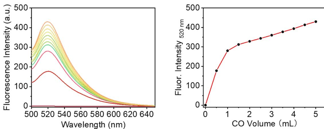
**Figure S4.** The fluorescence of FL-CO towards different concentration CO and plot of fluorescence at 520 nm.
