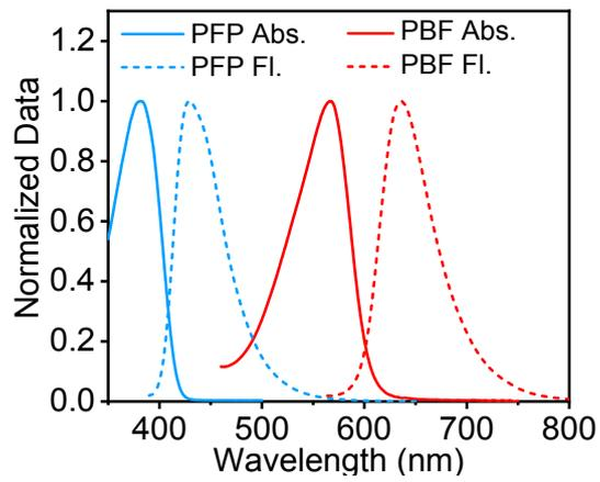
**Figure S1.** Absorption and fluorescence spectra of PFP and PBF.
