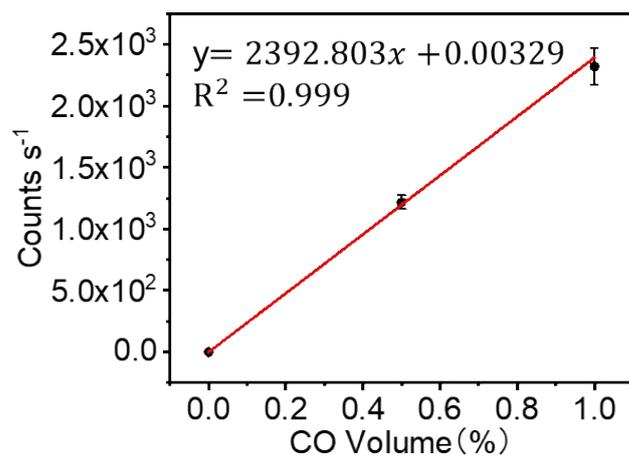
**Figure S3.** Standard curve of CO was tested by GC.
