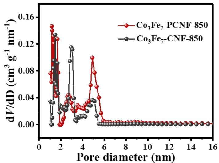
Fig. S8 Pore size distribution of Co<sub>3</sub>Fe<sub>7</sub>-PCNF-850 and Co<sub>3</sub>Fe<sub>7</sub>-CNF-850.
