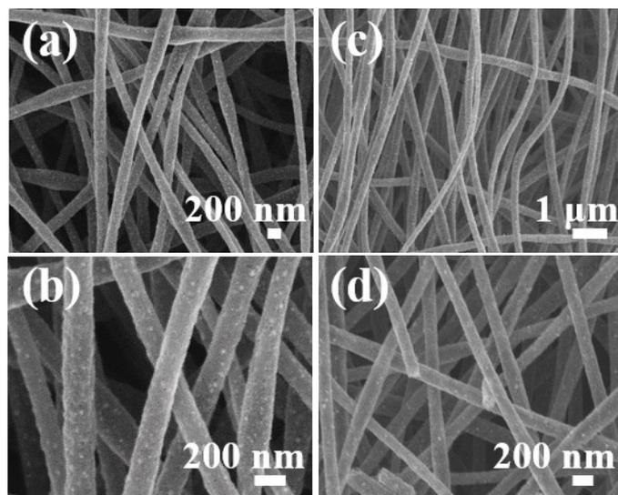
Fig. S10 (a, b) SEM images of  $\text{Co}_3\text{Fe}_7\text{-PCNF-800}$ , (c, d) SEM images of  $\text{Co}_3\text{Fe}_7\text{-PCNF-900}$ .
