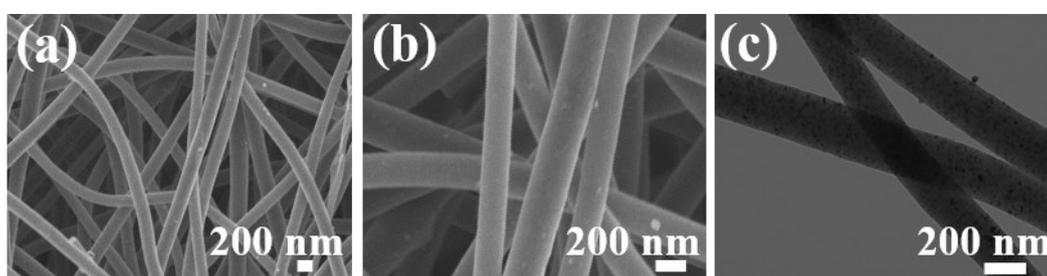
Fig. S2 (a, b) SEM images, (c) TEM image of  $\text{Co}_3\text{Fe}_7\text{-CNF-850}$ .
