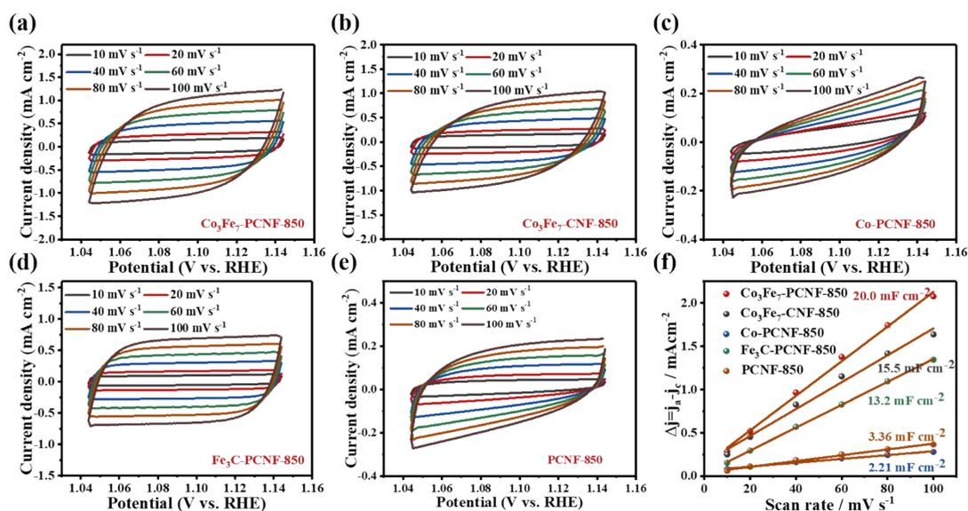
Fig. S13 (a-e) CVs at different scan rates of catalysts and (f) the corresponding  $C_{dl}$ .
