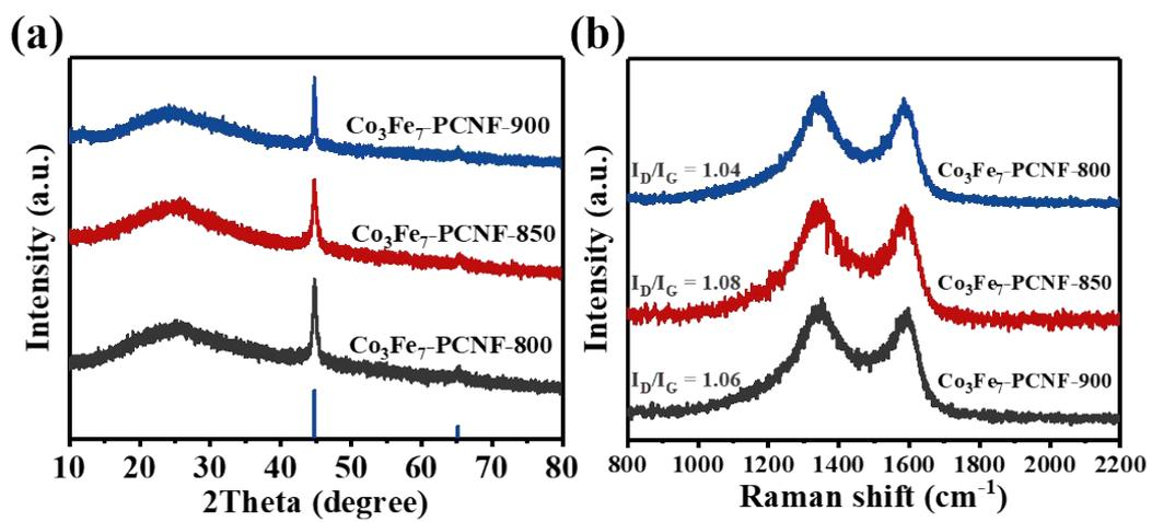
Fig. S11 (a) XRD patterns; (b) Raman spectra of electrocatalysts with different temperatures.
