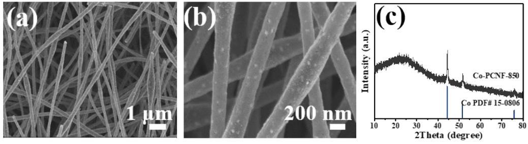
Fig. S6 (a, b) SEM images of Co-PCNF-850, (c) XRD patterns of Co-PCNF-850.
