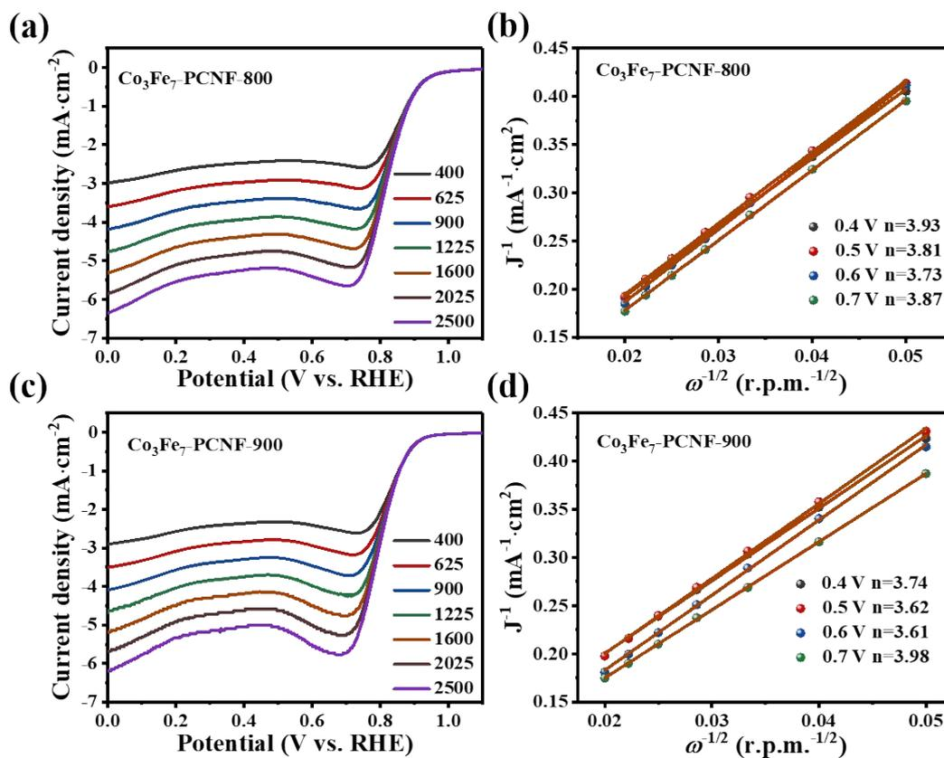
Fig. S19 LSV curves of catalysts in  $\text{O}_2$ -saturated 0.1 M KOH solution under different rotating speeds and their corresponding K-L plots.
