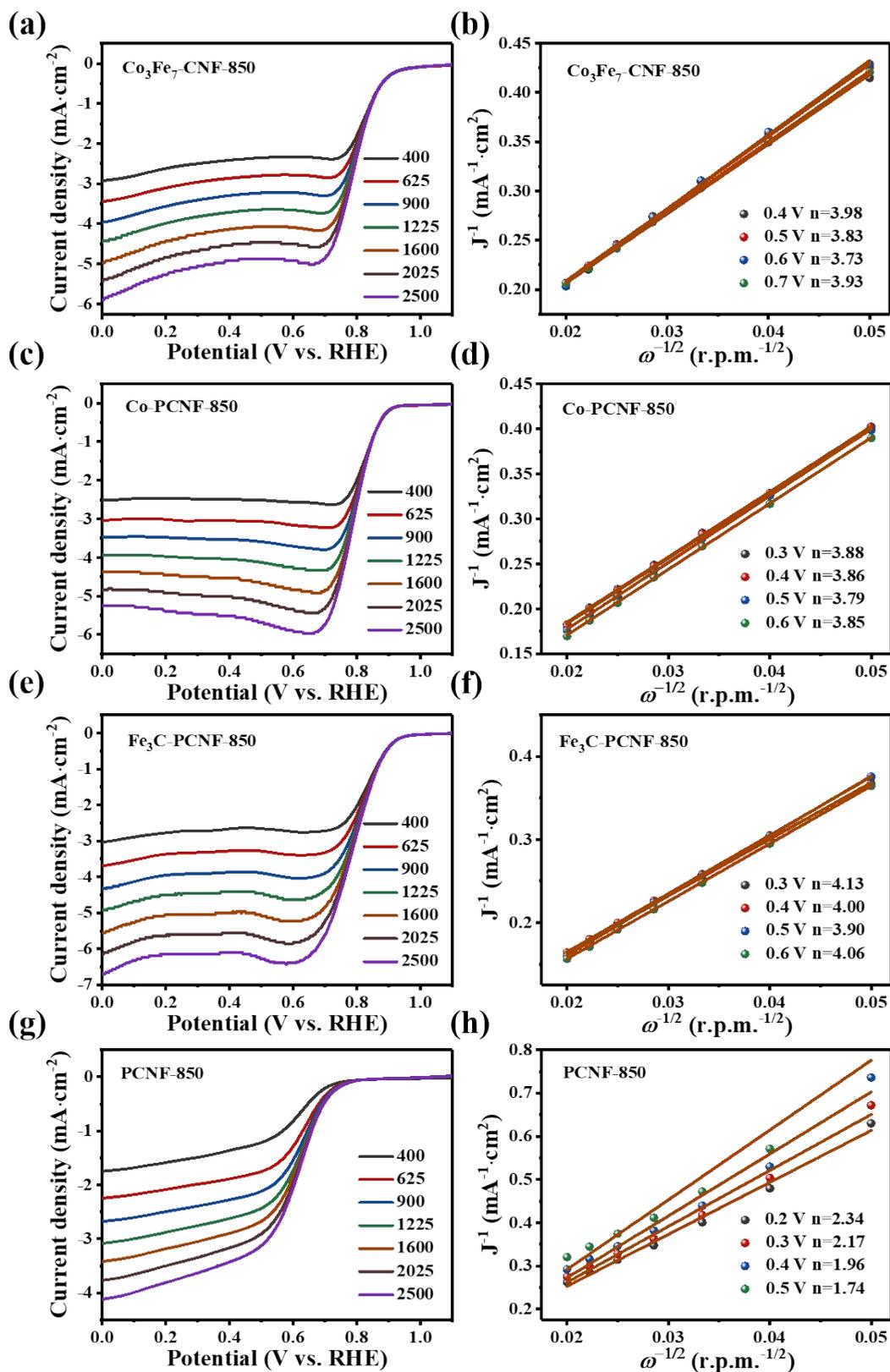
Fig. S14 LSV curves of catalysts in  $O_2$ -saturated 0.1 M KOH solution under different rotating speeds and their corresponding K-L plots.
