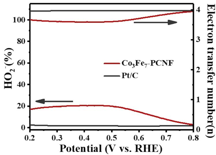
Fig. S15  $\text{HO}_2^-$  yield and the corresponding electron transfer number ( $n$ ) of  $\text{Co}_3\text{Fe}_7$ -PCNF-850 and Pt/C.
