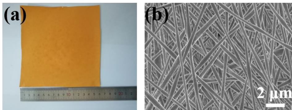
Fig. S1 (a) Digital photo and (b) SEM images of the electrospun nanofiber film.
