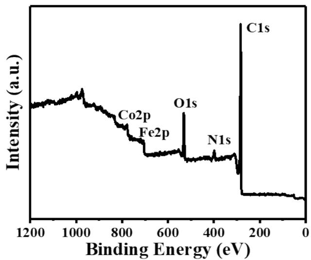
Fig. S9 Survey XPS spectra of Co<sub>3</sub>Fe<sub>7</sub>-PCNF-850.
