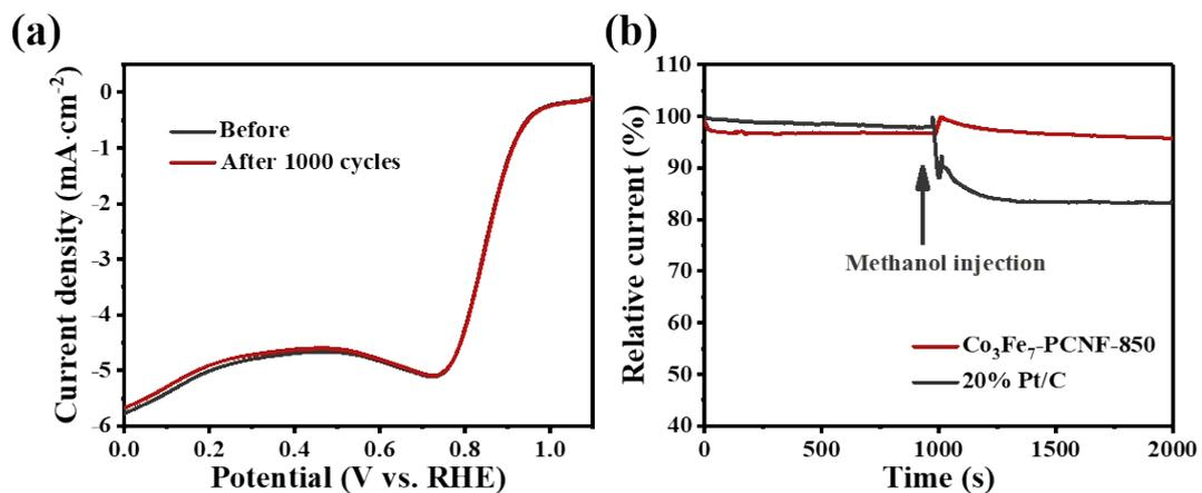
Fig. S17 (a) LSV curves of Co<sub>3</sub>Fe<sub>7</sub>-PCNF-850 before and after 1000 cycles cyclic voltammetry test; (b) Chronoamperometric response at 0.4 V vs. RHE after the introduction of 2 M methanol solution into 0.1 M KOH solution.
