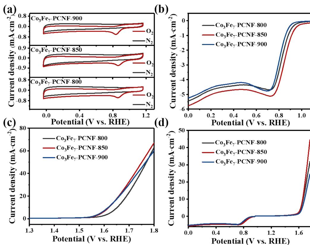
Fig. S18 Electrochemical performance of different temperature products. (a) CV curves in N<sub>2</sub> or O<sub>2</sub> saturated 0.1 M KOH solution. (b) LSV polarization curves for ORR (1600 rpm). (c) LSV polarization curves for OER. (d) Overall Polarization curves of as-prepared catalysts for bifunctional catalytic activity.
