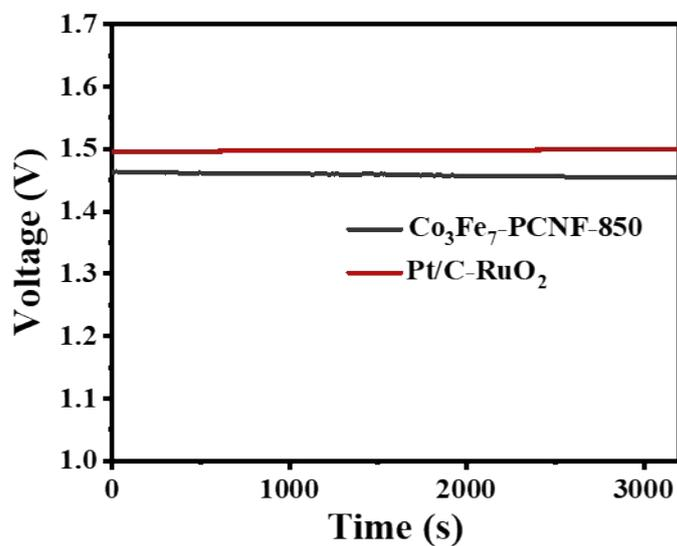
Fig. S21 Open-circuit potential of Co<sub>3</sub>Fe<sub>7</sub>-PCNF-850 assembled liquid zinc air battery.
