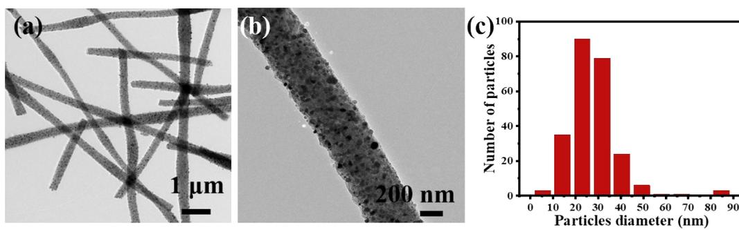
Fig.S5 (a, b) TEM images of Co<sub>3</sub>Fe<sub>7</sub>-PCNF-850. (c) shows the particle size distribution of Co<sub>3</sub>Fe<sub>7</sub> nanoparticles(b).
