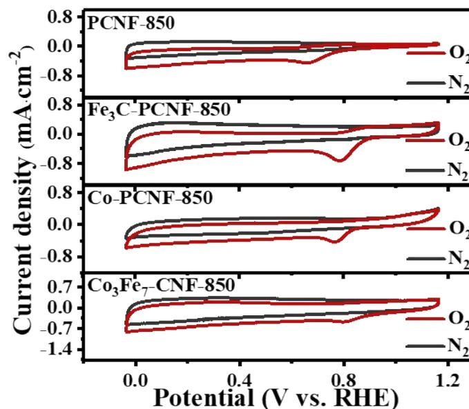
Fig. S12 Cycle voltammetry curves in 0.1 M KOH saturated with  $N_2$  or  $O_2$ .
