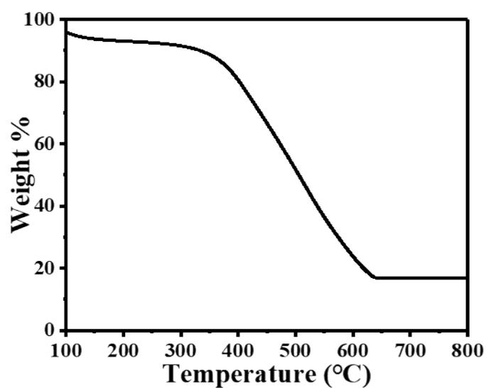
Fig. S3 TG curves of  $\text{Co}_3\text{Fe}_7\text{-PVP}$  fibers in  $\text{N}_2$ .
