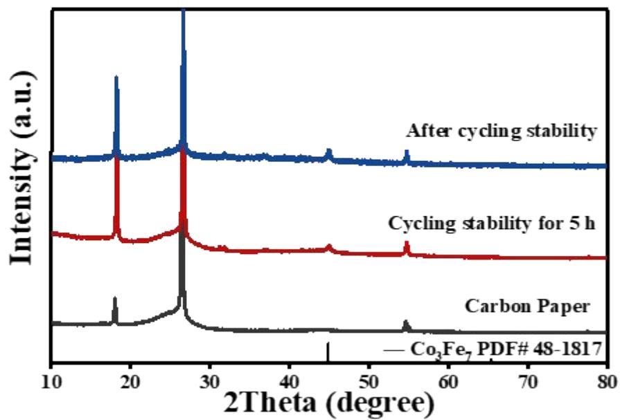
Fig. S22 XRD patterns of Co<sub>3</sub>Fe<sub>7</sub>-PCNF-850 based battery after cycling stability.
