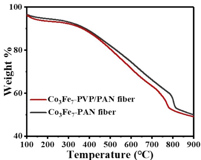
Fig. S4 TG curves of Co<sub>3</sub>Fe<sub>7</sub>-PVP/PAN fiber and Co<sub>3</sub>Fe<sub>7</sub>-PAN fiber in N<sub>2</sub>.
