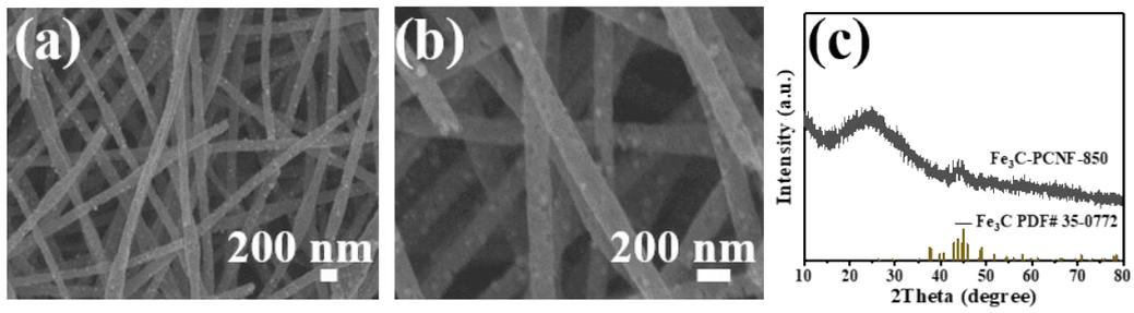
Fig. S7 (a, b) SEM images of Fe<sub>3</sub>C-PCNF-850, (c) XRD patterns of Fe<sub>3</sub>C-PCNF-850.
