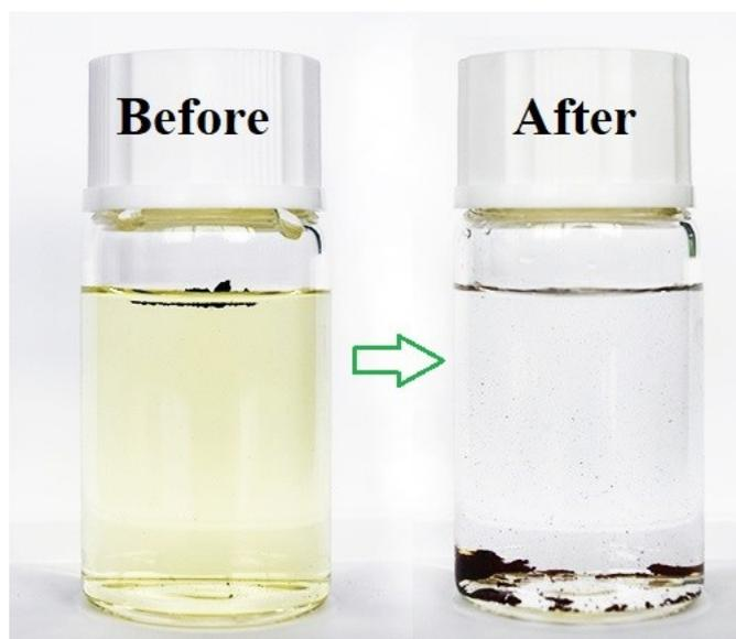
Figure S9. The images of the color change observed for the conversion of 4-nitrophenol to 4-aminophenol after the addition of AgNPs@NCOF catalyst after 3 minutes.
