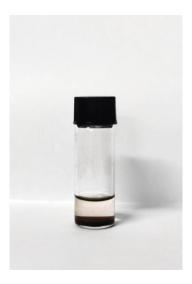
Figure S1. Photograph of 20 mg PIF suspended in 2 mL of blank electrolyte.
