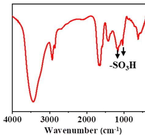
**Figure S2** Fourier transform infrared spectroscopy (FITR) of Pol. The peaks emerging at 1036 cm<sup>-1</sup> and 1167cm<sup>-1</sup> (indicating arrows) are characteristic peaks of sulfonic acid group<sup>1</sup>.
