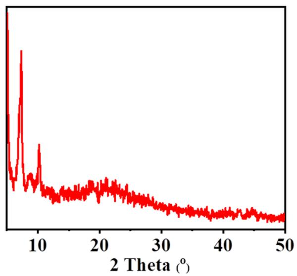
**Figure S4** X-ray diffraction (XRD) curve of PPNUH.
