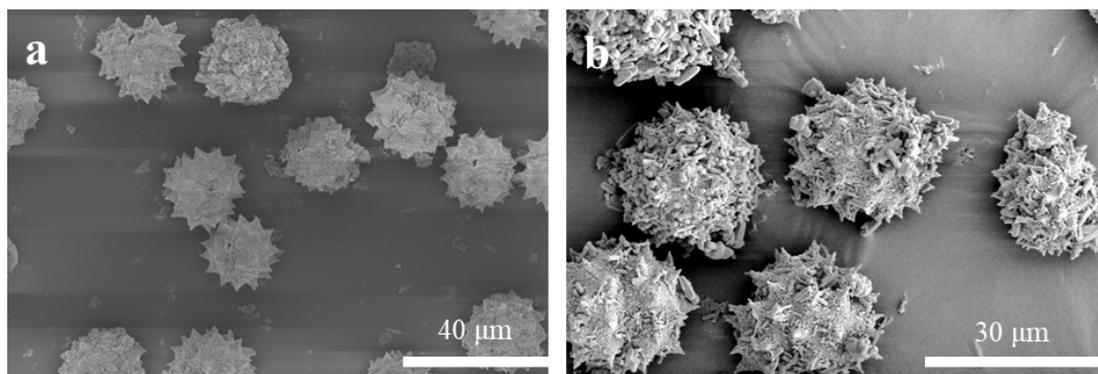
**Figure S3** a) Typical SEM image of PPNUH. b) Typical SEM image of PPNUH after 24-h incubation of PPNUH in PCS solution.
