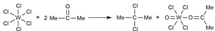
Figure S4. Reactions of \text{WCl}_6 with pure (a) EtOH and (b) acetone.
