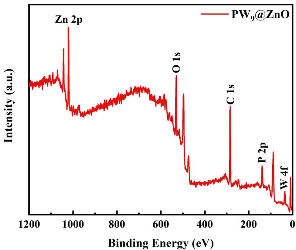
Figure S7. XPS full spectrum of PW<sub>9</sub>@ZnO NWs.
