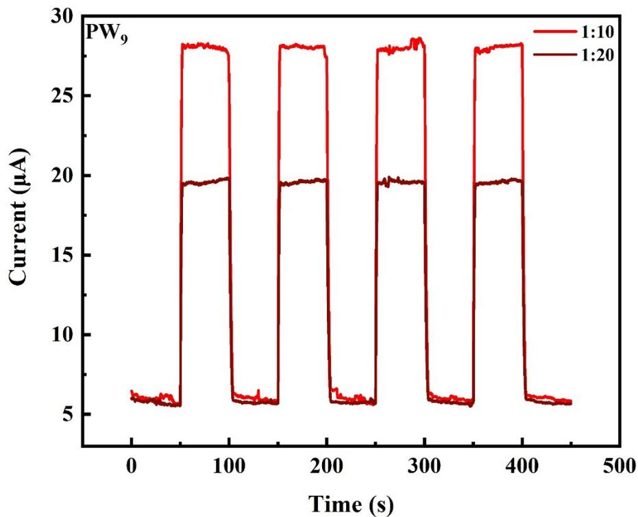
Figure S15. The I-t curve of the photodetector when the mass doping ratio of  $PW_9$  is 1:10 and 1:20 (spinning time 1 min).
