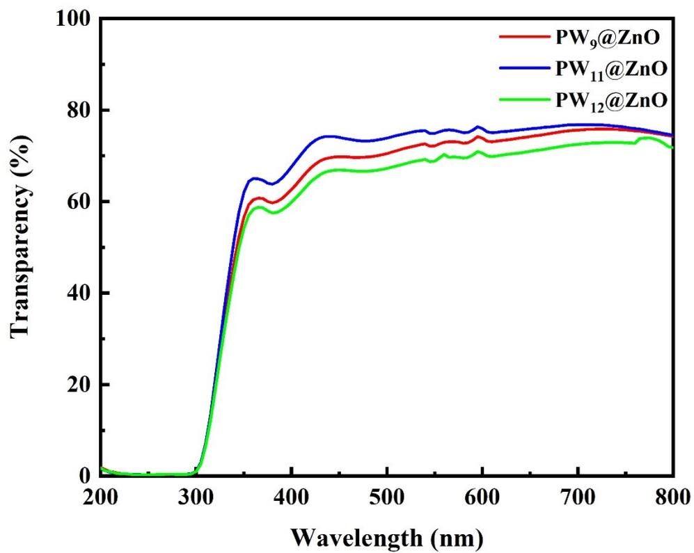
Figure S5. Light transmittance of POMs@ZnO NWs device.
