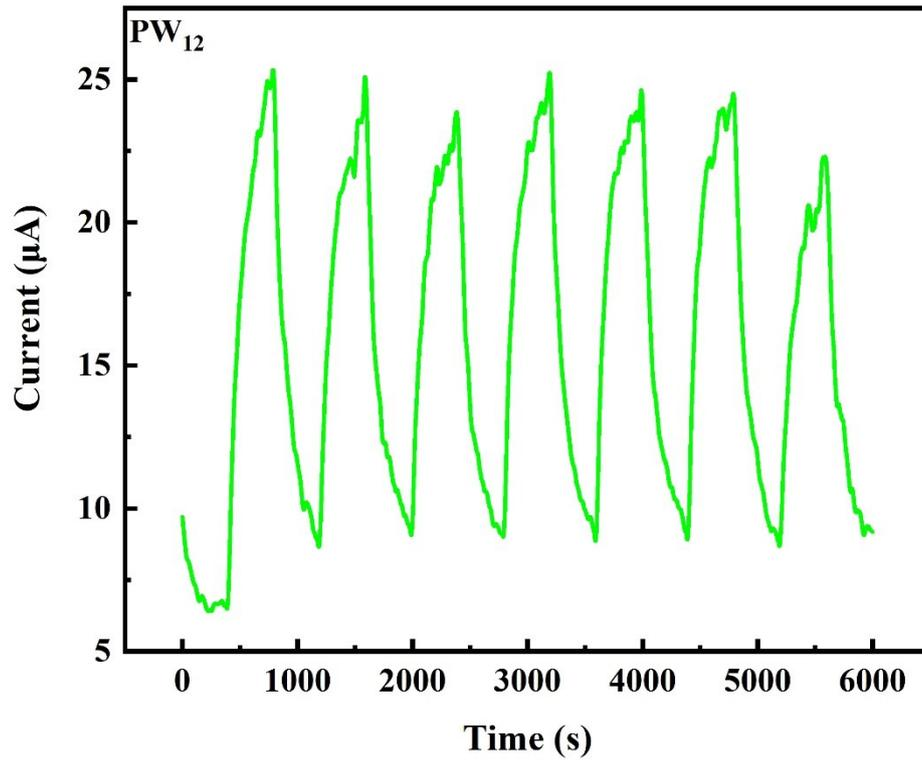
**Figure S16.** I-t curve of the photodetector when the mass doping ratio of PW<sub>12</sub> is 1:15 (spinning time 1 min).
