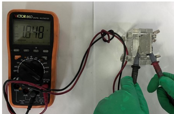
Figure S9. Picture of open-circuit voltage measurement of FeCo-NC-assembled Al-air battery.
