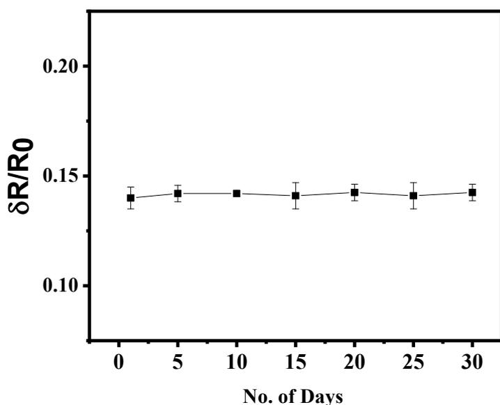
Figure S1. Stability and reusability test of FET biosensor for 30 days.
