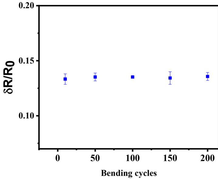
Figure S2. Flexibility studies of FET biosensor for over 200 cycles.
