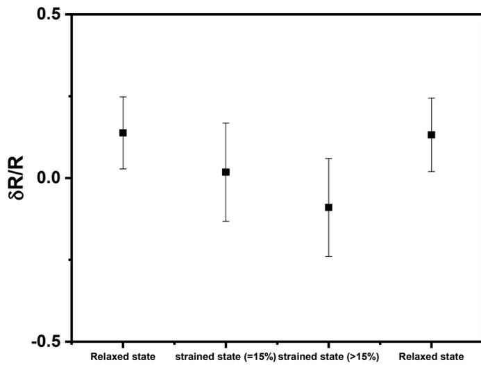
Figure S3. The normalised response of the sensor under relaxed state and strained conditions
