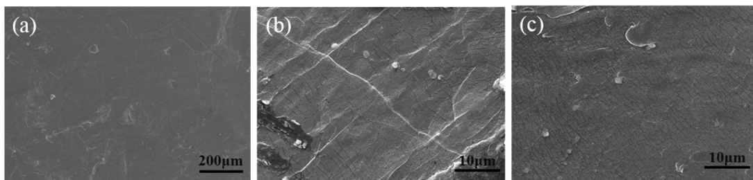
Fig. S1 Surface morphology of Li metal anode: (a) before galvanostatic cycling, (b) after 200h cycling and (c) after 800h cycling at 0.05\text{mA}\cdot\text{cm}^{-2} .
