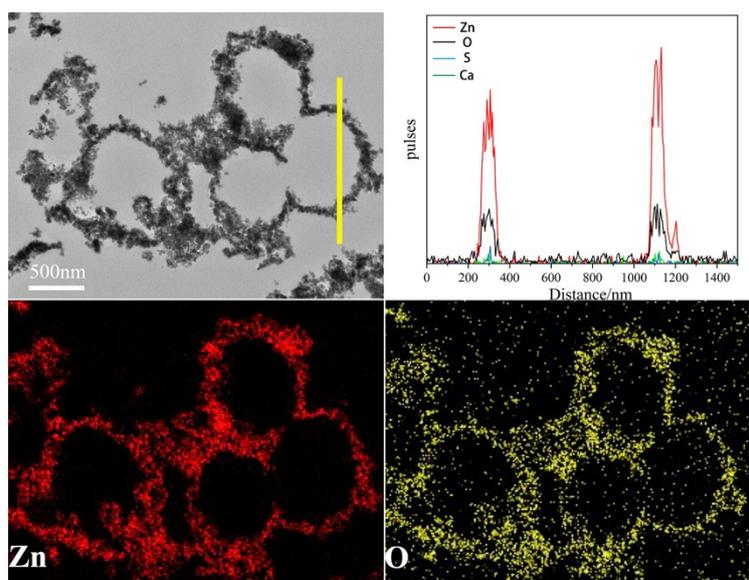
**Fig. S5** TEM and EDX elemental mapping of the ZnO hollow microspheres.
