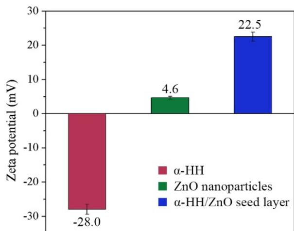
**Fig. S7** Zeta ( $\zeta$ ) potentials of  $\alpha$ -HH microspheres, ZnO nanoparticles and  $\alpha$ -HH/ZnO seed layers.
