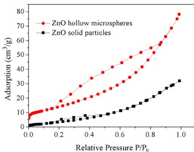
**Fig. S9** N<sub>2</sub> adsorption-desorption isotherm (BET) of the ZnO hollow microspheres and ZnO solid particles.
