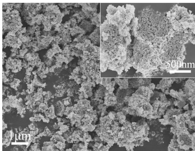
**Fig. S2** Fragments of ZnO seed layers after dissolving  $\alpha$ -HH microspheres coated with seed layers of ZnO in water.
