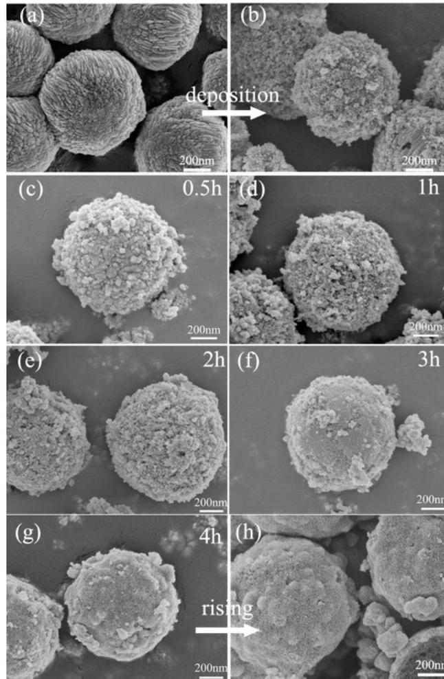
**Fig. S3** SEM images of the  $\alpha$ -HH microspheres (a),  $\alpha$ -HH/ZnO seeds (b),  $\alpha$ -HH/ZnO core-shell microspheres after 2nd deposition-precipitation for 0.5h(c), 1h(d), 2h(e), 3h(f), 4h(g), (h)ZnO hollow microspheres after  $\alpha$ -HH microspheres template removal by water rinse.
