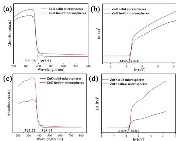
**Fig. S8** The UV-vis diffuse reflectance spectra (a,c) and Tauc's plot (b,d) for ZnO hollow microspheres and ZnO solid microspheres in the two parallel experiments.
