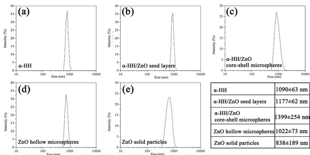
**Fig. S1** Particle size distribution of (a)  $\alpha$ -HH, (b)  $\alpha$ -HH/ZnO seed layers, (c)  $\alpha$ -HH/ZnO core-shell microspheres, (d) ZnO hollow microspheres and (e) ZnO solid particles.
