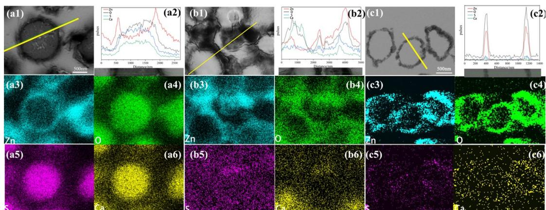
**Fig. S4** SEM (a1) and elemental line scanning (a2) and EDX-mapping (a3-a6) of the sliced  $\alpha$ -HH/ZnO core-shell microspheres; SEM (b1) and elemental line scanning (b2) and EDX-mapping (b3-b6) of the sliced  $\alpha$ -HH/ZnO core-shell during rinsing process, SEM (c1) and elemental line scanning (c2) and EDX-mapping (c3-c6) of the sliced ZnO hollow microspheres.
