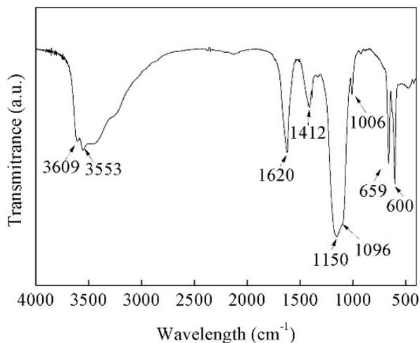
**Fig. S6** FTIR spectra of  $\alpha$ -HH microspheres.
