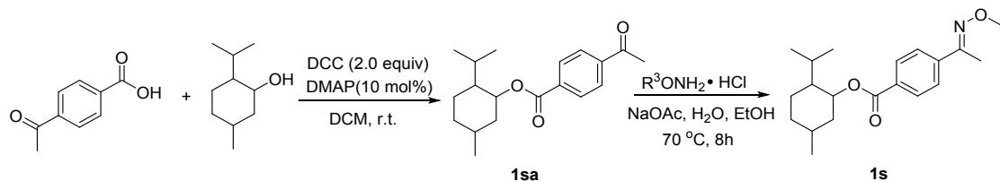
A round-bottom flask was charged with 4-Acetylbenzoic acid (1.0 equiv.), N, N'-Dicyclohexylcarbodiimide (2.0 equiv.) and 4-dimethylaminopyridine (0.1 equiv.), Dichloromethane (20 mL) was added and the mixture was stirred vigorously in ice bath. Then DL-Menthol 1.7 g (1.1 equiv.) was slowly added and the mixture was allowed to stir until the acid was consumed (determined by TLC). The combined
