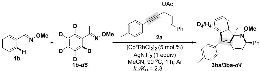
A sealed tube containing **1a** (30.1 mg, 0.2 mmol), **1a-d5** (29.9 mg, 0.2 mmol), **2a** (58.2 mg, 0.24 mmol),  $[\text{Cp}^*\text{RhCl}_2]_2$  (5.3 mg, 5 mol %) and  $\text{AgNTf}_2$  (76.3 mg, 1 equiv) was evacuated and purged with argon gas three times. Then MeCN (2 mL) was added via syringe under argon atmosphere and the reaction mixture was allowed to stir at 90 °C for 1 h. Then, the mixture was cooled, ethyl acetate (15 mL) was added,
