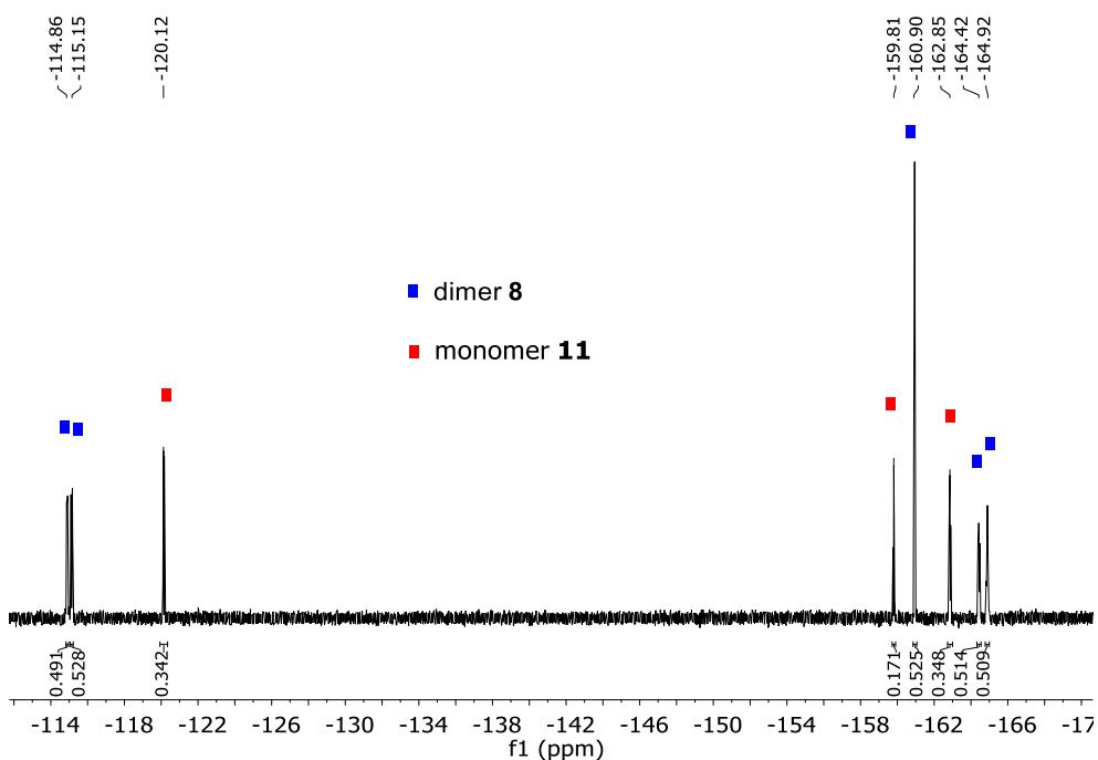
**Figure S39.**  $^{19}\text{F}$  NMR (470.17 MHz,  $\text{CD}_2\text{Cl}_2$ ) of the mixture formed after complex  $[\text{Pd}_2(\text{bipy-6-O})_2(\text{C}_6\text{F}_5)_2\mu\text{OH}_2]$  (**8**) is dissolved in  $\text{CD}_2\text{Cl}_2$ . The red species corresponds to the monomer species  $[\text{Pd}(\text{bipy-6-O})(\text{C}_6\text{F}_5)(\text{H}_2\text{O})]$ . Ratio dimer **8:11** = 1:1.
