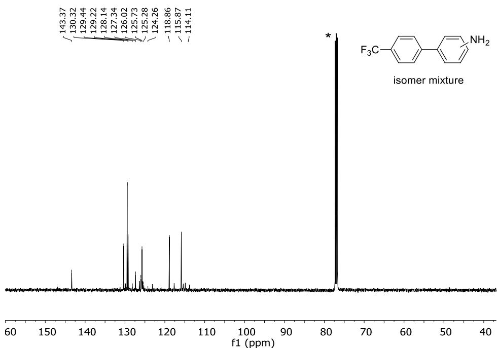
**Figure S25.**  $^{13}\text{C}\{\text{H}\}$  NMR (125.67 MHz,  $\text{CDCl}_3$ ) of an isomer mixture of 4'-(trifluoromethyl)-[1,1'-biphenyl]-2-amine, 4'-(trifluoromethyl)-[1,1'-biphenyl]-4-amine and 4'-(trifluoromethyl)-[1,1'-biphenyl]-3-amine (12:1:2) at 298 K. \* Signal corresponding to the solvent (chloroform).
