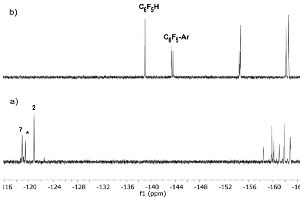
**Figure S1.**  $^{19}\text{F}$  NMR spectra in benzonitrile as solvent using a DMSO-d6 capillary. a) Complex **2** in benzonitrile. \* Unknown species. b) Mixture obtained after heating complex **2** for 1 h at 130 °C ( $\text{C}_6\text{F}_5\text{-Ar}$  is a mixture of two isomers). Only the  $^{19}\text{F}_{\text{ortho}}$  region is labeled for clarity (Ar =  $\text{C}_6\text{H}_4\text{CN}$ ).
