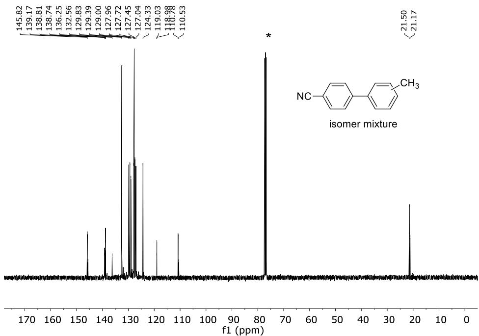
**Figure S16.**  $^{13}\text{C}\{^1\text{H}\}$  NMR (125.67 MHz,  $\text{CDCl}_3$ ) of an isomer mixture of 3'-methyl-[1,1'-biphenyl]-4-carbonitrile and 4'-methyl-[1,1'-biphenyl]-4-carbonitrile (1.7:1) at 298 K. \* Signal corresponding to the solvent (chloroform).
