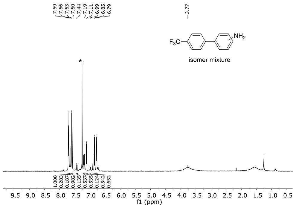
**Figure S23.**  $^1\text{H}$  NMR (499.73,  $\text{CDCl}_3$ ) of an isomer mixture of 4'-(trifluoromethyl)-[1,1'-biphenyl]-2-amine, 4'-(trifluoromethyl)-[1,1'-biphenyl]-4-amine and 4'-(trifluoromethyl)-[1,1'-biphenyl]-3-amine (12:1:2) at 298 K. \* Signal corresponding to the solvent (chloroform).
