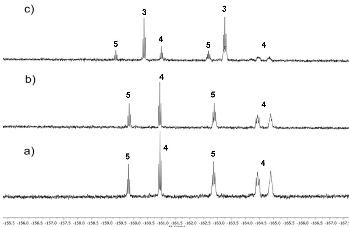
**Figure S7.**  $^{19}\text{F}$  NMR spectra (para and meta region) in  $\text{CD}_2\text{Cl}_2$ . a) Complex **4** dissolved in  $\text{CD}_2\text{Cl}_2$ . b) Mixture obtained after adding 10  $\mu\text{L}$  of pinacolone to complex **4** solution in  $\text{CD}_2\text{Cl}_2$  (ratio Pd:pinacolone = 1:10). c) Mixture obtained after adding 0.5 mL of pinacolone to complex **4** in  $\text{CD}_2\text{Cl}_2$  (ratio Pd:pinacolone = 1:1000).
