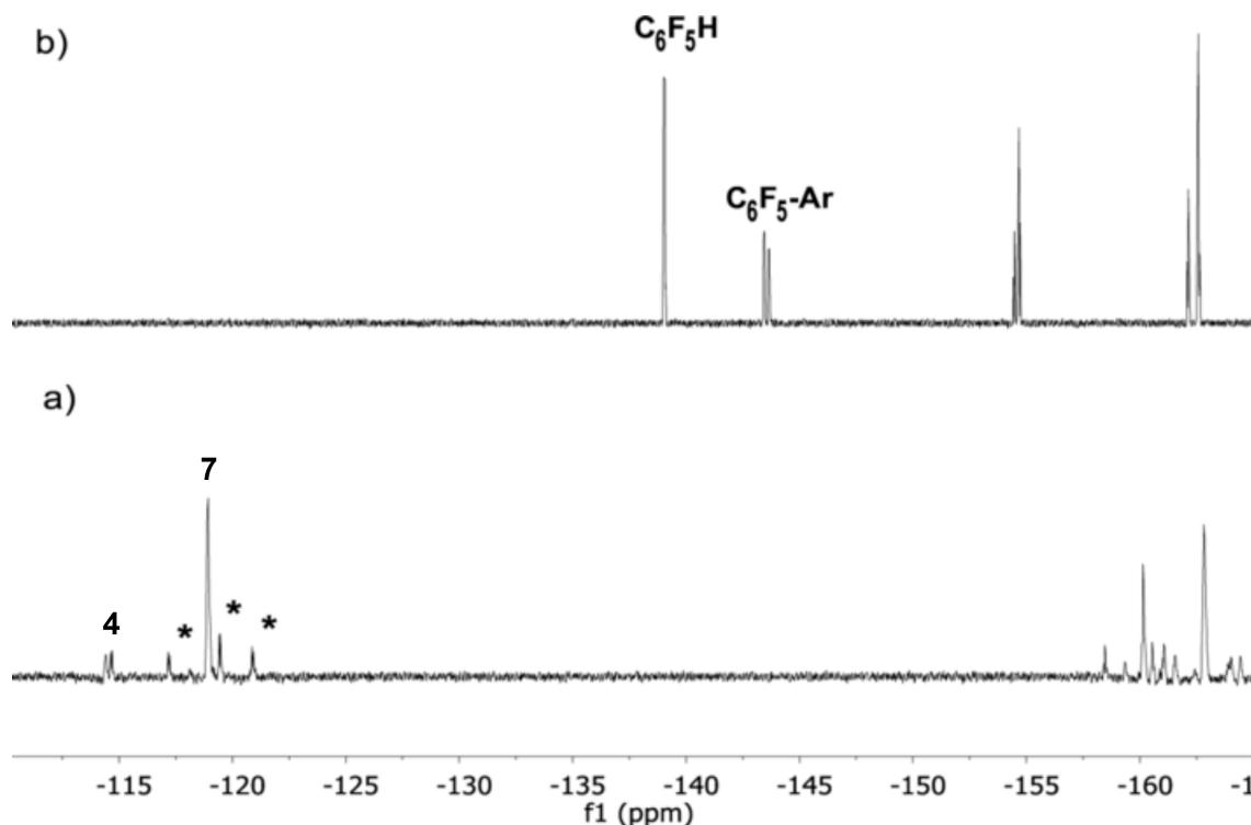
**Figure S3.**  $^{19}\text{F}$  NMR spectra in benzonitrile as solvent using a DMSO-d6 capillary. a) Complex 4 in benzonitrile. \* Unknown species. b) Mixture obtained after heating complex 4 for 1 h at 130 °C ( $\text{C}_6\text{F}_5\text{-Ar}$  is a mixture of two isomers). Only the  $^{19}\text{F}$  <sub>ortho</sub> region is labeled for clarity (Ar =  $\text{C}_6\text{H}_4\text{CN}$ ).
