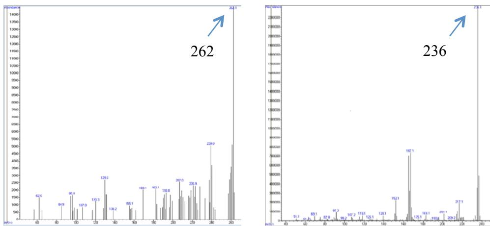
**Figure S11.** Mass spectra of the organic products obtained in the catalytic reaction shown in Eq. 3 (main text). Left:  $\text{C}_6\text{F}_5\text{-C}_6\text{D}_4\text{-}m\text{-CH}_3$ . Right: one of the isomers of Ar-Tol,  $p\text{-CF}_3\text{-C}_6\text{H}_4\text{-C}_6\text{H}_4\text{-}m\text{-CH}_3$
