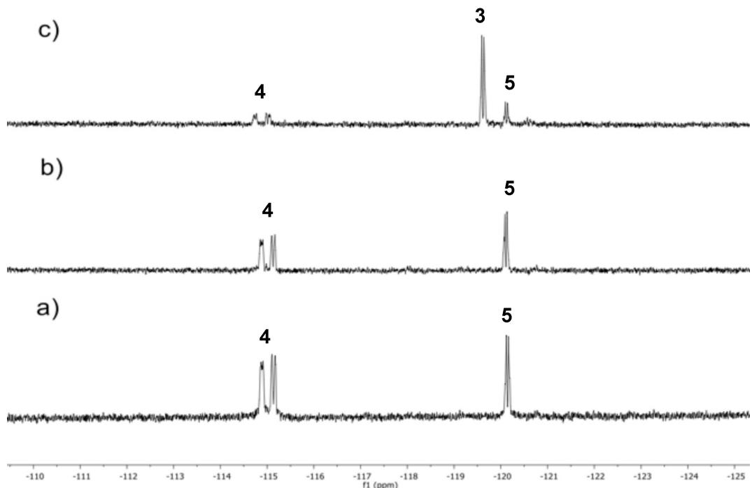
**Figure S6.**  $^{19}\text{F}$  NMR spectra (ortho region) in  $\text{CD}_2\text{Cl}_2$ . a) Complex **4** dissolved in  $\text{CD}_2\text{Cl}_2$ . b) Mixture obtained after adding 10  $\mu\text{L}$  of pinacolone to complex **4** solution in  $\text{CD}_2\text{Cl}_2$  (ratio Pd:pinacolone = 1:10). c) Mixture obtained after adding 0.5 mL of pinacolone to complex **4** in  $\text{CD}_2\text{Cl}_2$  (ratio Pd:pinacolone = 1:1000).
