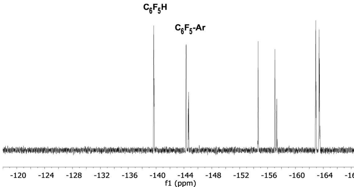
**Figure S4.**  $^{19}\text{F}$  NMR spectrum in toluene as solvent using a DMSO-d6 capillary after heating complex 4 for 1 h at 130 °C ( $\text{C}_6\text{F}_5\text{-Ar}$  is a mixture of two isomers). Only the  $^{19}\text{F}$  <sub>ortho</sub> region is labeled for clarity (Ar = Tolyl).
