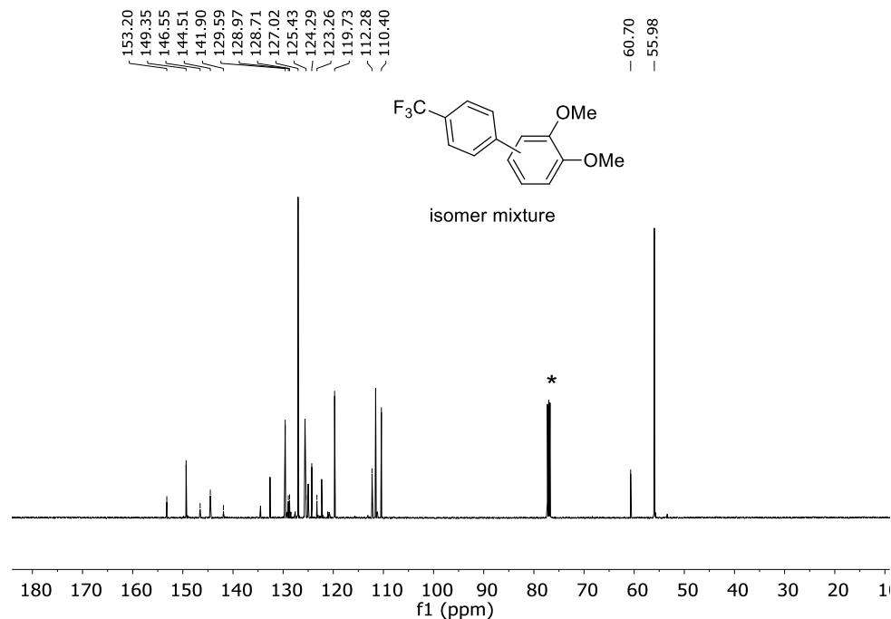
**Figure S28.**  $^{13}\text{C}\{\text{H}\}$  NMR (125.67 MHz,  $\text{CDCl}_3$ ) of an isomer mixture of 3,4-dimethoxy-4'-(trifluoromethyl)-1,1'-biphenyl and 2,3-dimethoxy-4'-(trifluoromethyl)-1,1'-biphenyl (3:1) at 298 K. \* Signal corresponding to the solvent (chloroform).
