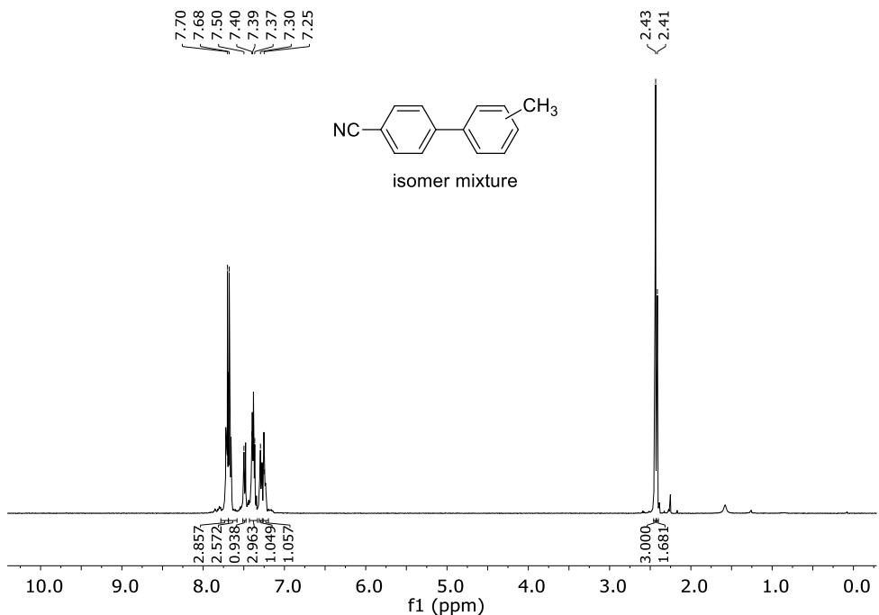
**Figure S15.**  $^1\text{H}$  NMR (499.73,  $\text{CDCl}_3$ ) of an isomer mixture of 3'-methyl-[1,1'-biphenyl]-4-carbonitrile and 4'-methyl-[1,1'-biphenyl]-4-carbonitrile (1.7:1) at 298 K.
