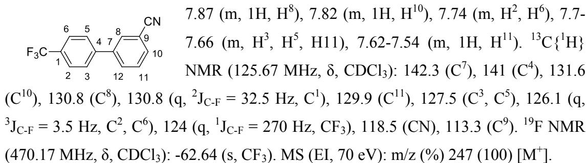
**4'-(Trifluoromethyl)-[1,1'-biphenyl]-4-carbonitrile:**<sup>13</sup> <sup>1</sup>H NMR (499.73 MHz, δ, CDCl<sub>3</sub>):
