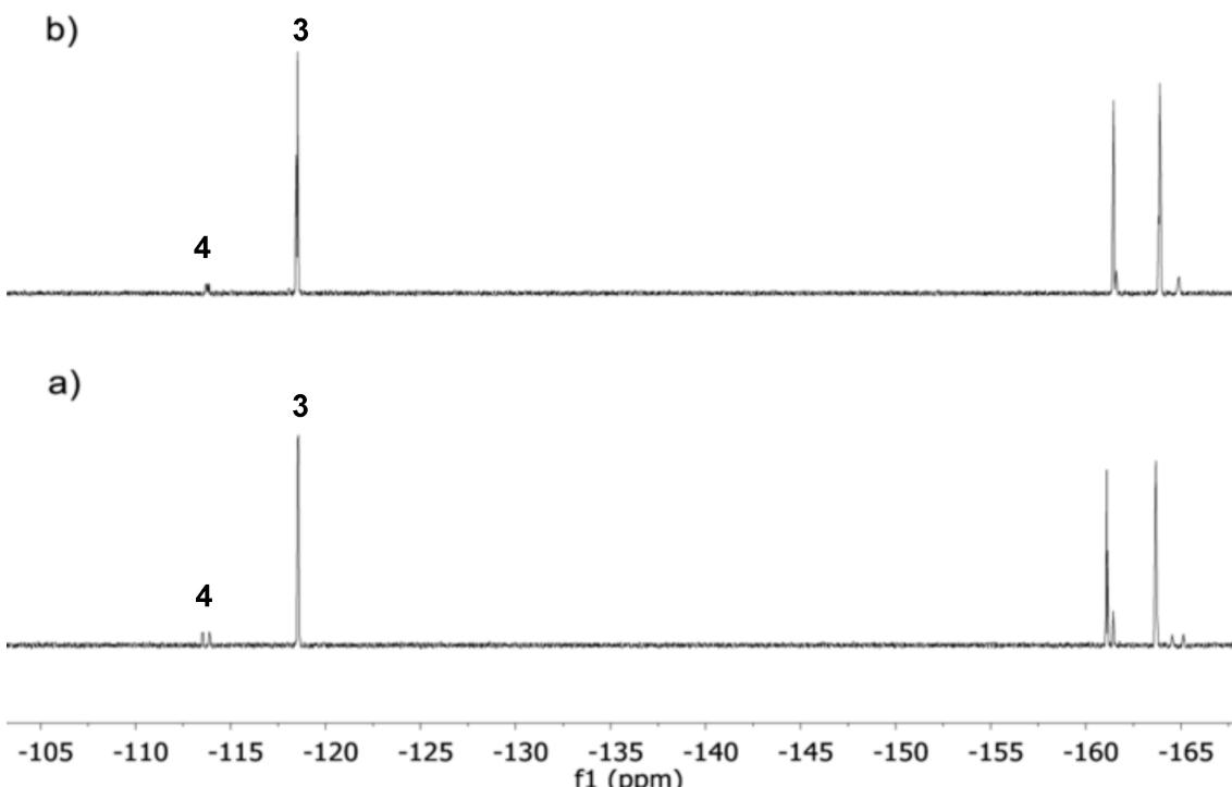
**Figure S5.** <sup>19</sup>F NMR spectra in the indicated solvent using a DMSO-d6 capillary as reference. a) complex **1** and Cs<sub>2</sub>CO<sub>3</sub> in a mixture of toluene and pinacolone (1:1) (**3:4** = 11:1 mol ratio). b) complex **1** and Cs<sub>2</sub>CO<sub>3</sub> in pinacolone (**3:4** = 20:1 mol ratio). Only the <sup>19</sup>F<sub>ortho</sub> region is labeled for clarity.
