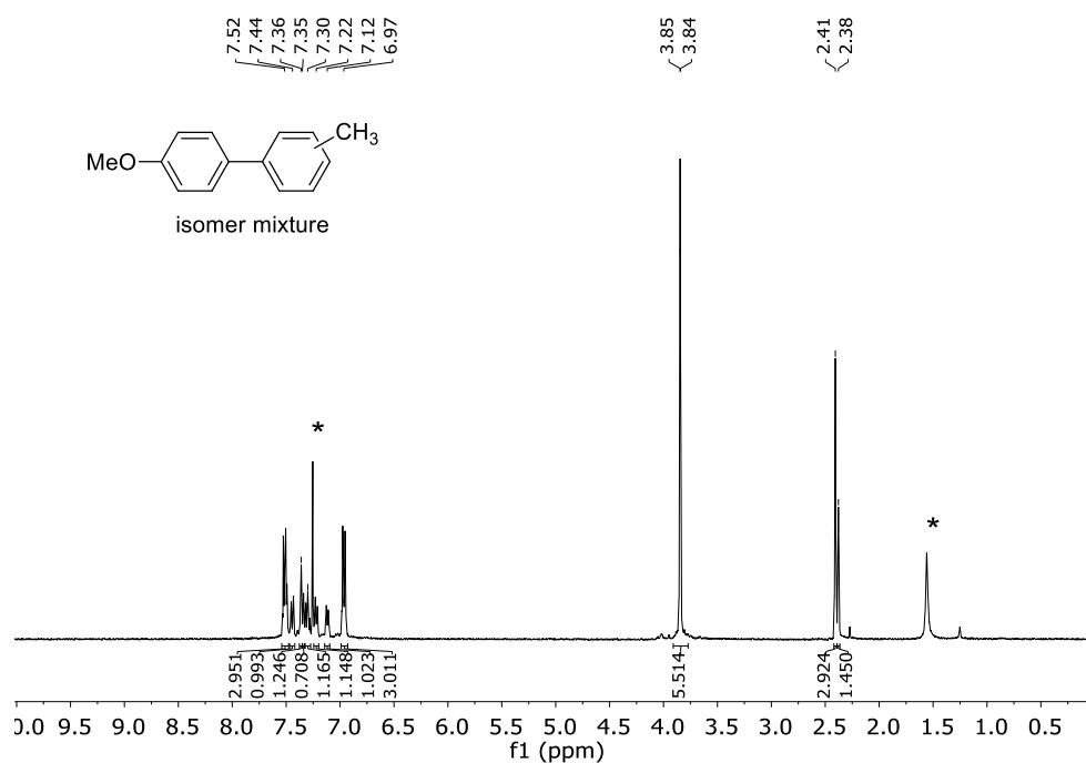
**Figure S13.**  $^1\text{H}$  NMR (499.73,  $\text{CDCl}_3$ ) of an isomer mixture of 4'-methoxy-3-methyl-1,1'-biphenyl and 4'-methoxy-4-methyl-1,1'-biphenyl (2:1) at 298 K. \* Signal corresponding to the solvent (chloroform and  $\text{H}_2\text{O}$ ).
