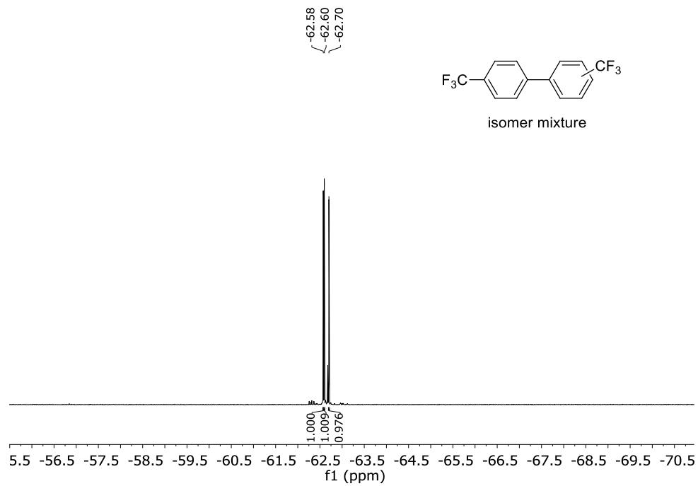
**Figure S21.**  $^{19}\text{F}$  NMR (470.17 MHz,  $\text{CDCl}_3$ ) of an isomer mixture of 3,4'-bis(trifluoromethyl)-1,1'-biphenyl, and 4,4'-bis(trifluoromethyl)-1,1'-biphenyl (2:1) at 298 K.
