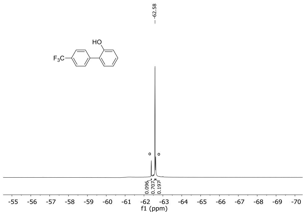
**Figure S36.** <sup>19</sup>F NMR (470.17 MHz, CDCl<sub>3</sub>) of 4'-(trifluoromethyl)-[1,1'-biphenyl]-2-ol (80 % pure) at 298 K. ° Signals corresponding to the doble arylation of phenol products (m/z = 382).
