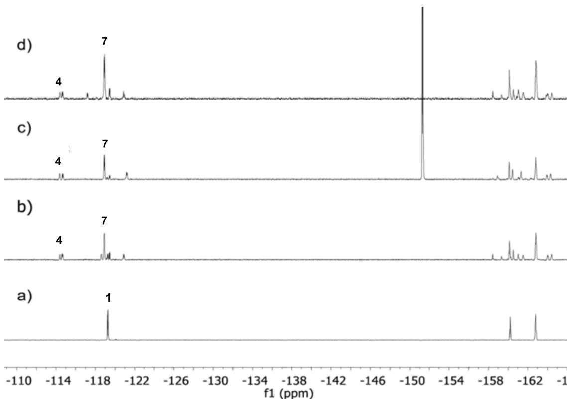
**Figure S10.**  $^{19}\text{F}$  NMR spectra in benzonitrile as solvent using a DMSO-d6 capillary. a) Complex **1** in benzonitrile. b) Complex **1** in benzonitrile after adding  $\text{Cs}_2\text{CO}_3$ . c) mixture b with  $\text{AgBF}_4$ . d) Complex **8** isolated independently and dissolved in benzonitrile. Only the  $^{19}\text{F}_{\text{ortho}}$  region is labeled for clarity.
