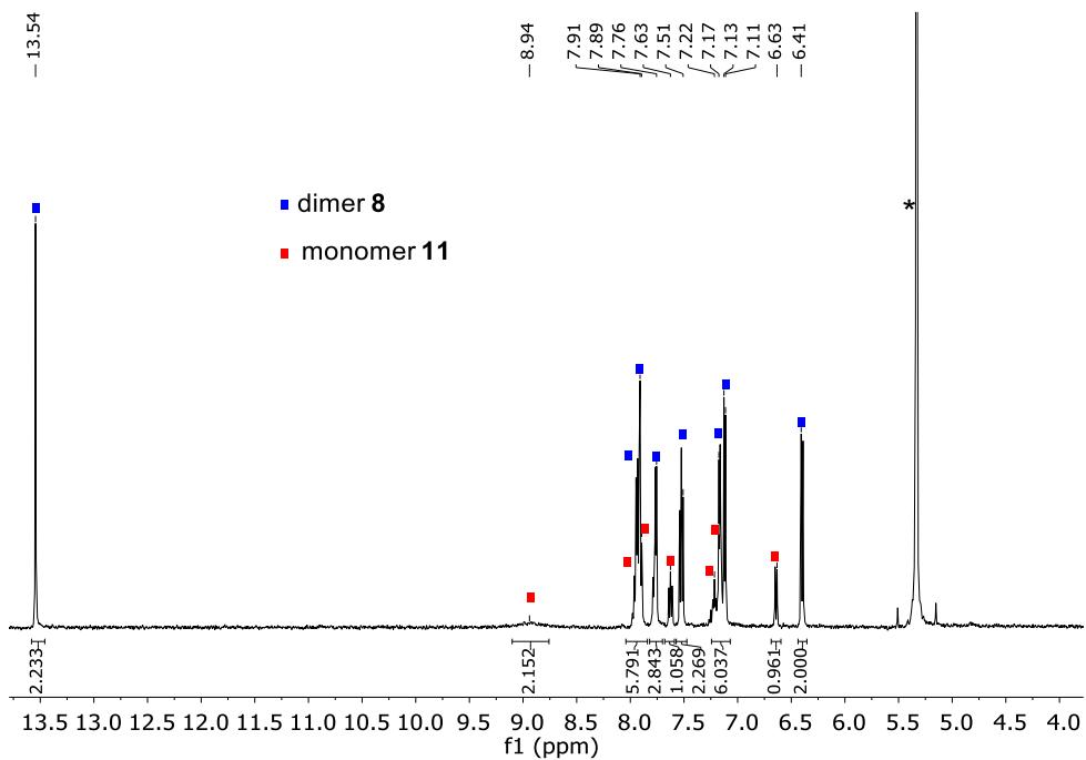
**Figure S38.**  $^1\text{H}$  NMR (499.73 MHz,  $\text{CD}_2\text{Cl}_2$ ) of the mixture formed after complex  $[\text{Pd}_2(\text{bipy}-6-\text{O})_2(\text{C}_6\text{F}_5)_2\mu\text{OH}_2]$  (**8**) is dissolved in  $\text{CD}_2\text{Cl}_2$ . The red species corresponds to the monomer species  $[\text{Pd}(\text{bipy}-6-\text{O})(\text{C}_6\text{F}_5)(\text{H}_2\text{O})]$ . Ratio dimer **8:11** = 1:1. \* Signal corresponding to the solvent.
