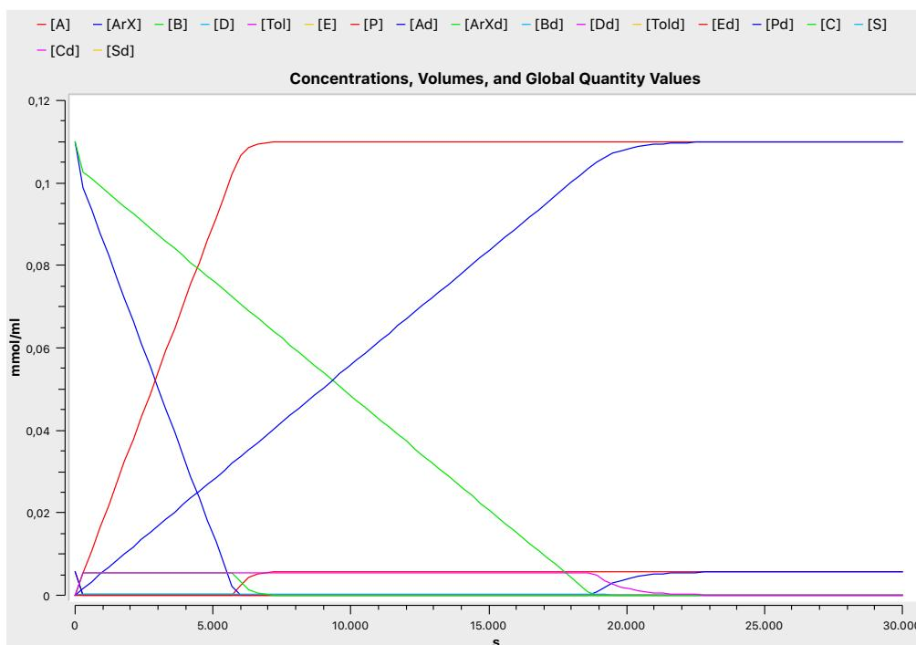
**Figure S44.** Kinetic simulation of the KIE in separate flasks. It shows the evolution of concentration ( $M$ ) over time (s) for the reaction in Eq. S3 in toluene/pinacolone (product P, red) or toluene-d8/pinacolone (product Pd, blue). The concentration of toluene and pinacolone remain constant and have been omitted for clarity.
