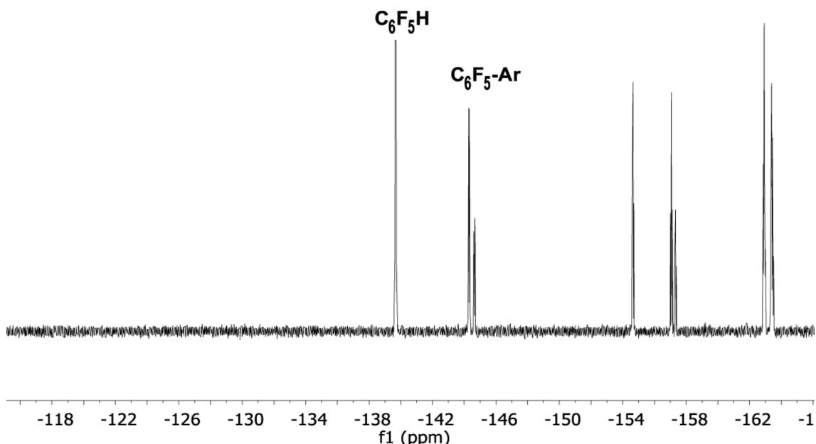
**Figure S2.**  $^{19}\text{F}$  NMR spectrum in toluene as solvent using a DMSO-d6 capillary after heating complex **2** for 1 h at 130 °C ( $\text{C}_6\text{F}_5\text{-Ar}$  is a mixture of two isomers). Only the  $^{19}\text{F}_{\text{ortho}}$  region is labeled for clarity (Ar = Tolyl).
