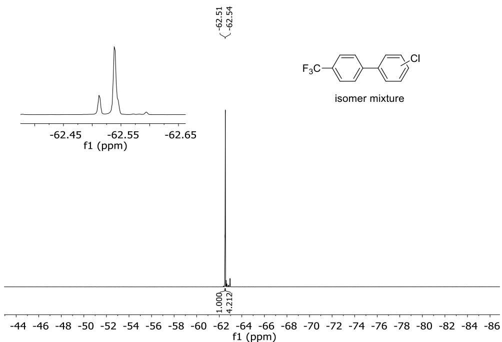
**Figure S33.**  $^{19}\text{F}$  NMR (470.17 MHz,  $\text{CDCl}_3$ ) of an isomer mixture of 3-chloro-4'-(trifluoromethyl)-1,1'-biphenyl and 4-chloro-4'-(trifluoromethyl)-1,1'-biphenyl (4:1) at 298 K.
