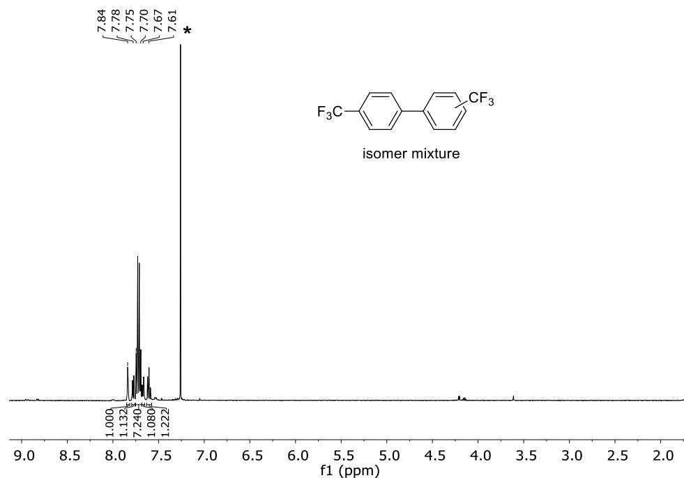
**Figure S20.**  $^1\text{H}$  NMR (499.73,  $\text{CDCl}_3$ ) of an isomer mixture of 3,4'-bis(trifluoromethyl)-1,1'-biphenyl, and 4,4'-bis(trifluoromethyl)-1,1'-biphenyl (2:1) at 298 K. \* Signal corresponding to the solvent (chloroform).
