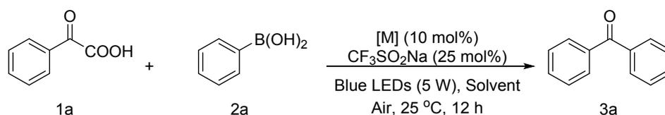
A mixture of phenylglyoxylic acid (**1a**), phenylboronic acid (**2a**), sodium trifluoromethanesulfonate, transition-metal-catalyst and solvent was added into a quartz tube which was placed in a photochemical reactor. The reaction mixture was stirred at the designed temperature under air. After concentrated under reduced pressure, the residue was purified by
