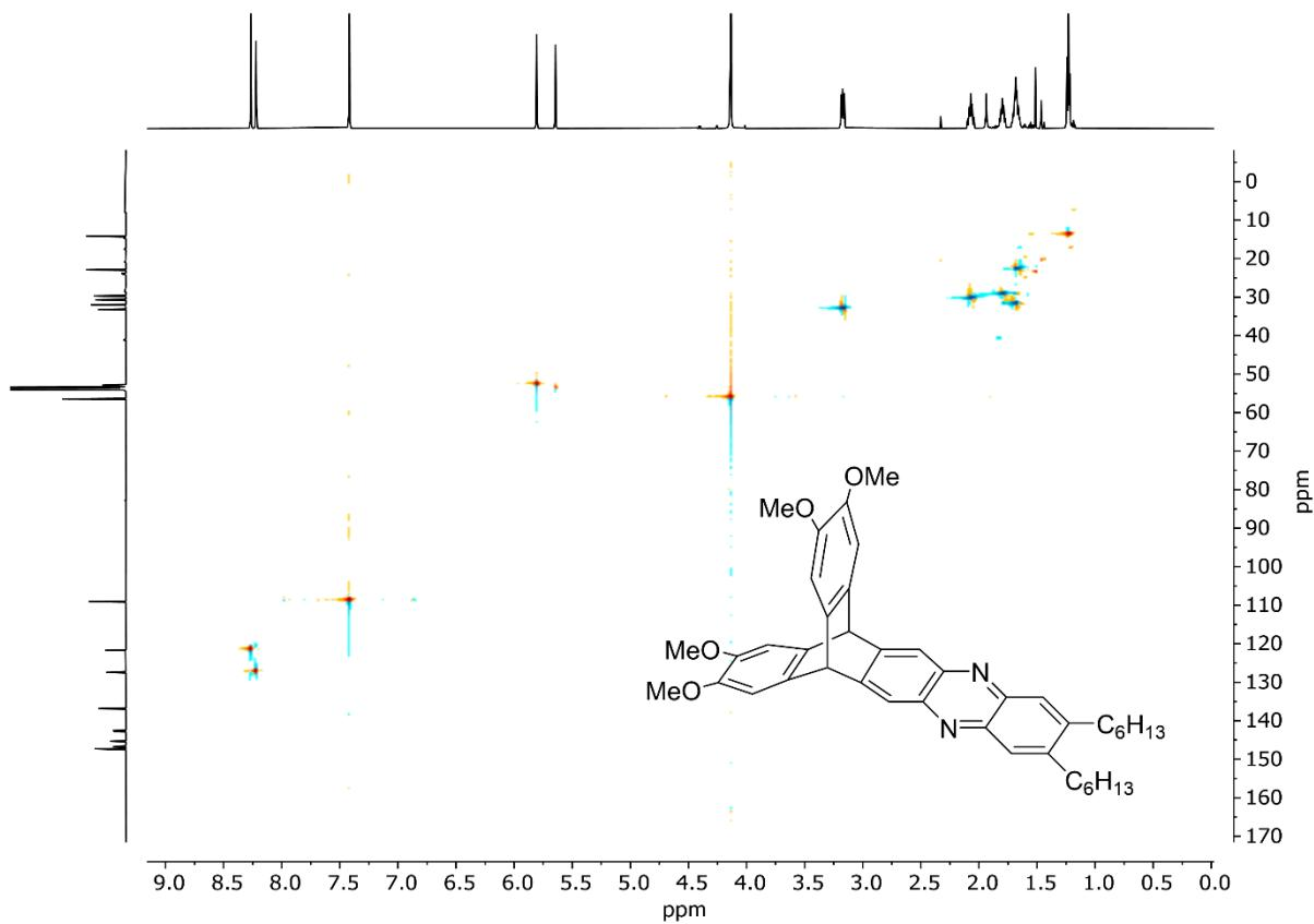
**Figure S18:**  $^1\text{H}, ^{13}\text{C}$ -HSQC Spectrum ( $\text{CD}_2\text{Cl}_2$ , 600MHz, 151 MHz) of **4**.
