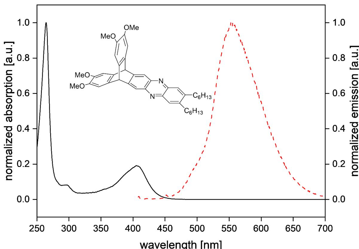
**Figure S55:** UV/vis (black solid line) and fluorescence (red dotted line) spectrum of **4** in dichlormethane. The excitation energy for the fluorescence is 406 nm.
