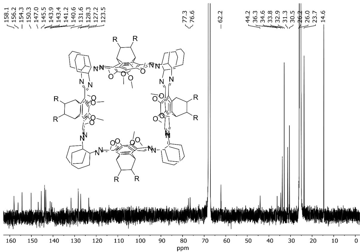
**Figure S15:**  $^{13}\text{C}$  NMR Spectrum ( $\text{THF-d}_8$ , 151 MHz) of **10** (not pure).
