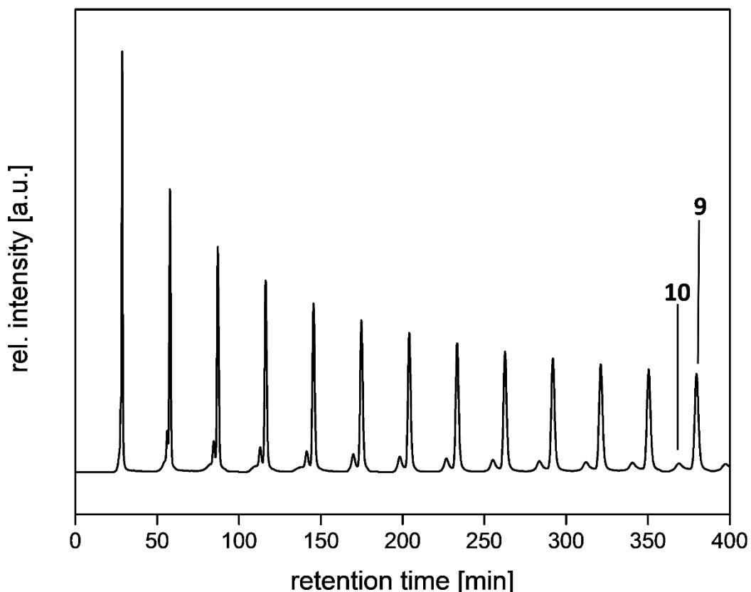
**Figure S65:** Chromatogram of the crude mixture of **9** and **10** (SDV column, THF, 5 mL/min,  $R_t = 28.65$  min, 254 nm).
