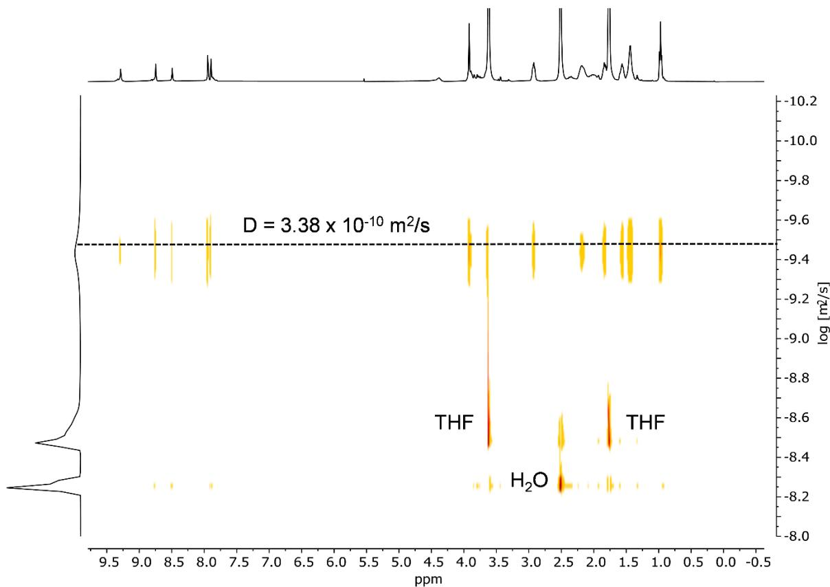
**Figure S41:**  $^1\text{H}$ -DOSY Spectrum (THF-d<sub>8</sub>, 400MHz) of **10**.
