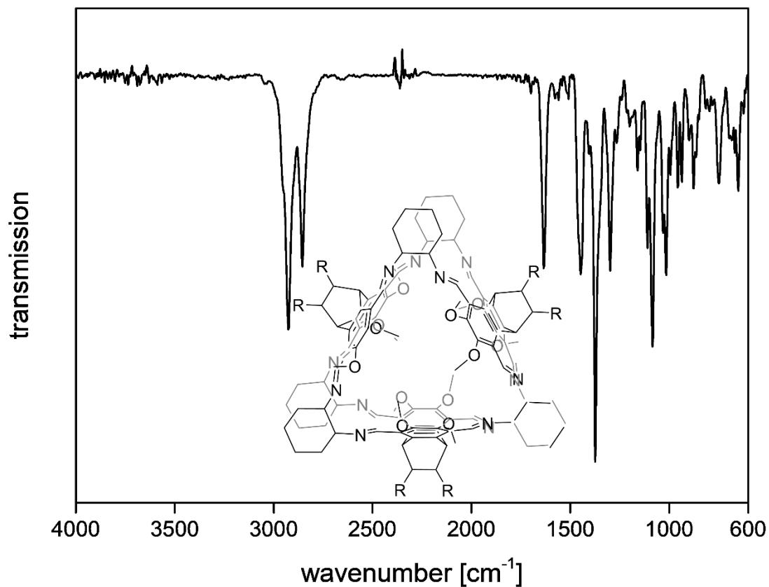
Figure S54: IR Spectrum (ATR, ZnSe) of 9.
