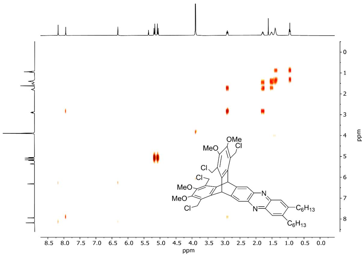
**Figure S20:**  $^1\text{H}$ , $^1\text{H}$ -COSY Spectrum ( $\text{CD}_2\text{Cl}_2$ , 400MHz) of **5**.
