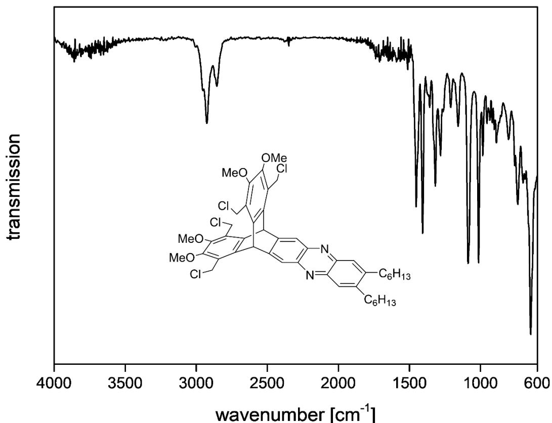
**Figure S51:** IR Spectrum (ATR, ZnSe) of 5.
