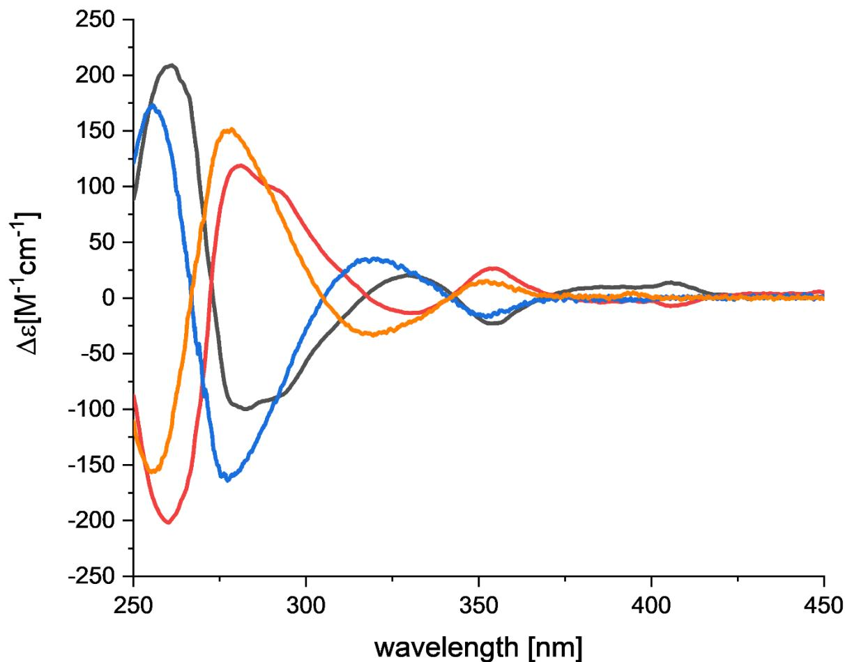
**Figure S60:** CD spectra of (R,R)-**9** (black line,  $c = 6.09 \cdot 10^{-6}$  mol/L), (S,S)-**9** (red line,  $c = 5.98 \cdot 10^{-6}$  mol/L), (R,R)-**10** (blue line,  $c = 6.00 \cdot 10^{-6}$  mol/L), (S,S)-**10** (orange line,  $c = 6.00 \cdot 10^{-6}$  mol/L), in DCM at 20 °C.
