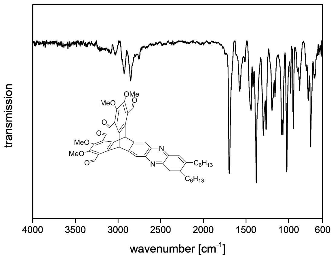
Figure S53: IR Spectrum (ATR, ZnSe) of 7.
