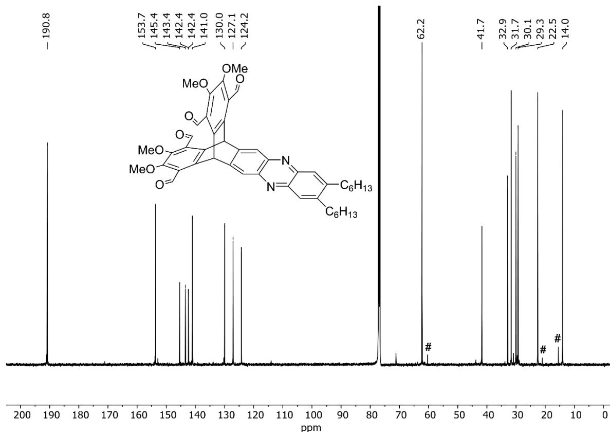
**Figure S13:**  $^{13}\text{C}$  NMR Spectrum ( $\text{CDCl}_3$ , 151 MHz) of **7**. Solvent residues: #: EA.
