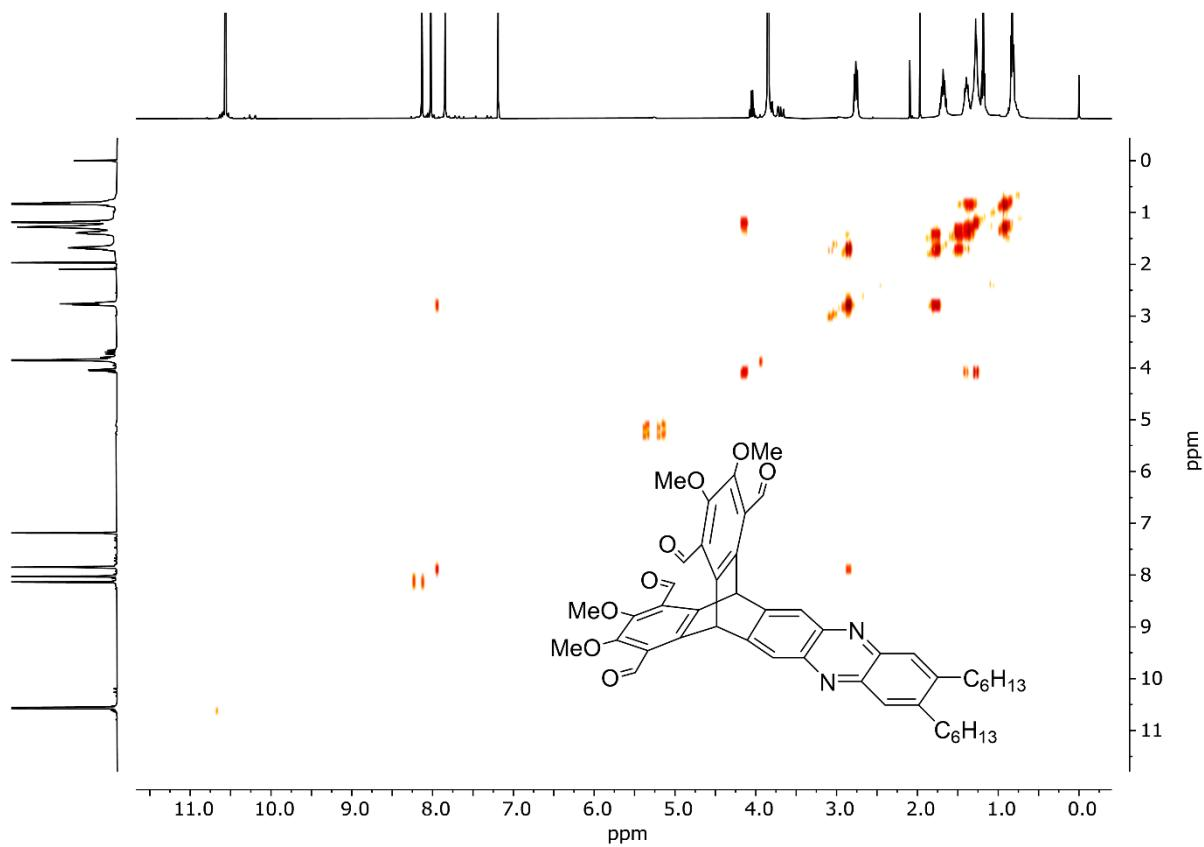
**Figure S28:**  $^1\text{H}$ , $^1\text{H}$ -COSY Spectrum ( $\text{CDCl}_3$ , 600MHz) of 7.
