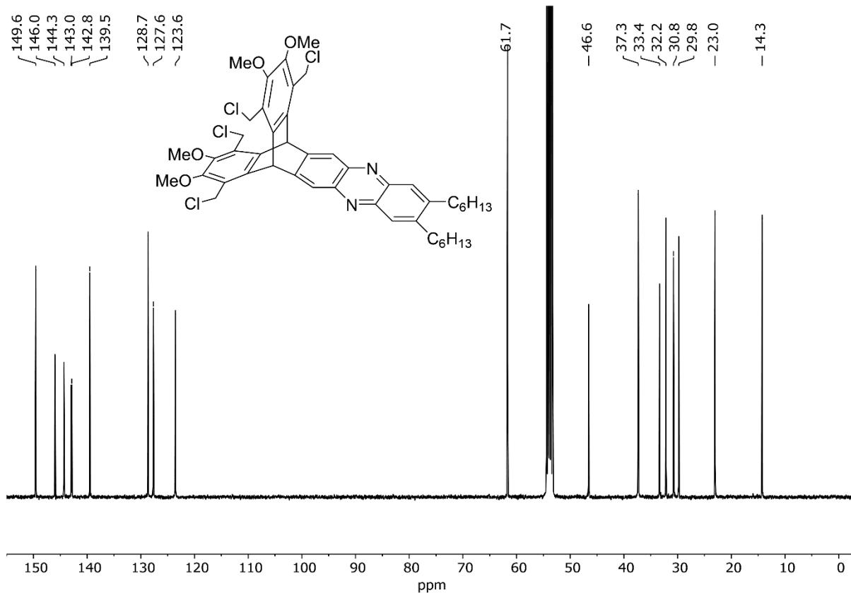
**Figure S11:**  $^{13}\text{C}$  NMR Spectrum ( $\text{CD}_2\text{Cl}_2$ , 101 MHz) of **5**.
