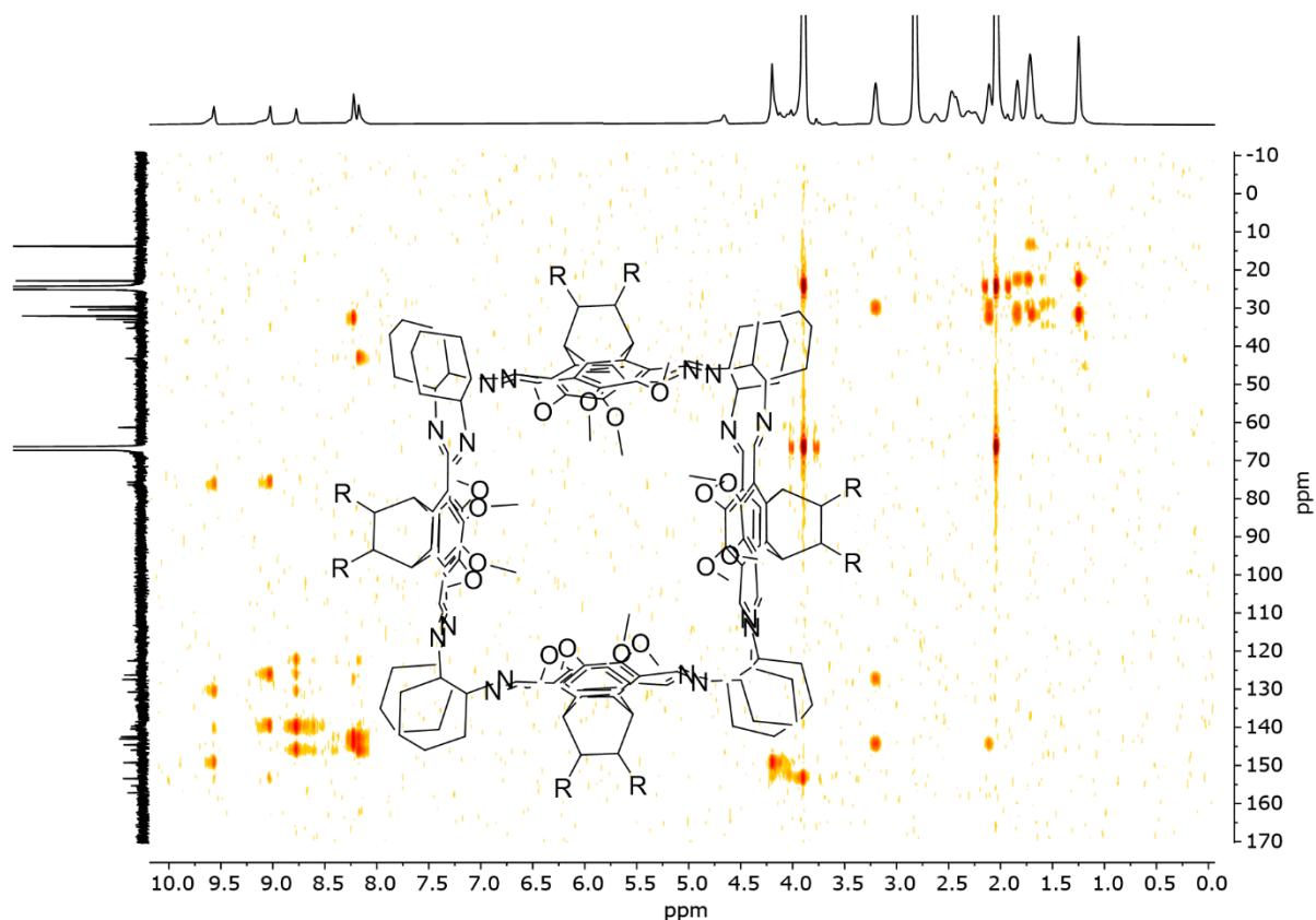
**Figure S39:**  $^1\text{H}, ^{13}\text{C}$ -HMBC Spectrum (THF-d<sub>8</sub>, 600MHz, 151MHz) of **10**.
