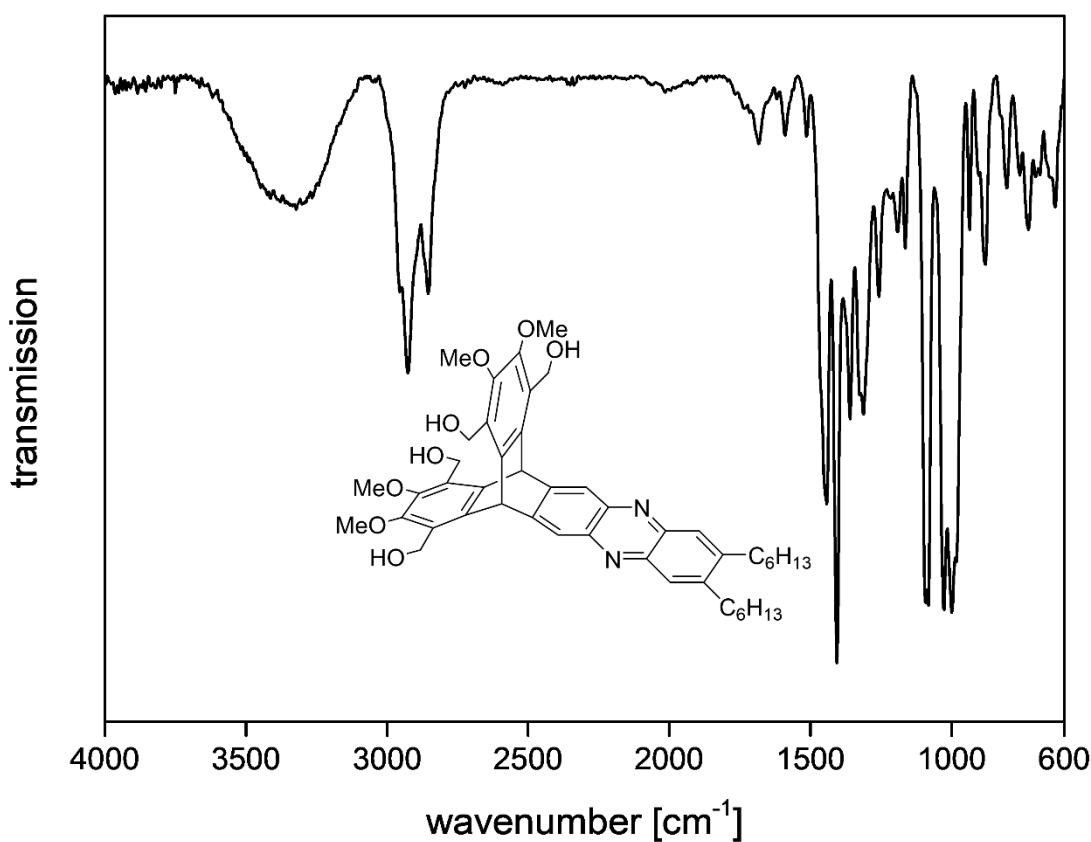
**Figure S52:** IR Spectrum (ATR, ZnSe) of 6.
