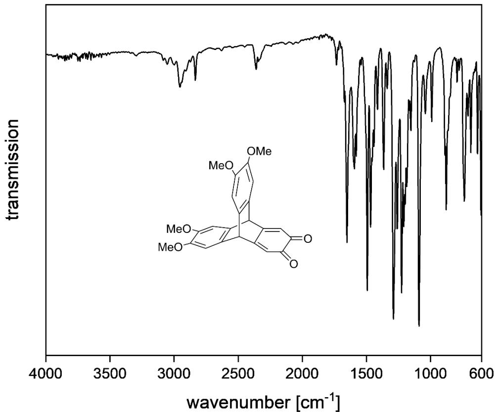
**Figure S49:** IR Spectrum (ATR, ZnSe) of 2.
