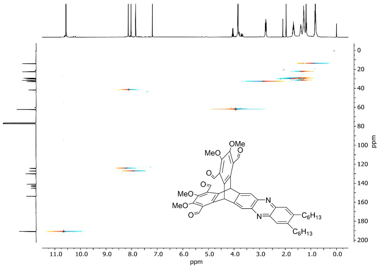
**Figure S30:**  $^1\text{H}, ^{13}\text{C}$ -HSQC Spectrum ( $\text{CDCl}_3$ , 400MHz, 101MHz) of 7.
