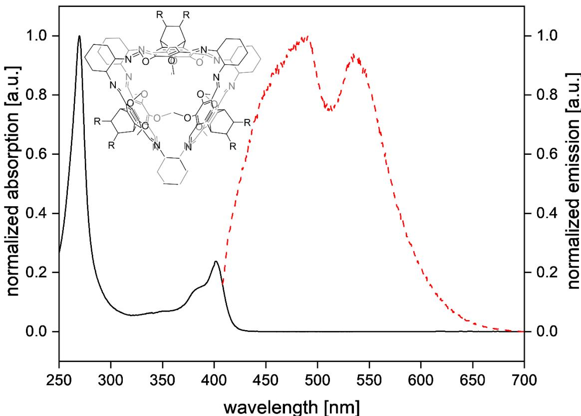
**Figure S59:** UV-vis (black solid line) and fluorescence (red dotted line) spectrum of **9** in dichloromethane. The excitation energy for the fluorescence is 402 nm.
