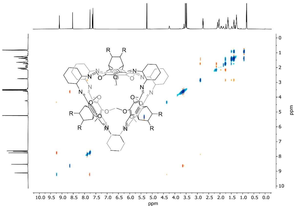
**Figure S33:**  $^1\text{H}, ^1\text{H}$ -ROESY Spectrum ( $\text{CD}_2\text{Cl}_2$ , 700MHz) of **9**.
