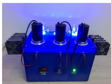
Figure S1. The Photo Reaction Setup and Blue LED lamps
