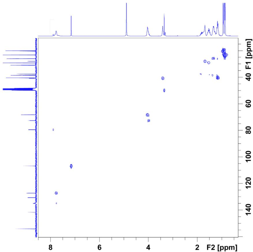
$^1\text{H},^{13}\text{C}$ -HMOC spectrum (MeOD- $d_4$ , 25  $^\circ\text{C}$ ) of compound 11.
