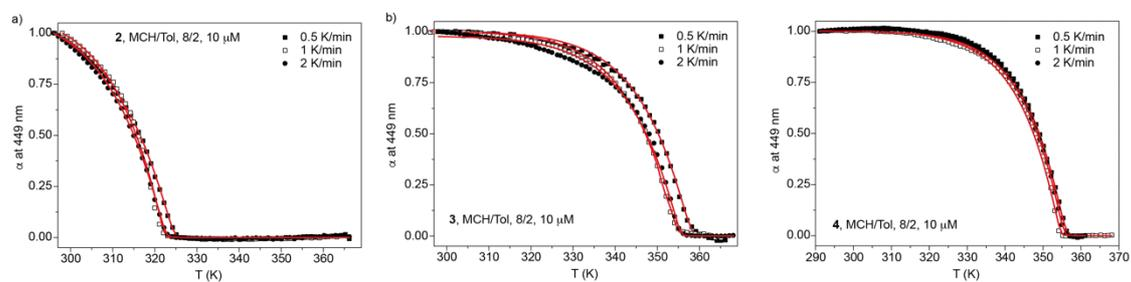
**Figure S8.** Plot of the variation of the degree of aggregation ( $\alpha$ ) versus temperature for compounds **2** (a), **3** (b) and **4** (c) at different cooling rates (0.5, 1 or 2  $^{\circ}\text{C}/\text{min}$ ). The red lines depict the fitting to the one-component EQ model. Experimental conditions: MCH/Tol 8/2 as solvent,  $c_T = 10 \mu\text{M}$ .
