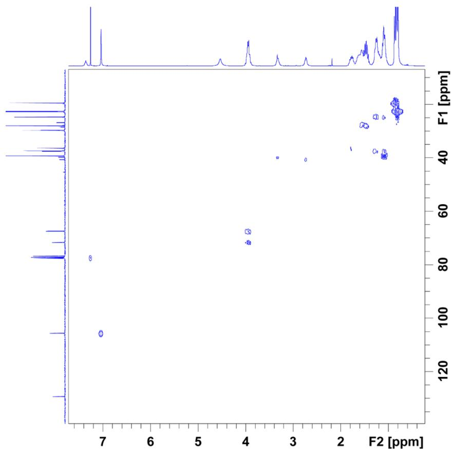
$^1\text{H},^{13}\text{C}$ -HMOC spectrum ( $\text{CDCl}_3$ , 25  $^\circ\text{C}$ ) of compound 8.
