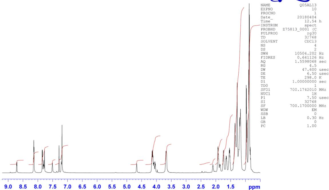
$^1\text{H}$  NMR ( $\text{CDCl}_3$ , 700 MHz, 25  $^\circ\text{C}$ ) of compound 2.
