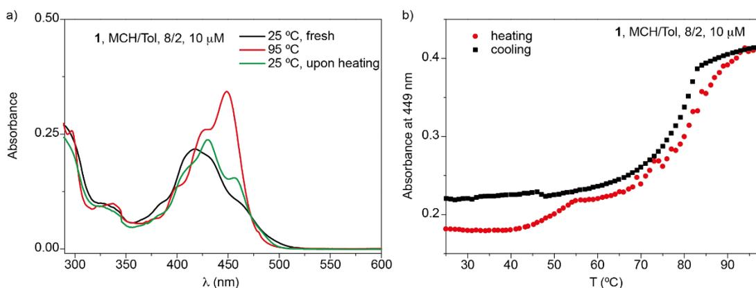
**Figure S3.** UV-Vis spectra (a) and variation of the absorbance at  $\lambda = 449$  nm (b) of a diluted solution of **1** (MCH/Tol (8/2);  $c_T = 10 \mu\text{M}$ ; cooling and heating rate =  $1 \text{ }^\circ\text{C}/\text{min}$ ).
