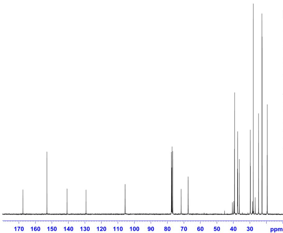
$^{13}\text{C}$  NMR ( $\text{CDCl}_3$ , 75 MHz, 25  $^\circ\text{C}$ ) of compound 8.
