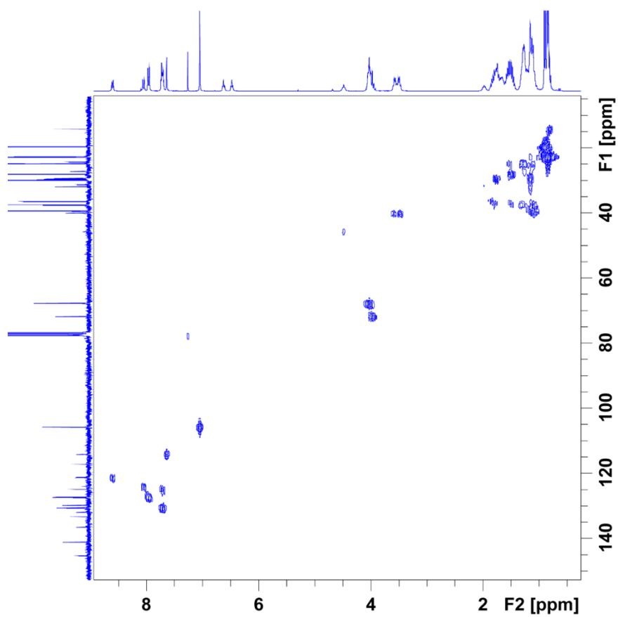
$^1\text{H},^{13}\text{C}$ -HMQC spectrum ( $\text{CDCl}_3$ , 25  $^\circ\text{C}$ ) of compound 4.
