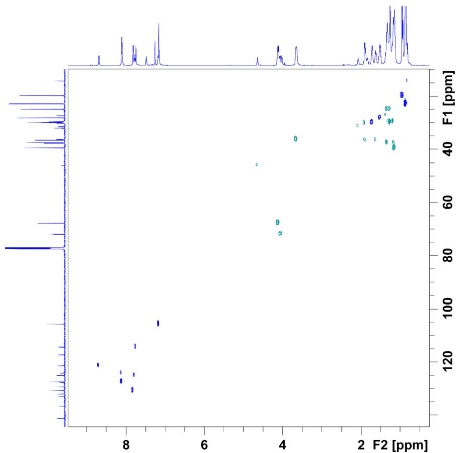
$^1\text{H},^{13}\text{C}$ -HMQC spectrum ( $\text{CDCl}_3$ , 25  $^\circ\text{C}$ ) of compound 2.
