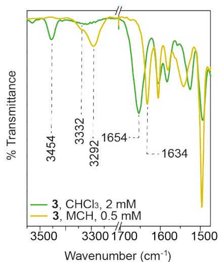
**Figure S2.** Partial FTIR spectra of **3** in solution showing the region in which the stretching N-H and Amide I bands are observed.
