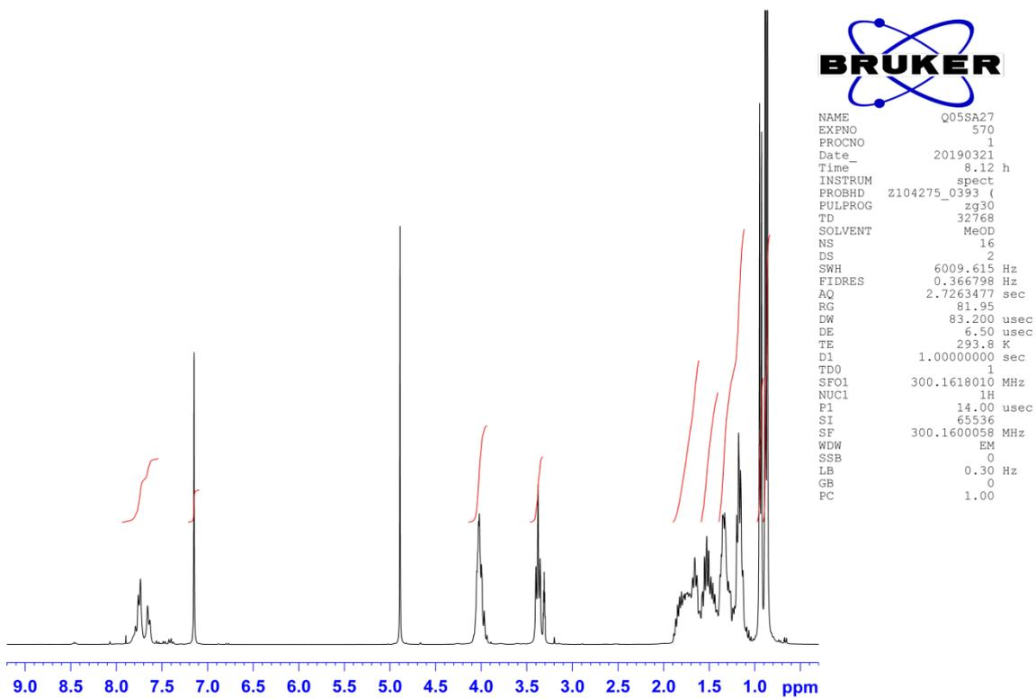
$^1\text{H}$  NMR (MeOD- $d_4$ , 300 MHz, 25  $^\circ\text{C}$ ) of compound 12.
