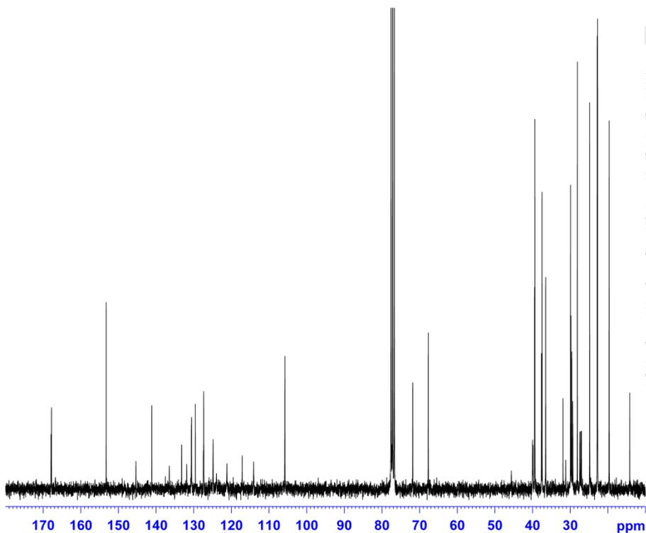
$^{13}\text{C}$  NMR ( $\text{CDCl}_3$ , 75 MHz, 25  $^\circ\text{C}$ ) of compound 3.
