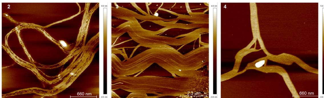
**Figure S7.** AFM images of the fibrillar bundles formed by the supramolecular polymers of compounds **2-4**. Experimental conditions: MCH/Tol 8/2 as solvent,  $c_T = 10 \mu\text{M}$ , mica as surface.
