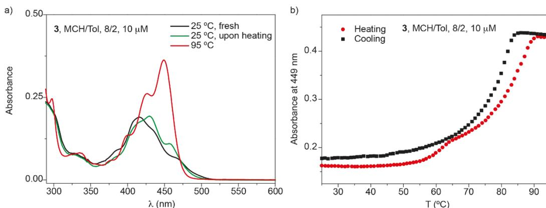
**Figure S4.** (a) UV-Vis spectra of **3**; (b) Variation of the absorbance at  $\lambda = 449$  nm of a diluted solution of **3** (experimental conditions: MCH/Tol (8/2);  $c_T = 10 \mu\text{M}$ ; cooling and heating rate =  $1 \text{ }^\circ\text{C}/\text{min}$ ).
