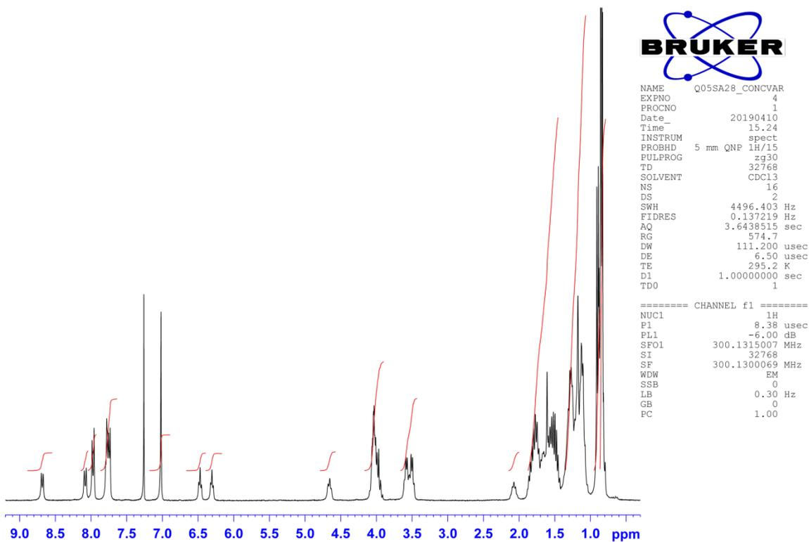
$^1\text{H}$  NMR ( $\text{CDCl}_3$ , 300 MHz, 25  $^\circ\text{C}$ ) of compound 4.
