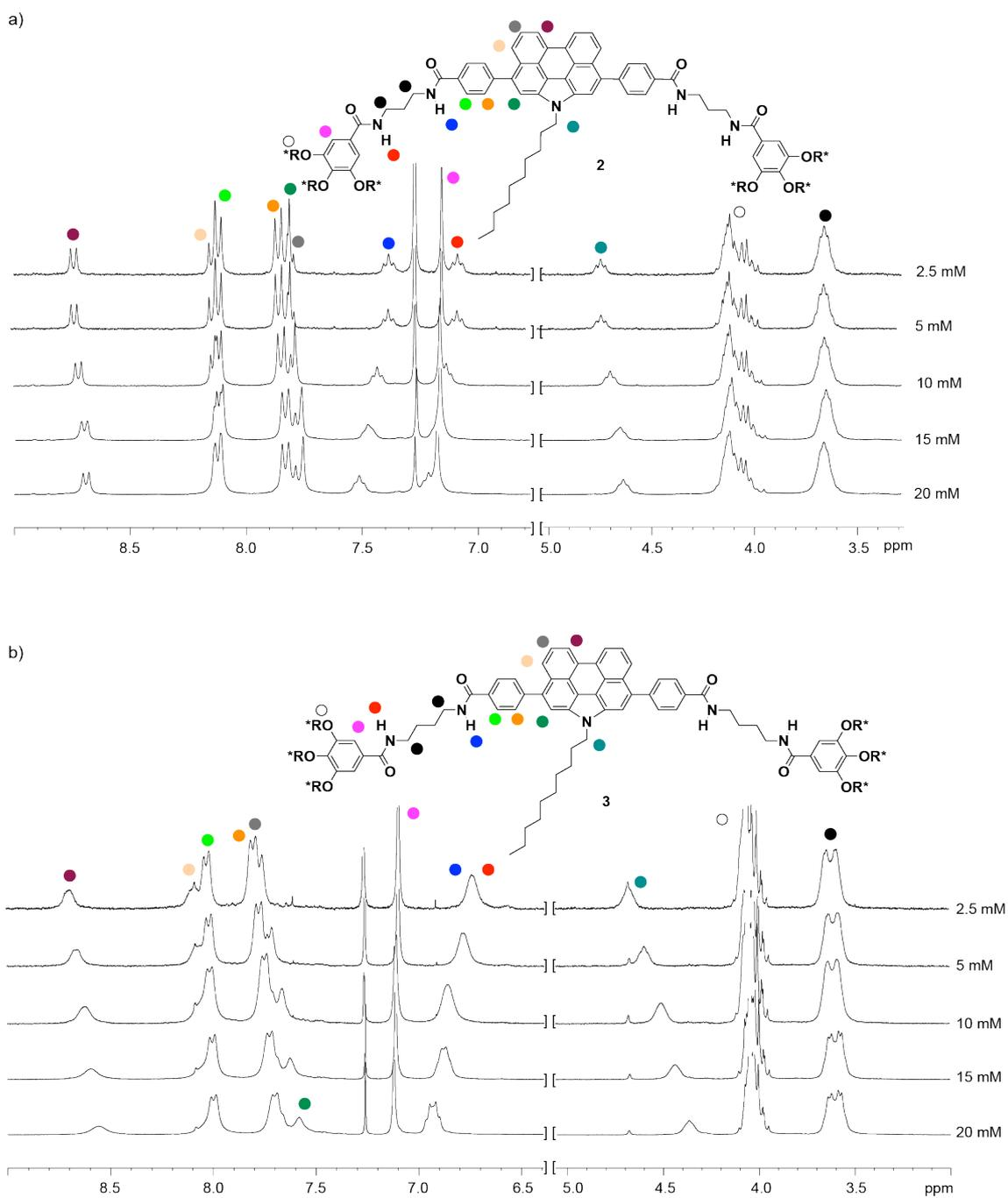
**Figure S1.** Partial  $^1\text{H}$  NMR spectra of **2** (a) and **3** (b) in  $\text{CDCl}_3$  at different concentrations (300 MHz, 25  $^\circ\text{C}$ ).
