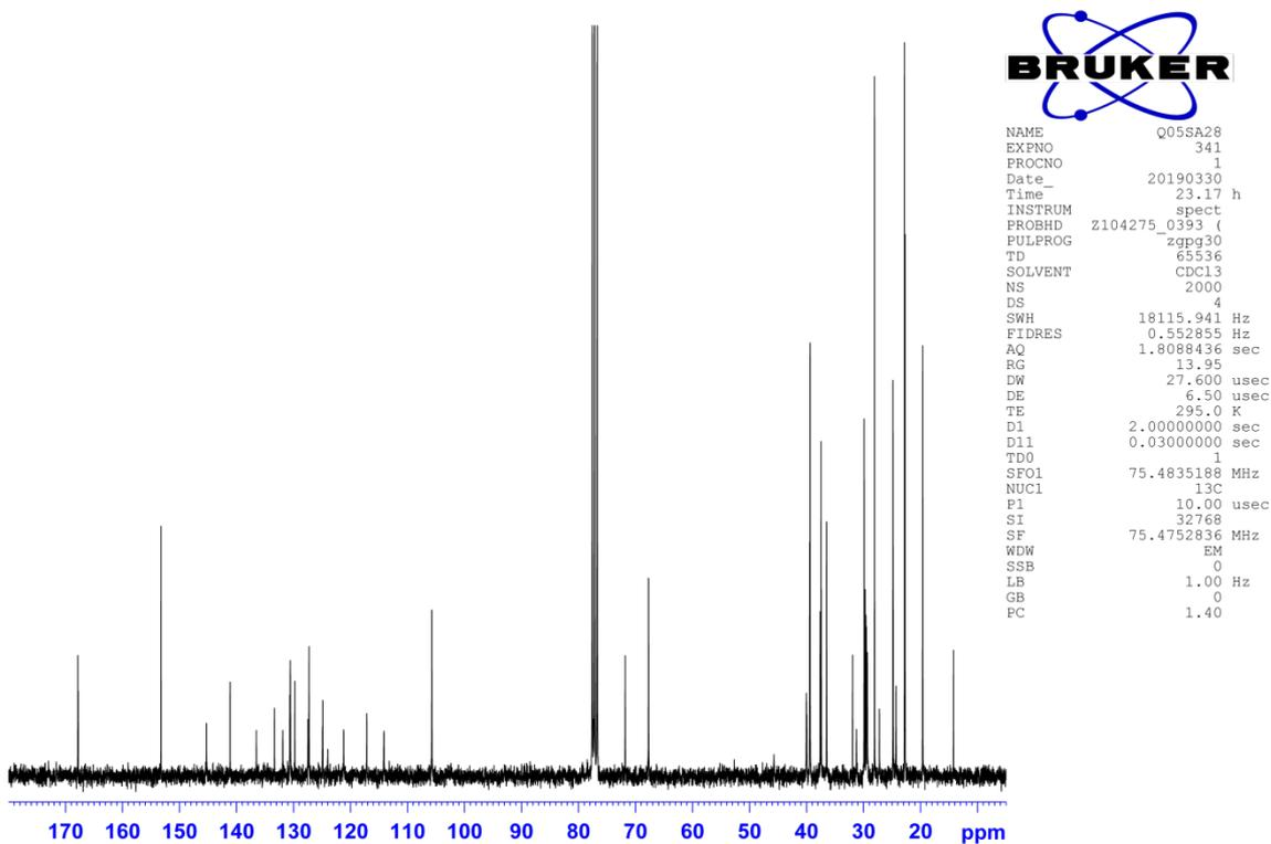
$^{13}\text{C}$  NMR ( $\text{CDCl}_3$ , 75 MHz, 25  $^\circ\text{C}$ ) of compound 4.
