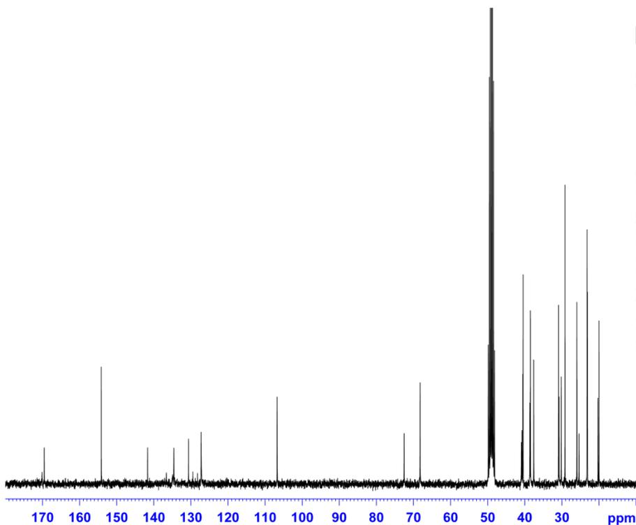
$^{13}\text{C}$  NMR (MeOD- $d_4$ , 75 MHz, 25  $^{\circ}\text{C}$ ) of compound **12**.
