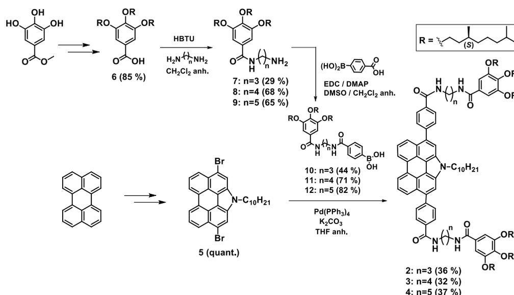
**Scheme S1.** Synthesis of chiral *N*-annulated perylenetetracarboxamides 2-4.
