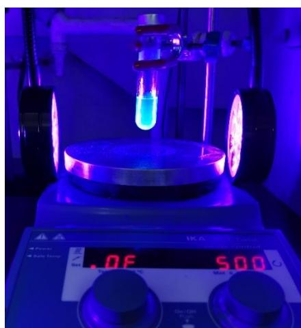
**Supplementary Figure 1.** Experimental setup for photocatalytic activation of alkyl chlorides.
