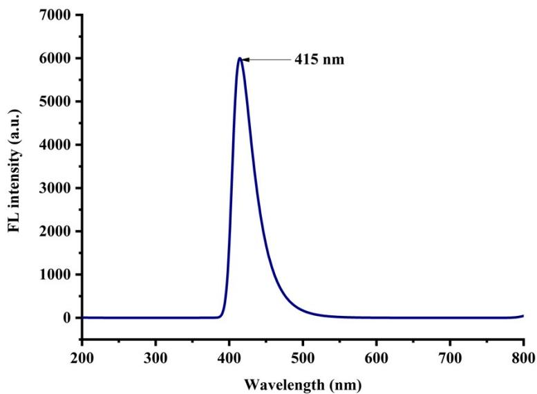
**Supplementary Figure 2.** Emission spectra of the 415 nm LED lamp.
