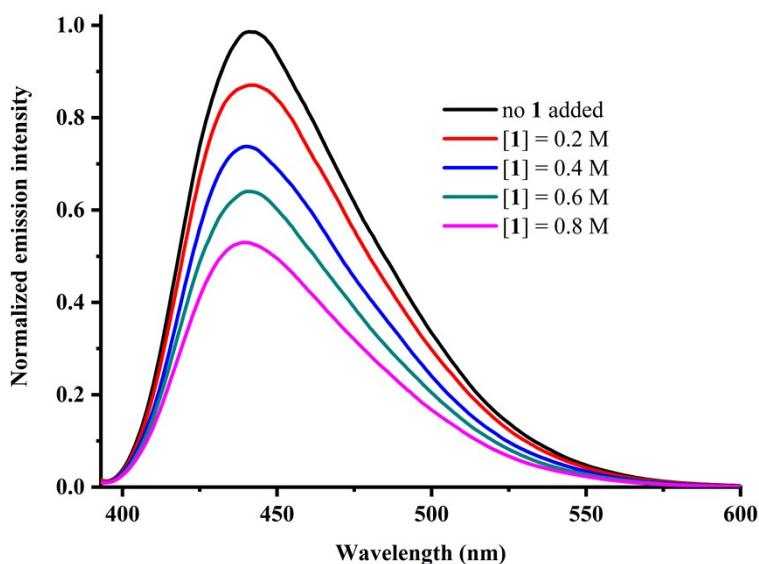
**Supplementary Figure 7.** Quenching of the phenolate anion of **DBPP1** emission ( $5 \times 10^{-5}$  M in DMF) in the presence of increasing amounts of **1**.
