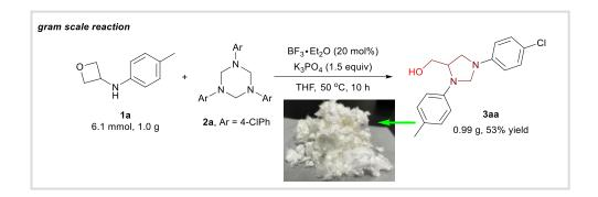
To a dried flask was added **1a** (1.0 g, 6.13 mmol), **2a** (2.05 g, 4.9 mmol), and  $K_3PO_4$  (1.89 g, 9.2 mmol), THF (61 mL). Then, BF<sub>3</sub>·Et<sub>2</sub>O (20 mol%) was added to the mixture. The reaction mixture was stirred at 50 °C for 6 h. The crude product was purified by chromatography on silica gel (petroleum ether/ethyl acetate = 50:1 to 10:1) directly to give the desired product **3aa** (0.99 g) in 53% isolated yield as a white solid.
