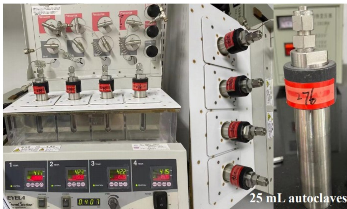
Figure S1. 25-mL autoclaves (Tokyo Rikakikai Co., LTD (PPM-5512))
