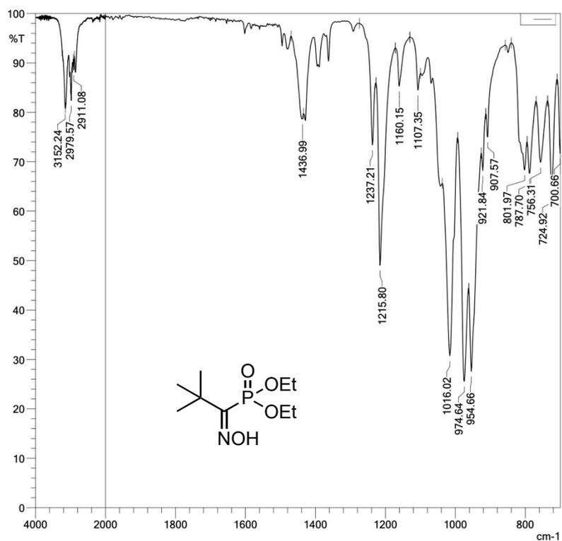
**Figure S125.** Infrared spectrum of diethyl (1-(hydroxyimino)-2,2-dimethylpropyl)phosphonate (neat) (**11b**).
