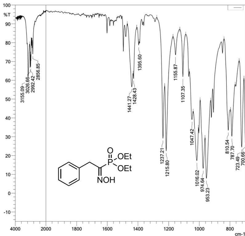
**Figure S124.** Infrared spectrum of diethyl (1-(hydroxyimino)-2-phenylethyl)phosphonate (neat) (**2b**).
