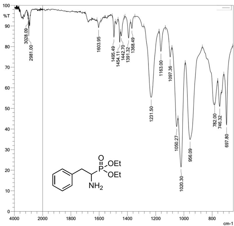
**Figure S128.** Infrared spectrum of diethyl (1-amino-2-phenylethyl)phosphonate (neat) (**am-2b**).
