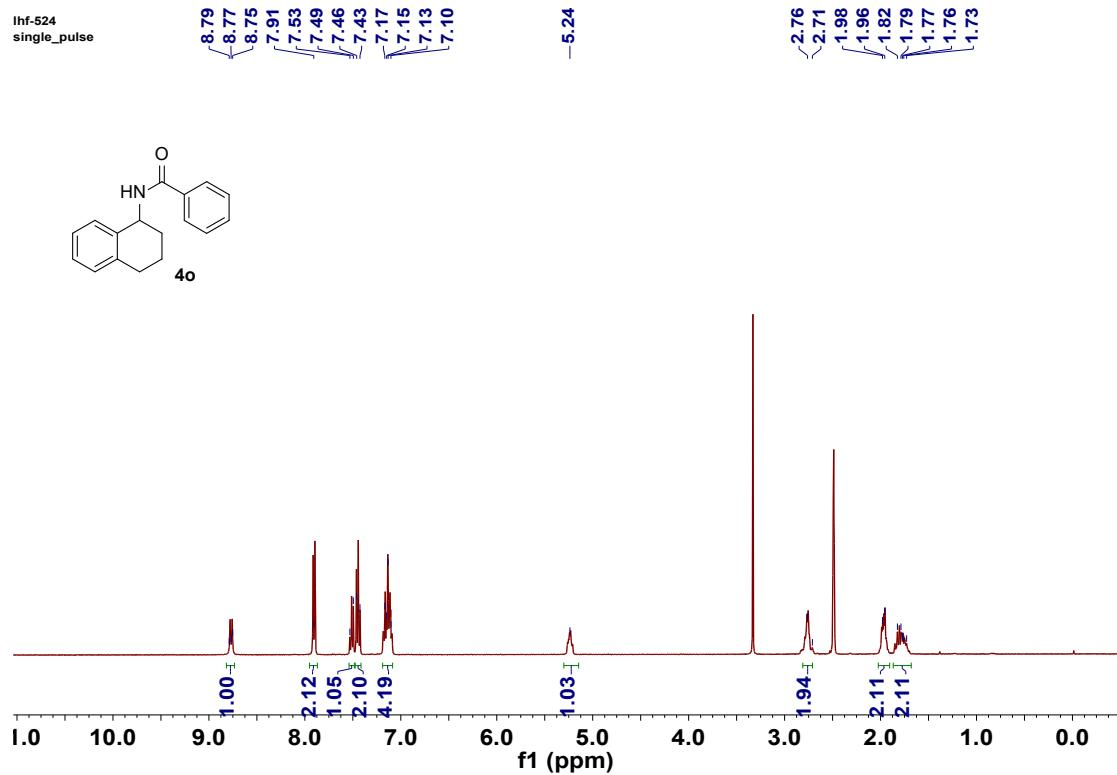
Figure S127. <sup>1</sup>H NMR spectrum of compound 4o (400 MHz, solvent: DMSO-*d*<sub>6</sub>)
