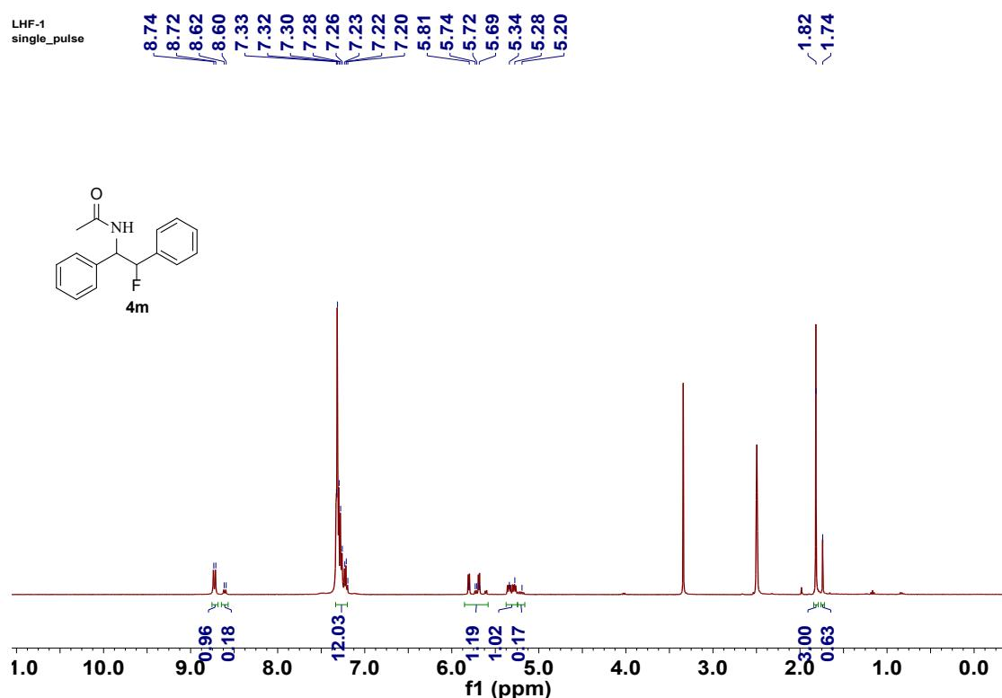
**Figure S120.**  $^1\text{H}$  NMR spectrum of compound **4m** (400 MHz, solvent: DMSO- $d_6$ ) *d.r.* = 5:1
