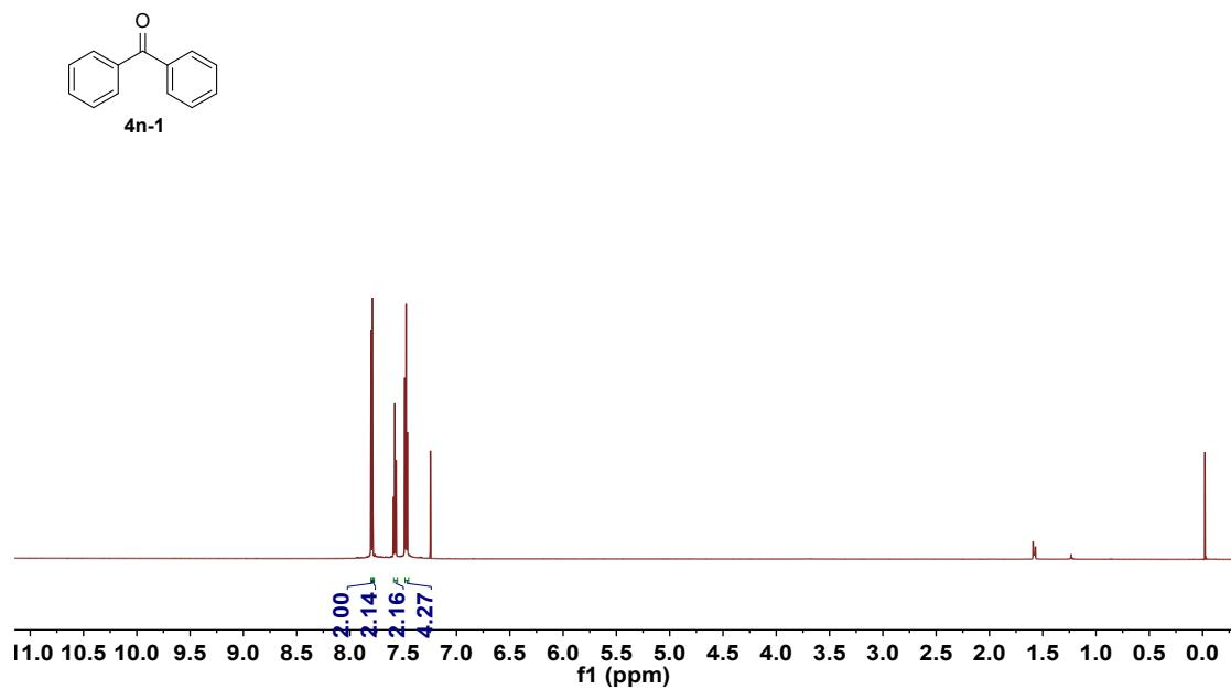
**Figure S125.**  $^1\text{H}$  NMR spectrum of compound **4n-1** (600 MHz, solvent:  $\text{CDCl}_3$ )
