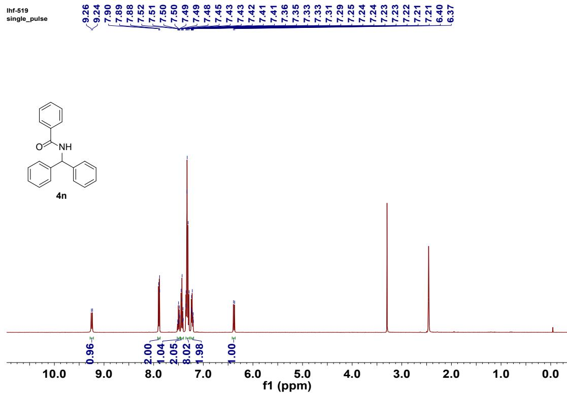
**Figure S123.**  $^1\text{H}$  NMR spectrum of compound **4n** (400 MHz, solvent: DMSO- $d_6$ )
