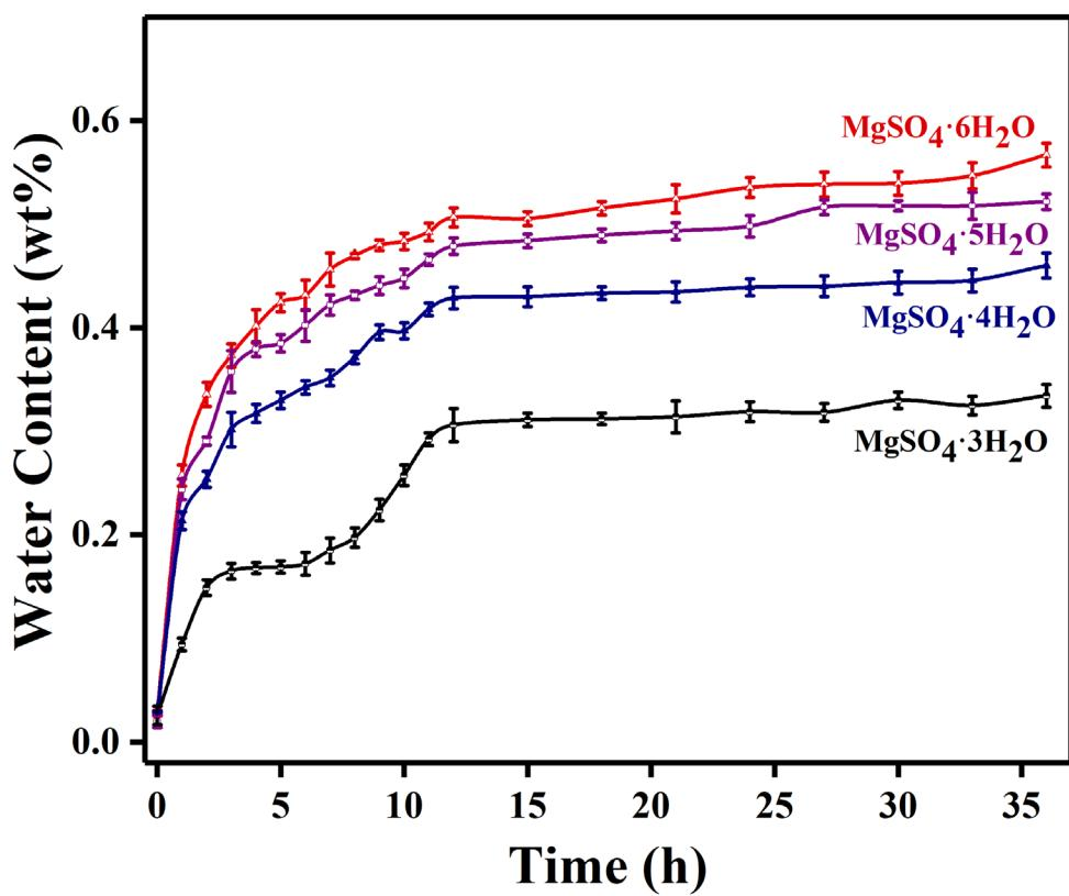
**Figure S1.** The water content of MgSO<sub>4</sub> hydrates as a function of time.
