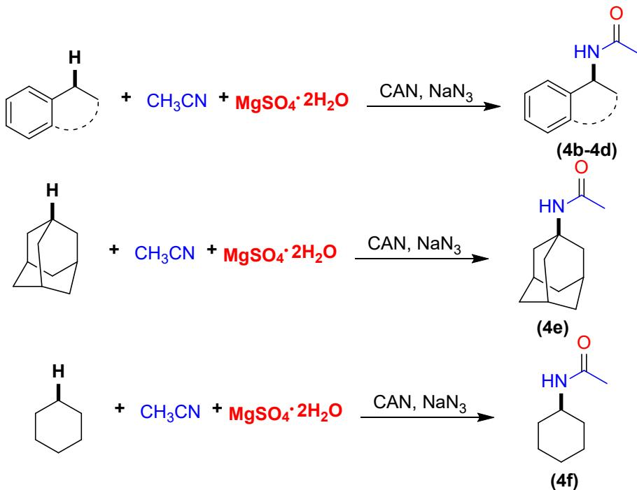
A deoxygenated solution of CAN (2.3 equiv.) in acetonitrile (30 mL) was added dropwise to a solution of substrates (1 equiv.), sodium azide (1.5 equiv.) and
