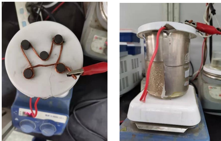
Fig. S2 Gram-scale electrolysis setup (graphite rods (*5): diameter 1.0 cm, length 10 cm, immersion depth 3.0 cm; nickel plate: width 23 cm, immersion depth 5.0 cm)
