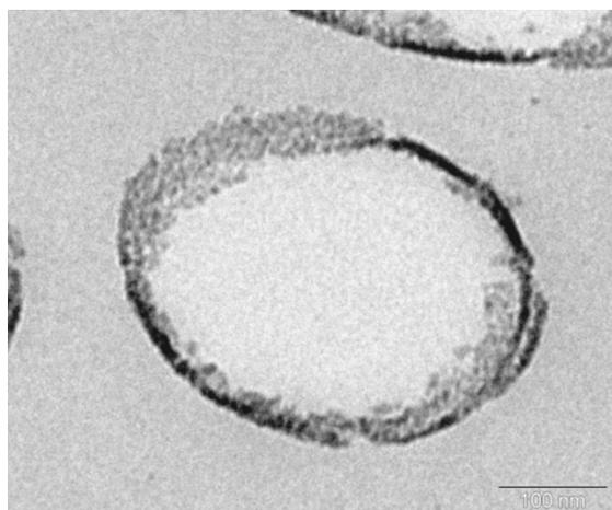
Figure S1: TEM image of a Pd-activated ion-track etched polycarbonate membrane, cut perpendicular to the pore axis.
