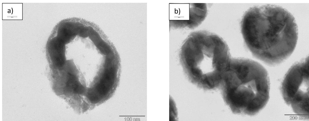
Figure S2: a, b) TEM images of cross-sections of electrolessly deposited Bi films in ion-track etched polycarbonate membranes using a higher DMAB concentration and longer plating time (100 mM DMAB, 120 h plating).
