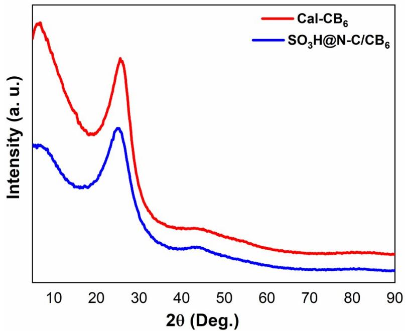
**Figure S2.** Powder XRD pattern of Cal-CB<sub>6</sub> and SO<sub>3</sub>H@N-C/CB<sub>6</sub>.
