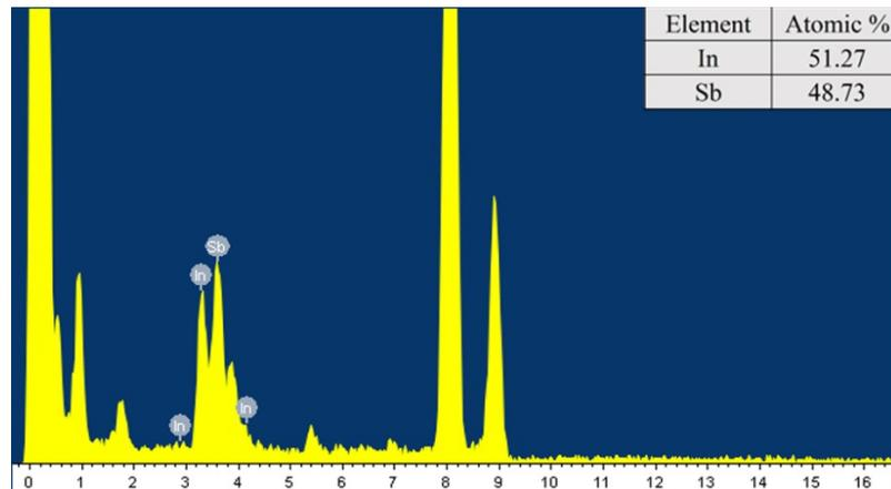
**Figure S9.** STEM-EDX spectra of a typical InSb nanowire stem. The signal of Cu and C arises from the TEM grid made of Cu.
