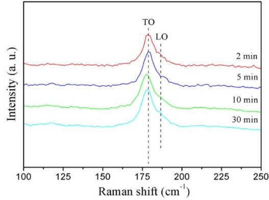
**Figure S7.** Raman spectra of the as-synthesized InSb nanowires with reaction times of 2 min, 5 min, 10 min, 30 min detected at room temperature detected at room temperatures were shown.
