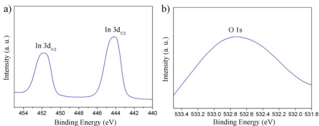
**Figure S1.** XPS spectra of the as-synthesized InSb nanowires. a) The In 3d core-level spectrum. b) The O 1s spectrum of the as-synthesized InSb nanowires.
