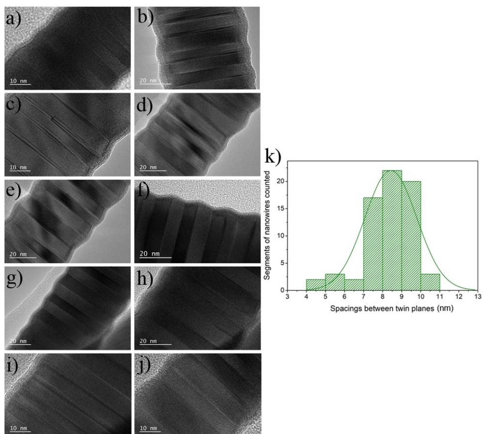
**Figure S3.** (a-j) TEM images for the as-prepared InSb twinning superlattice nanowires, and (k) the spacings between two consecutive twin planes for the InSb nanowires data are indicated in the histogram. The solid line shows a Gaussian fit of the spacings between twin planes distribution.
