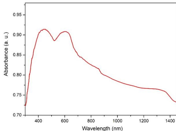
**Figure S2.** The room temperature UV-vis-NIR absorption spectra spectra of InSb twinning superlattice nanowires.
