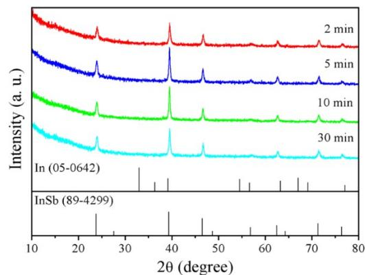
**Figure S6.** XRD patterns of the as-synthesized InSb nanowires with reaction times of 2 min, 5 min, 10 min, 30 min.
