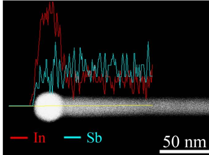
**Figure S10.** STEM-EDX line scan of a single InSb nanowire from the In tip. Red and light blue lines represent In and Sb elements, respectively.
