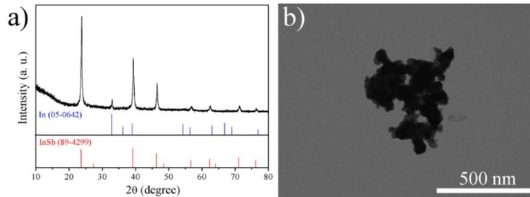
**Figure S8.** (a) XRD pattern, and (b) TEM image for the InSb nanocrystals prepared at about 175 °C for 60 s at the absence of TOP.
