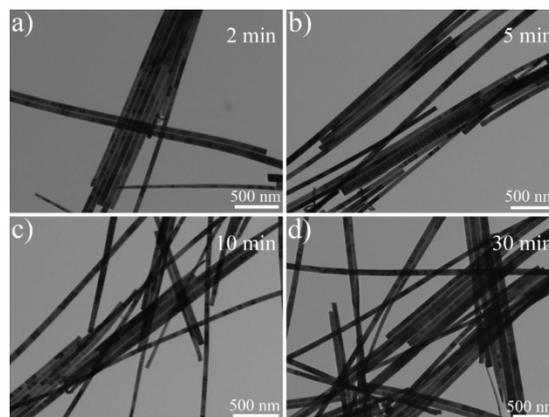
**Figure S5.** TEM images of InSb NWs with reaction times of 2 min, 5 min, 10 min, 30 min detected at room temperatures were shown.
