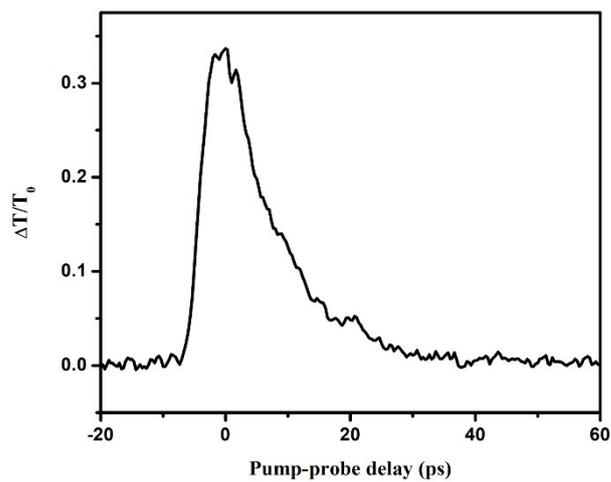
**Figure S11.** Pump-induced change in peak transmitted terahertz electric field ( $\Delta T/T_0$ ) for different pump-probe delays for InSb nanowires excited at 800 nm with an incident pump fluence of 50 mJ/cm<sup>2</sup>.
