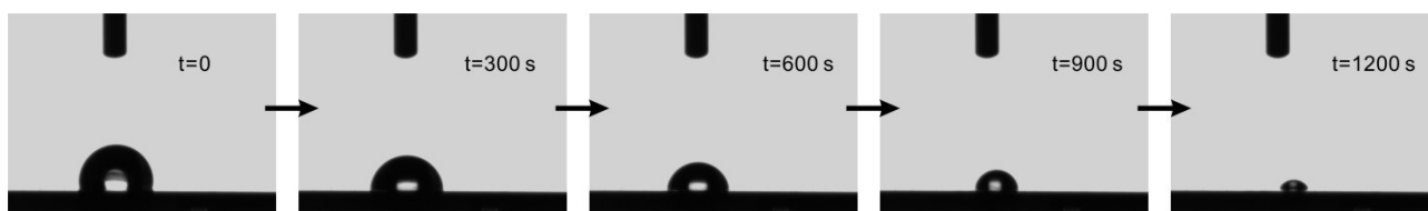
Fig.S1 Optical images of an aqueous droplet sitting on the hydrophobic silicon wafer at different states over time.
