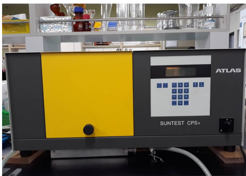
Figure S2. Photo of the solar simulator.
