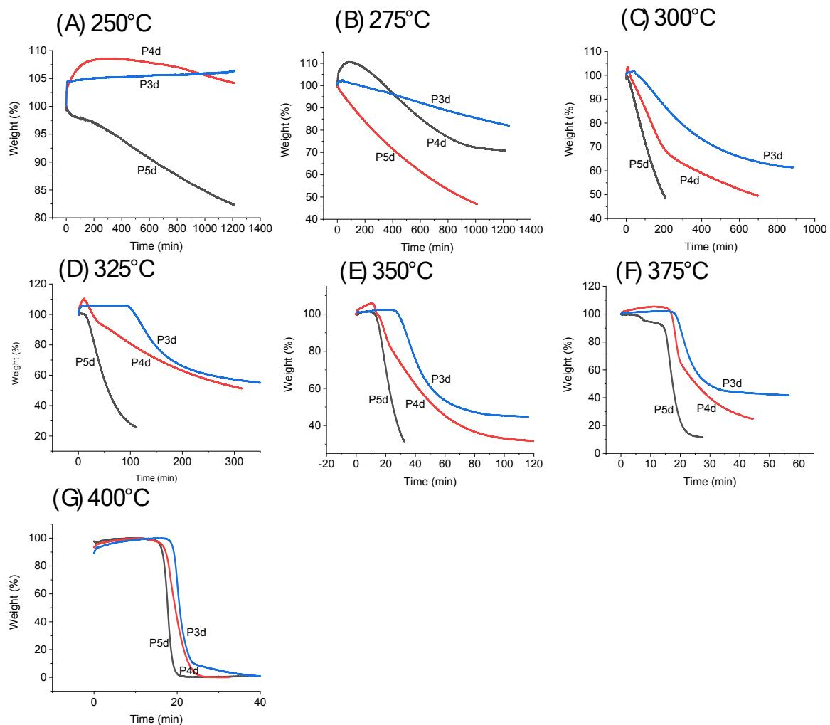
Figure S29 TGA weight-loss curves of polyesters **P3d**, **P4d** and **P5d** (reported earlier) by isothermal heating under nitrogen at the different temperatures, including (A) 250 °C, (B) 275 °C, (C) 300 °C, (D) 325 °C, (E) 350 °C, (F) 375 °C, and (G) 400 °C. The chemical structures of **P4d** and **P5d** are shown in Fig. S27.
