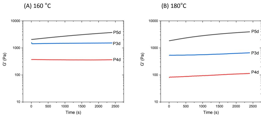
Figure S30. Shear storage modulus of **P3d**, **P4d** and **P5d** measured by rheology at the processing temperatures, 160 °C (A) and 180 °C (B).
