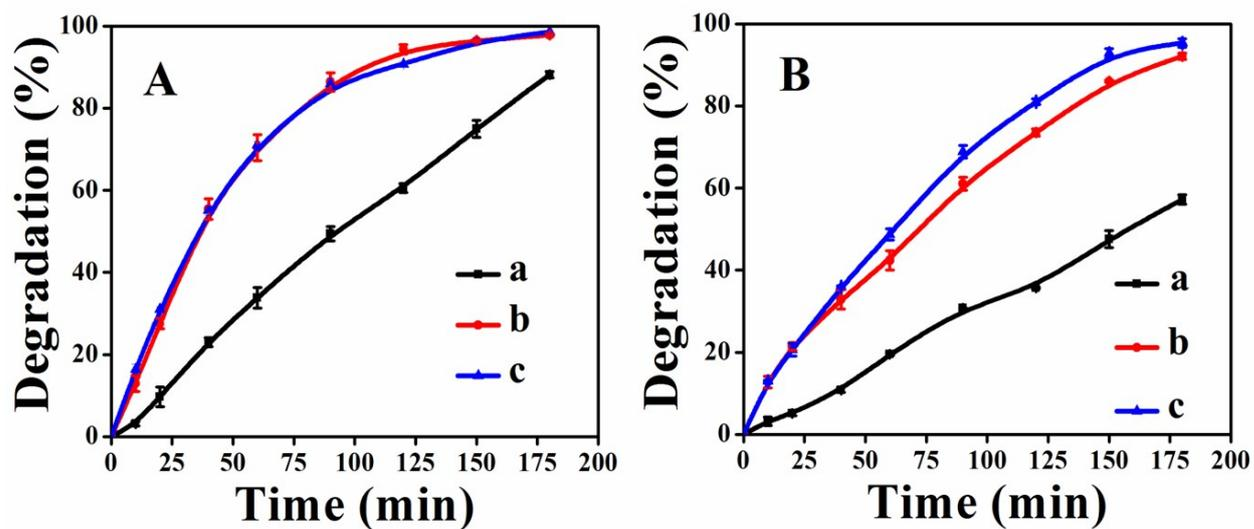
**Fig. S5.** Effect of various catalysts on the photo-catalytic degradation of CV (A) and MO (B) dyes. (a) ACP2, (b) ACP5, and (c) ACP7. Conditions: Initial concentration of dye = 0.0245 mM, catalyst dose = 0.5g/L, pH = 6.0, Room temperature.
