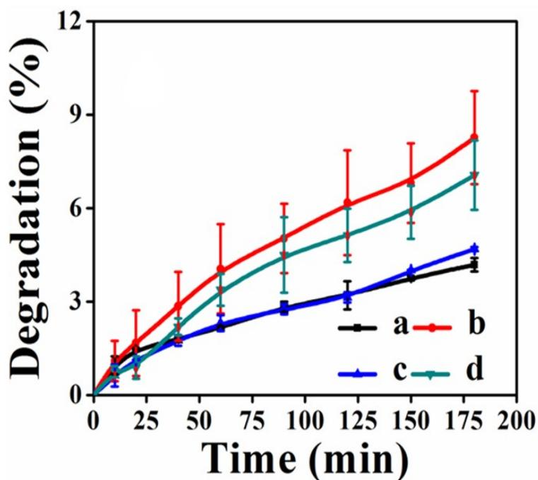
**Fig. S6.** Effect of UV-light alone (a and c), and bare CP (b and d) on the degradation of CV (a and b) and MO (c and d) dyes, respectively.
