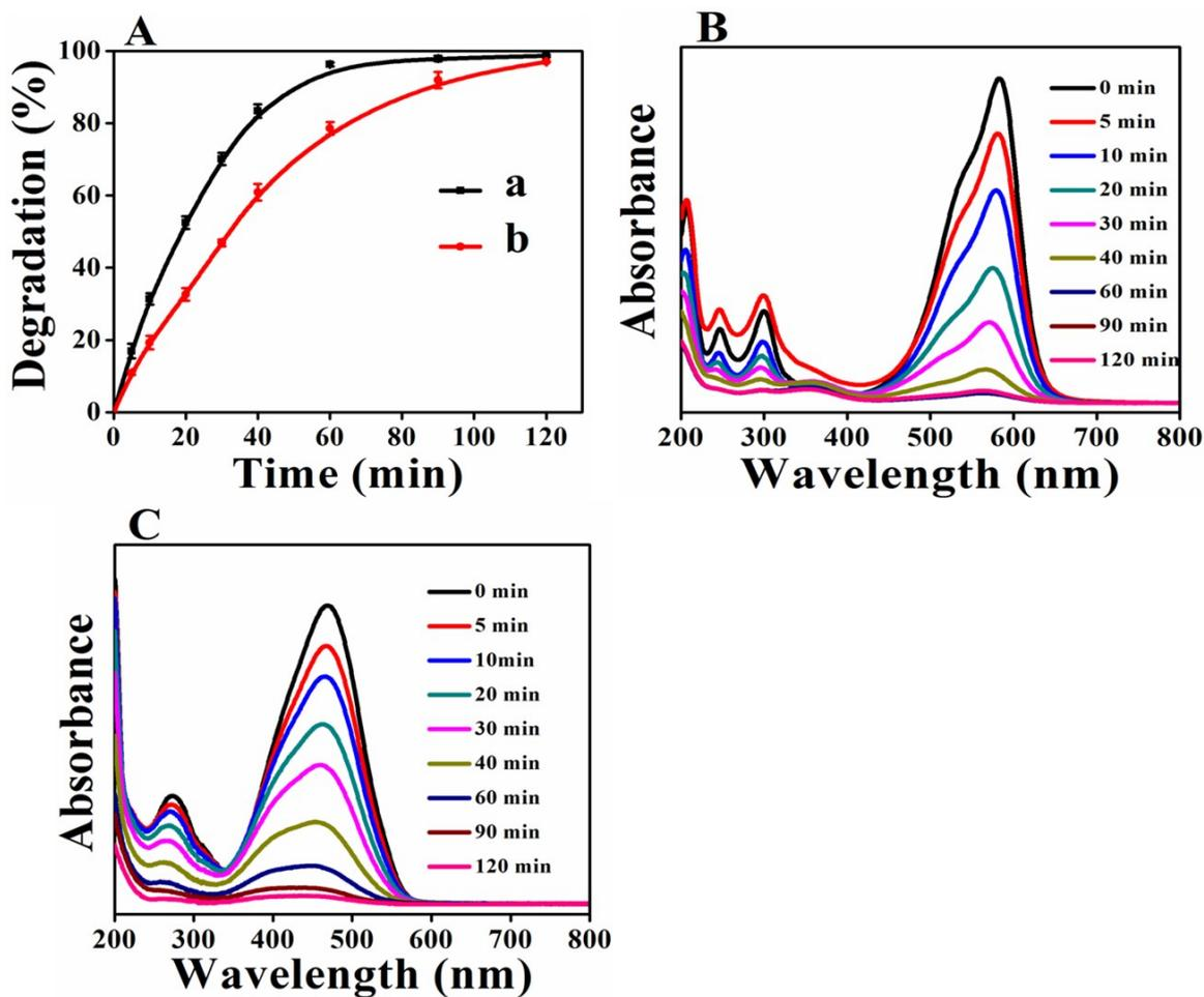
**Fig. S7.** A: Effect of irradiation time on the photo-catalytic degradation of CV (a) and MO (b) dyes. B: UV-Vis absorbance spectra of CV. C: UV-Vis absorbance spectra of MO at different irradiation time intervals, catalyzed by ACP6. Conditions: Initial concentration of dye = 0.0245 mM, catalyst dose = 0.75 g/L, pH = 8.0, Time = 120 min, and Room temperature.
