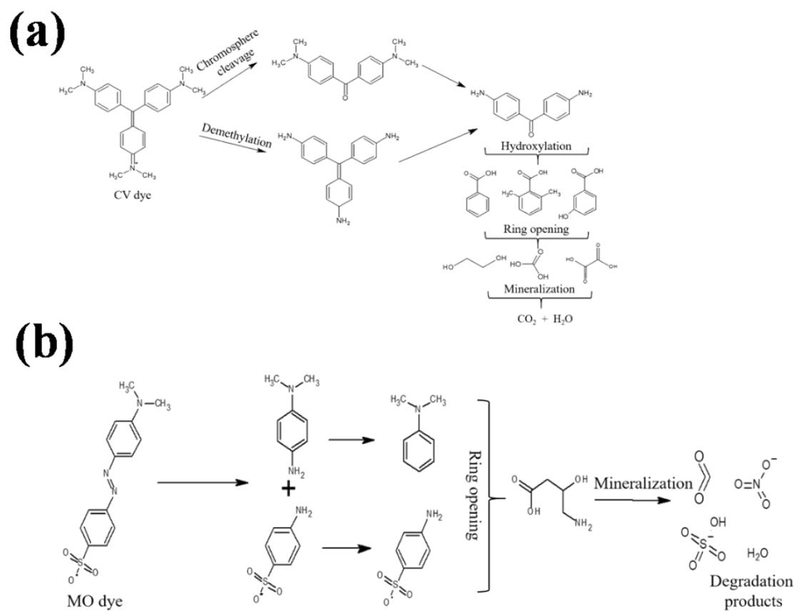
**Fig. S9.** Proposed degradation mechanisms of (a) CV and (b) MO dyes.
