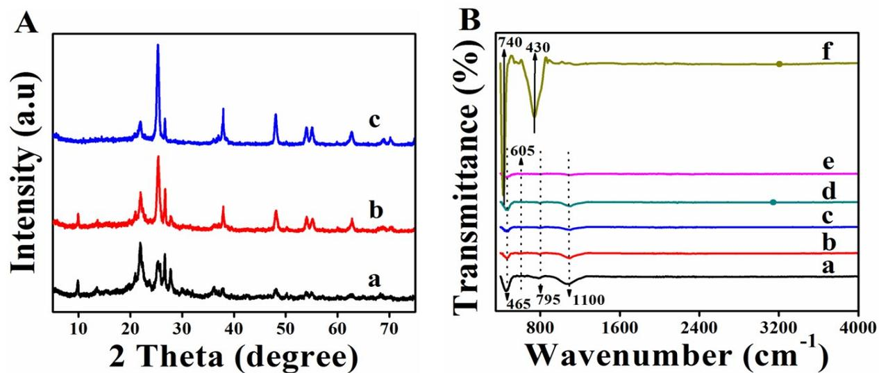
**Fig. S2.** XRD patterns (A) of (a) ACP2, (b) ACP5, and (c) ACP7 and FT-IR spectra (B) of (a) ACP1, (b) ACP2, (c) ACP4, (d) ACP5, (e) ACP7, and (f) anatase TiO<sub>2</sub>.
