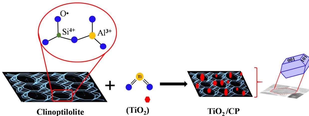
**Fig. S1.** Schematic illustration of the synthesis of TiO<sub>2</sub>/CPs.
