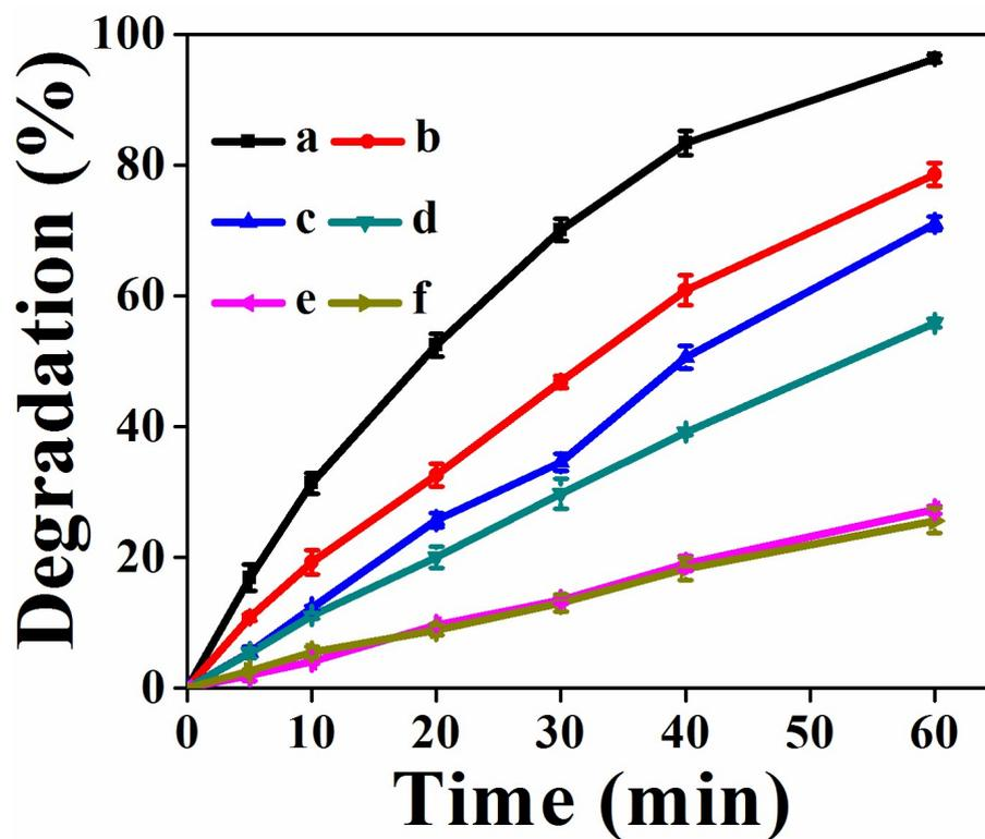
**Fig. S8.** Effect of radicals scavengers on the photocatalytic degradation of CV and MO dyes, a: CV degradation without scavengers, b: MO degradation without scavengers, c: CV degradation in the presence of isopropyl alcohol, d: MO degradation in the presence of isopropyl alcohol, e: CV degradation in the presence of benzoquinine, and f: MO degradation in the presence of benzoquinine.
