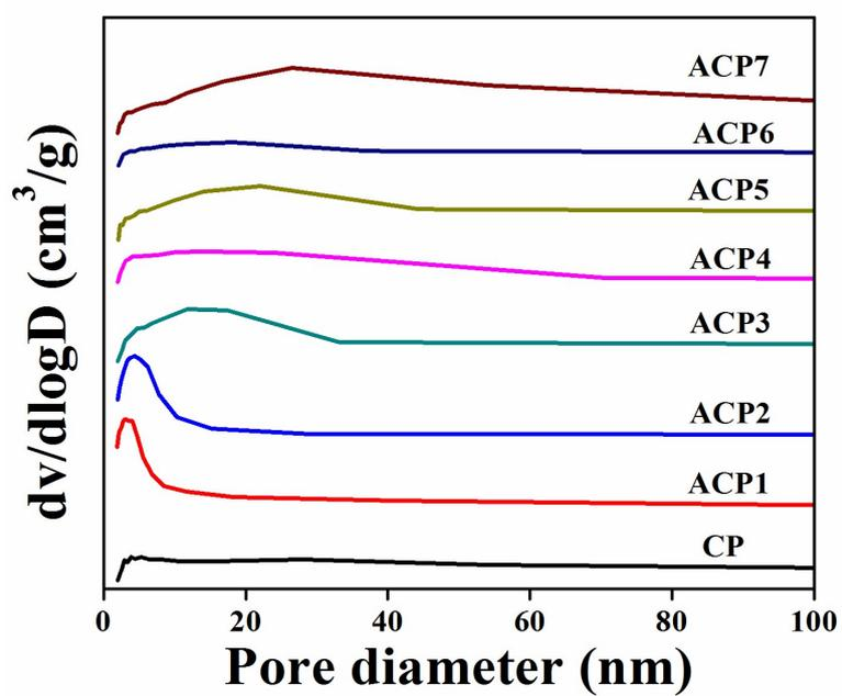
**Fig. S4.** Pore size distribution curves of  $\text{TiO}_2/\text{CPs}$  deriving from the desorption branch of the isotherms on the BJH model.
