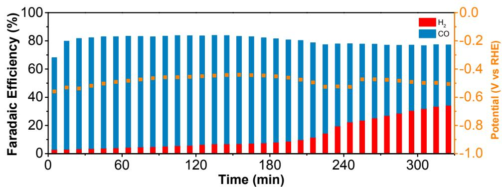
Fig. S9. Stability analysis of AgZn-CNF in 1 M KOH at -150 mA/cm<sup>2</sup>.
