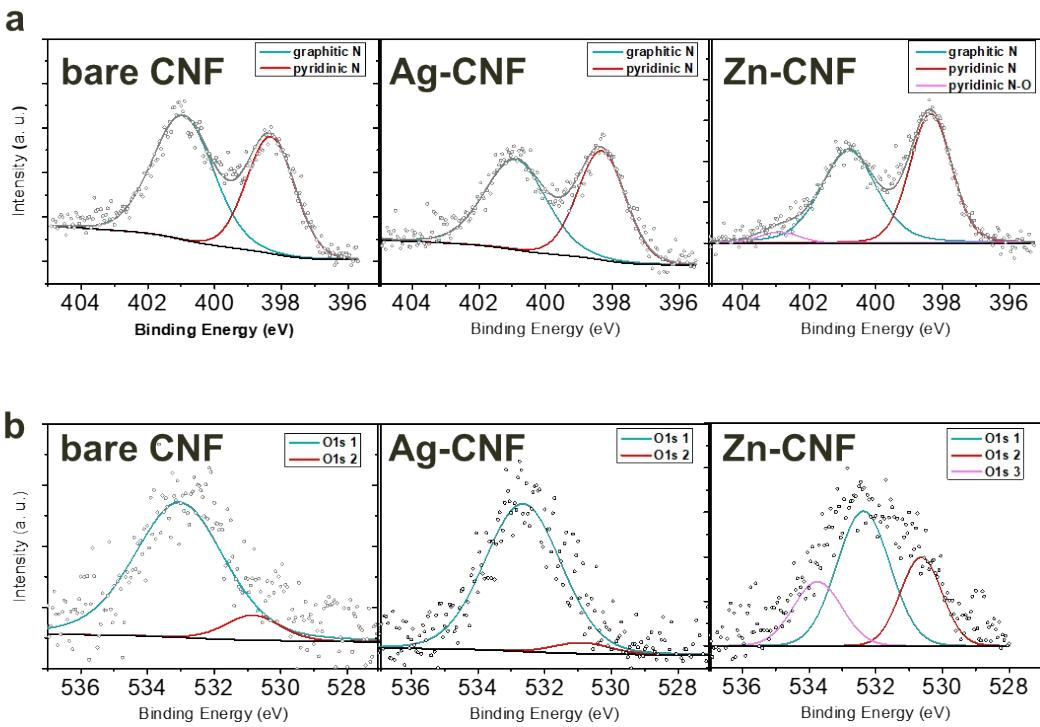
40 **Fig. S6.** XPS analysis (a) deconvolution result of N 1s of w/o metal, Ag-CNF and Zn-CNF (b) deconvolution
