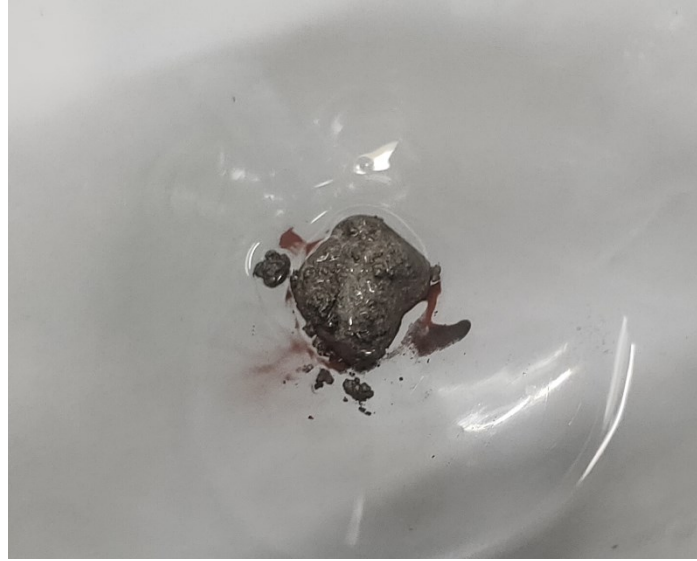
Fig. S3 Digital photograph of as-synthesized Cu@Sn-Bi using the purchased Sn-Bi alloy particles ( 10 \leq d \leq 25 \mu\text{m} ) as the precursor (Sample 7).
