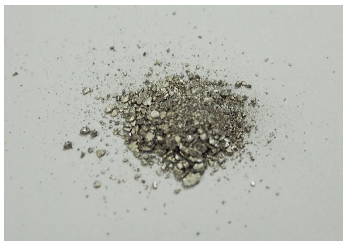
Fig. S2 Digital photograph of as-synthesized Cu@Sn-Bi at the stirring speed of 90 rpm (Sample 3).
