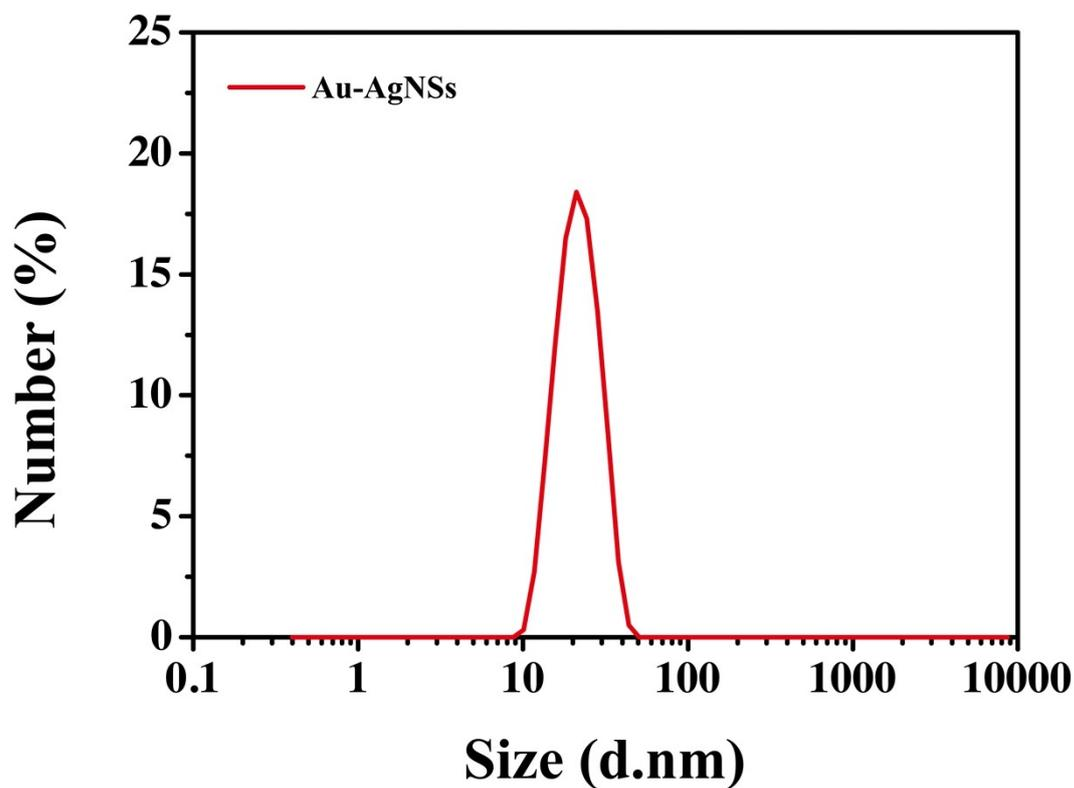
Fig. S1 Dynamic light scattering of Au-AgNSs.
