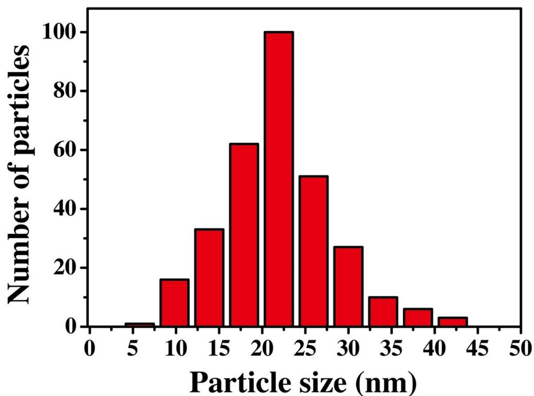
**Fig. S2** Particle size distributions of Au-AgNBs from SEM.
