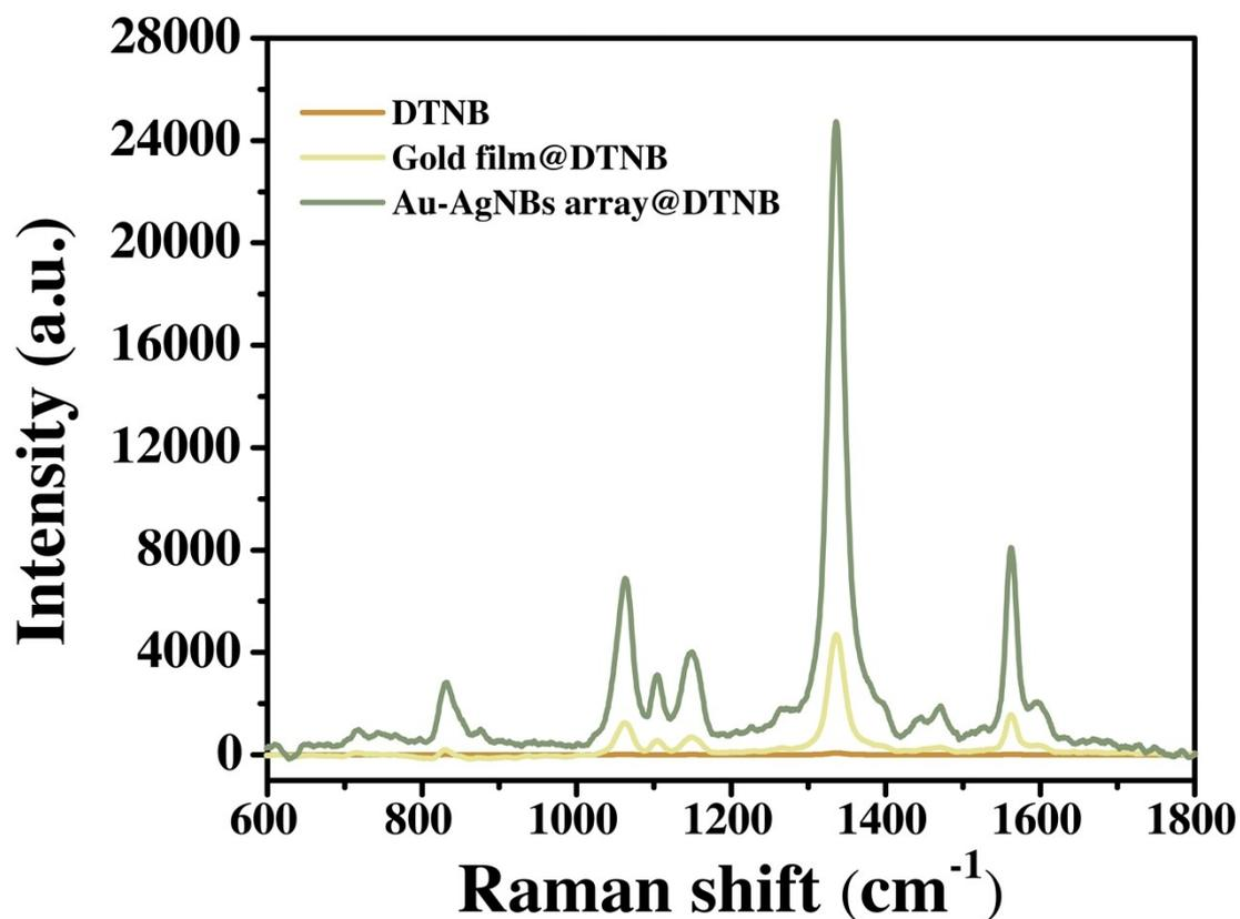
**Fig. S3** SERS spectra of the DTNB, DTNB-labeled gold film and DTNB-labeled Au-AgNBs array.
