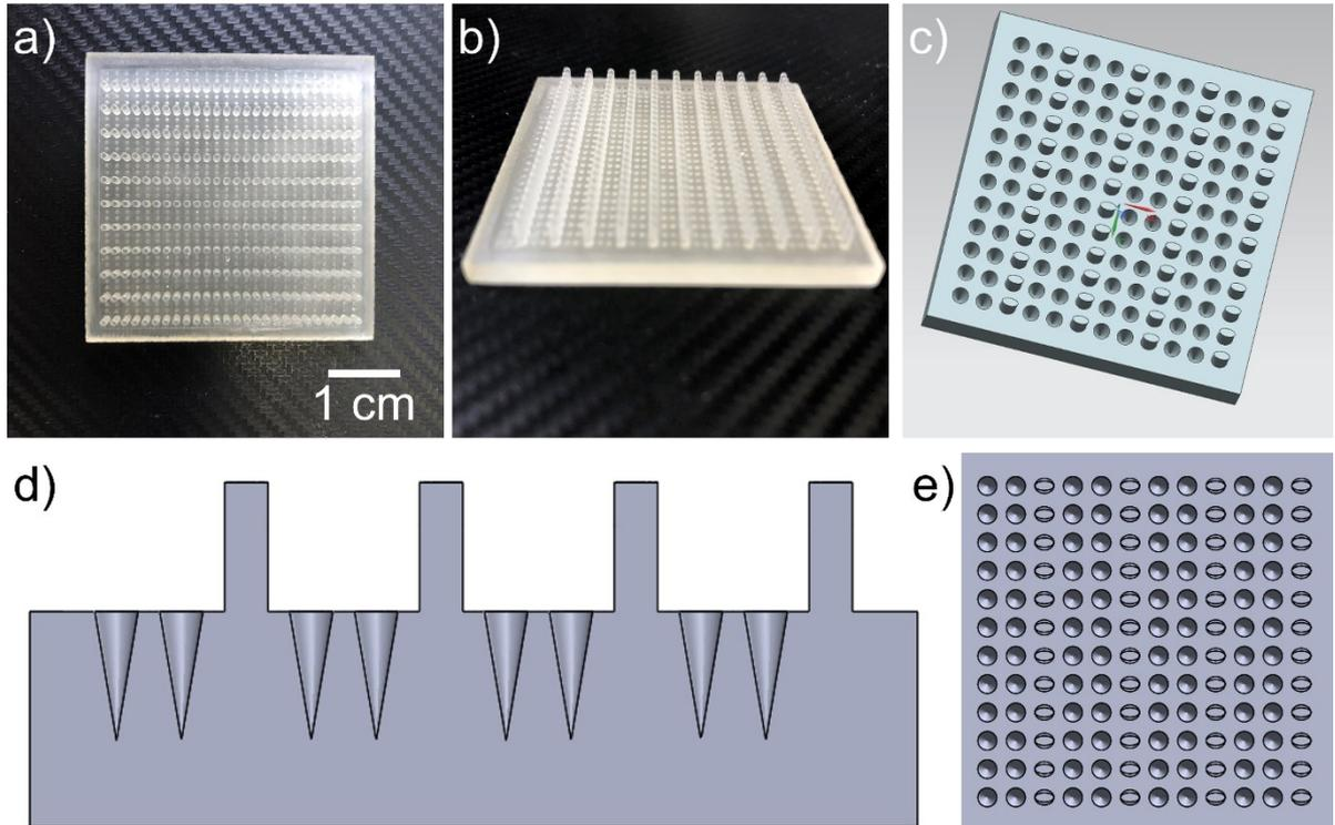
**Fig. S6** The model with negative topography. The model is composed by the raised pillar arrays and concave arrays. a-b) The optical images of the model. c-e) The sketches of the model
