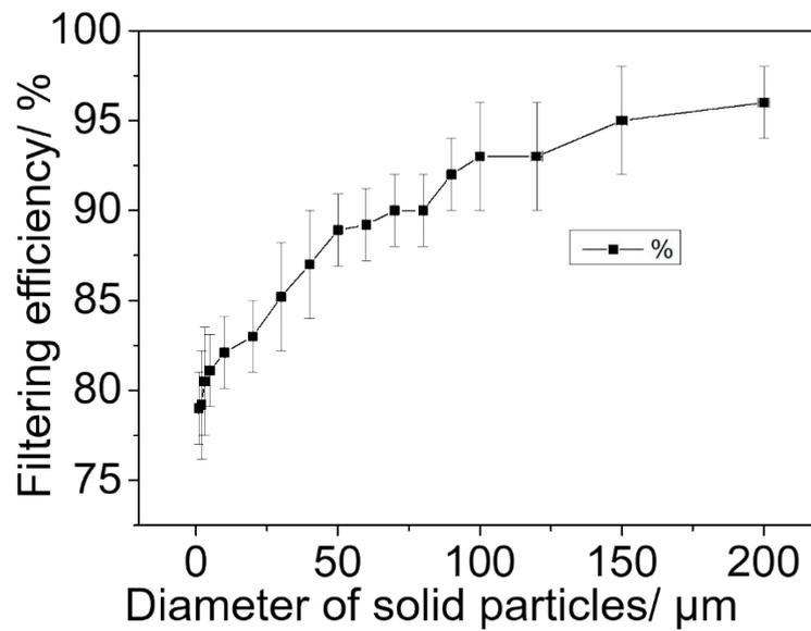
**Fig. S5 The filtering efficiency.** During the inhalation, solid particles in the air having a larger diameter are easily filtered. The filtering efficiency declines as the particle diameter decreases
