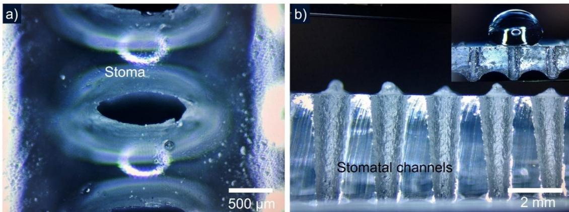
**Fig. S3** **a)** The long and short diameters of elliptical stomata are 1mm and 500  $\mu\text{m}$ , respectively. The space between two neighboring stomata is 500  $\mu\text{m}$ . **b)** The view on the surface from the other side. The stomatal channels have a height of 4 mm. The inset shows the state of the droplet on the surface
