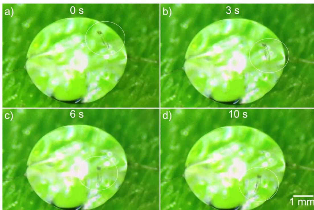
**Fig. S1** A solid particle is captured and wetted by a water droplet. The solid particle flows inside the droplet. The air is filtered by the droplet
