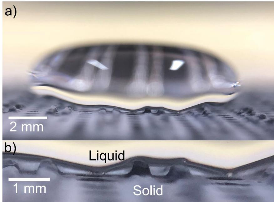
**Fig. S4** The side view of the solid/liquid interface of the bio-fabricated surface. The liquid suspends on the top region of micro-setae and hardly directly contact with the stomata
