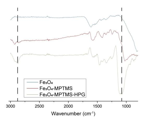
**Figure S1.** IR spectra of the synthesized and later functionalized iron oxide particles with their corresponding functionalization (MPTMS and HPG). Typical PG IR bands can be observed, C-H (s): 2850 cm<sup>-1</sup> and C-O-C (vs): 1100 cm<sup>-1</sup>.
