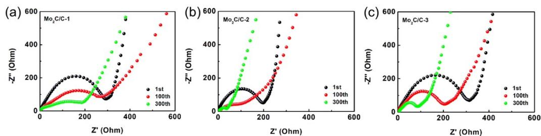
Fig. S7 Nyquist plots of (a) Mo<sub>2</sub>C/C-1, (b) Mo<sub>2</sub>C/C-2, and (c) Mo<sub>2</sub>C/C-3 during cycling test.
