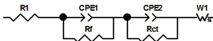
Fig. S6 The equivalent circuit of impedance spectra of Mo<sub>2</sub>C/C nanosheet composites.
