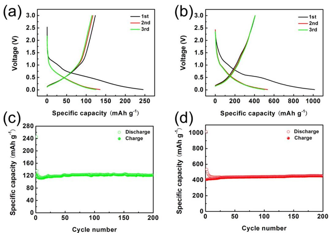
Fig. S5 The initial three charge/discharge curves of (a) p-C and (b) Mo<sub>2</sub>C/C-4; Cycling performances of (c) p-C and (d) Mo<sub>2</sub>C/C-4 at 0.2 A g<sup>-1</sup>.
