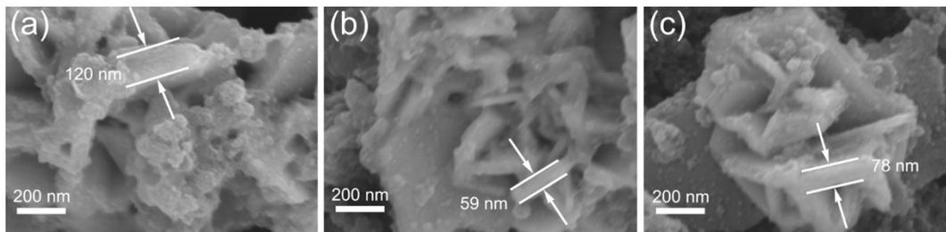
Fig. S4 SEM images of (a) Mo<sub>2</sub>C/C-1, (b) Mo<sub>2</sub>C/C-2, and (c) Mo<sub>2</sub>C/C-3 after 300 cycles at the current density of 0.2 A g<sup>-1</sup>.
