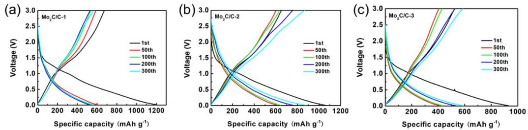
Fig. S3 The galvanostatic charge/discharge curves of (a) Mo<sub>2</sub>C/C-1, (b) Mo<sub>2</sub>C/C-2, and (c) Mo<sub>2</sub>C/C-3 at different cycles.
