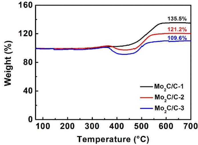
Fig. S2 TGA curves of various Mo<sub>2</sub>C/C nanosheet composites in air.
