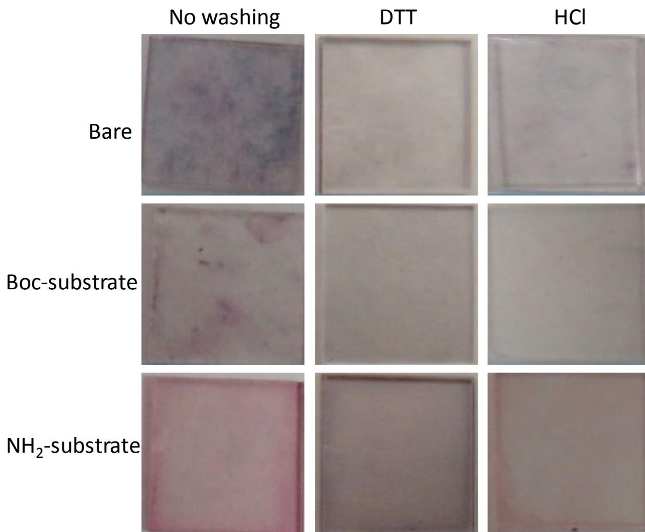
Fig. S6 Photographs of the AuNPs-immobilized substrates (1 cm × 1 cm, 0.5 mm thick). Insets of Fig. 3a.
