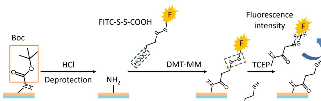
Fig. S3 Schematic illustration of the process to quantify amino groups displayed on the PMMA substrate.
