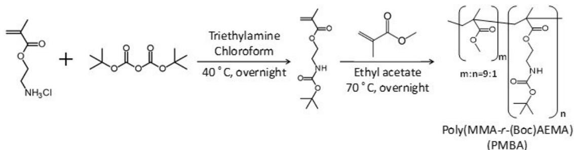
Fig. S1 Synthesis of a functional polymer (PMBA).
