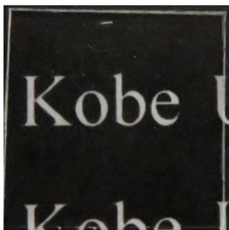
Fig. S5 Transparency of an acrylic substrate after dip-coating and deprotection.
