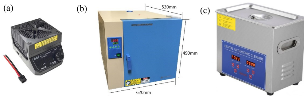
Figure S2. Equipment requirement (a) Battery module discharger, (b) High temperature oven and (c) Ultrasonic cleaner
