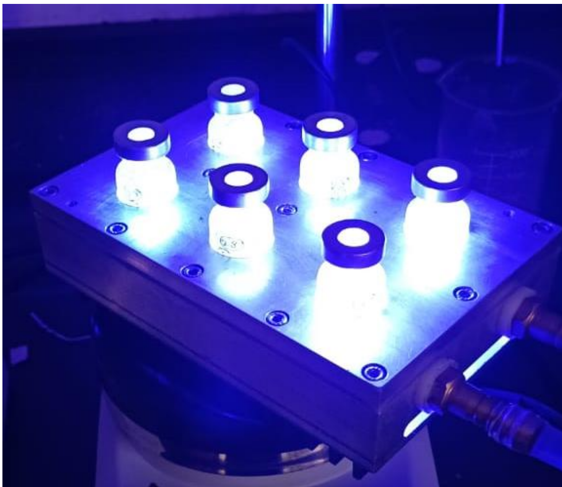
Figure 1: Blue LED reactor with magnetic stirring plate
