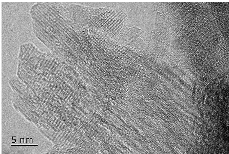
Figure S3. HRTEM spectra of prepared CuFe NP/IF.
