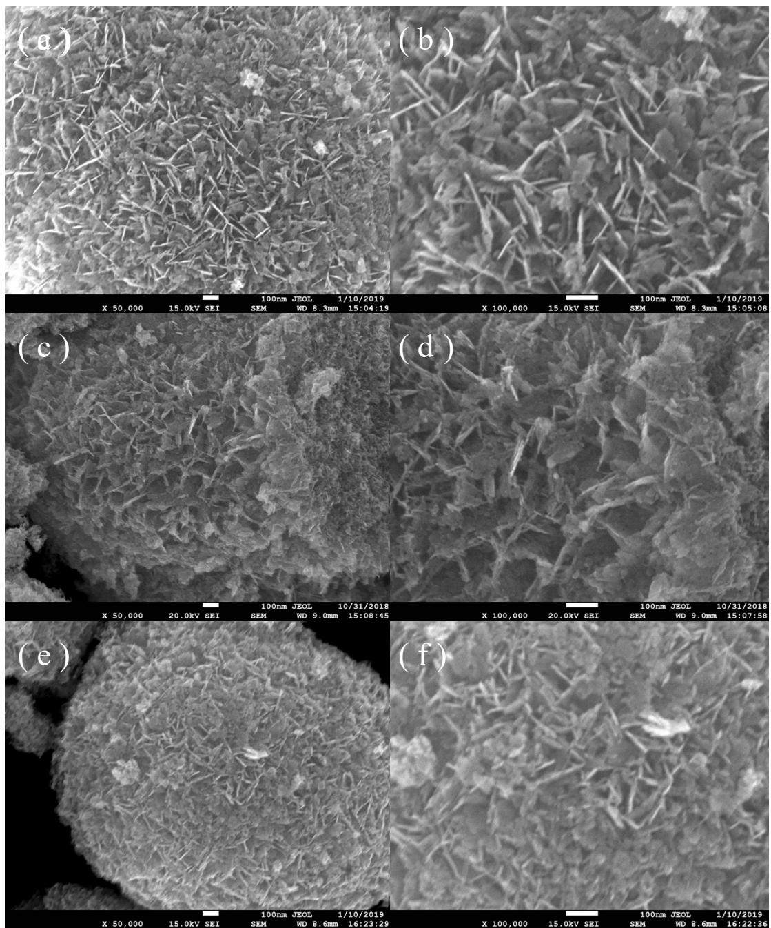
**Fig. S2** FE-SEM images of BMO-SOVs(a,b), Au/BMO(c,d) and CQDs/BMO(e,f).
