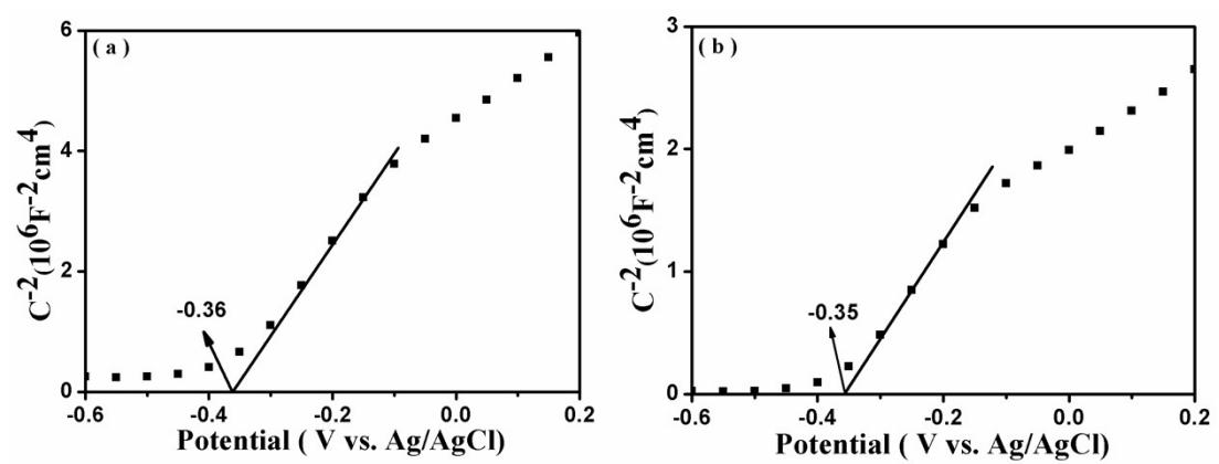
**Fig. S7** Mott-Schottky plots of (a) BMO and (b) BMO-SOVs.
