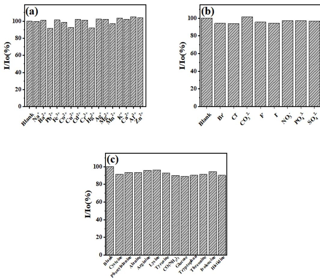
**Figure S7.** Selectivity experiments of the CDs sensor towards (a) cation ions, (b) anion ions and (c) various compounds.
