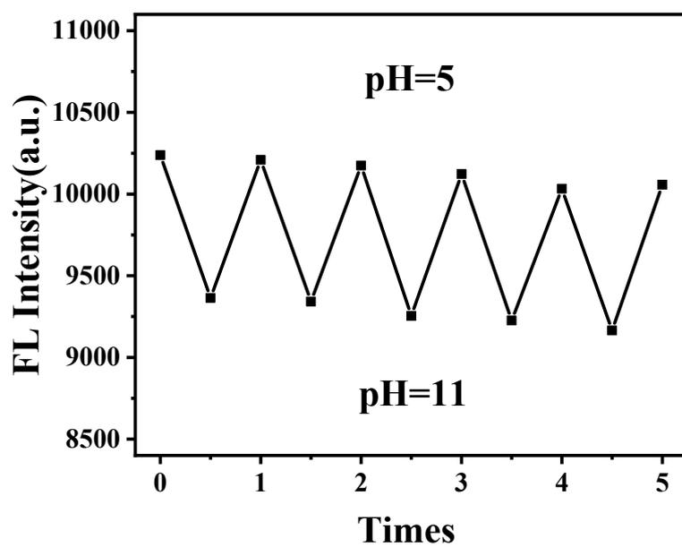
**Figure S6.** FL intensity upon the cyclic switching of CDs under alternating conditions of pH =5 and pH = 11.
