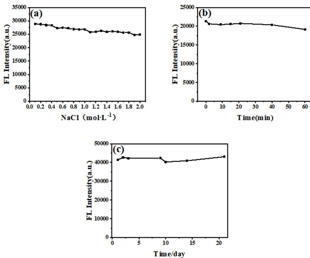
**Figure S5.** (a) Effect of the concentration of NaCl from 0 to 2 M and increase with 0.1 M increments on the FL intensities of CDs. (b) FL intensity of the as-prepared CDs during continuous excitation at 365nm with a UV beam. (c) FL stability of the as-prepared CDs for 20 days at room temperature in air-tight closed tubes.
