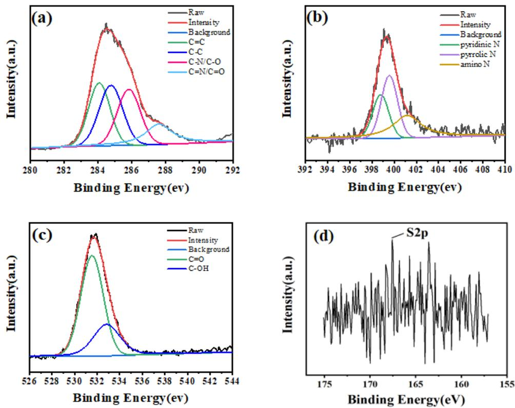
Figure S2. High-resolution XPS spectra of (a) C, (b) N, (c) O, and (d) S
