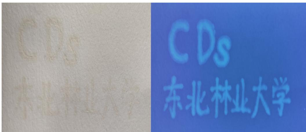
**Figure S4.** Image of CDs and fluorescence patterns under visible light and a UV beam of 365 nm.
