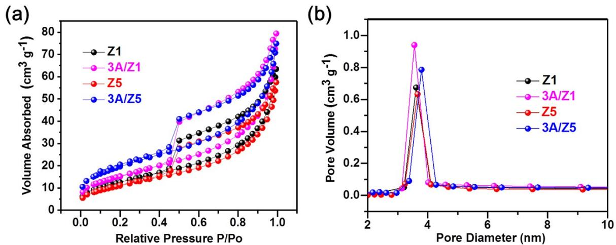
**Figure S7.** (a) N<sub>2</sub> adsorption-desorption isotherms and (b) the pore size distribution curve of Z1, 3A/Z1, Z5, 3A/Z5.
