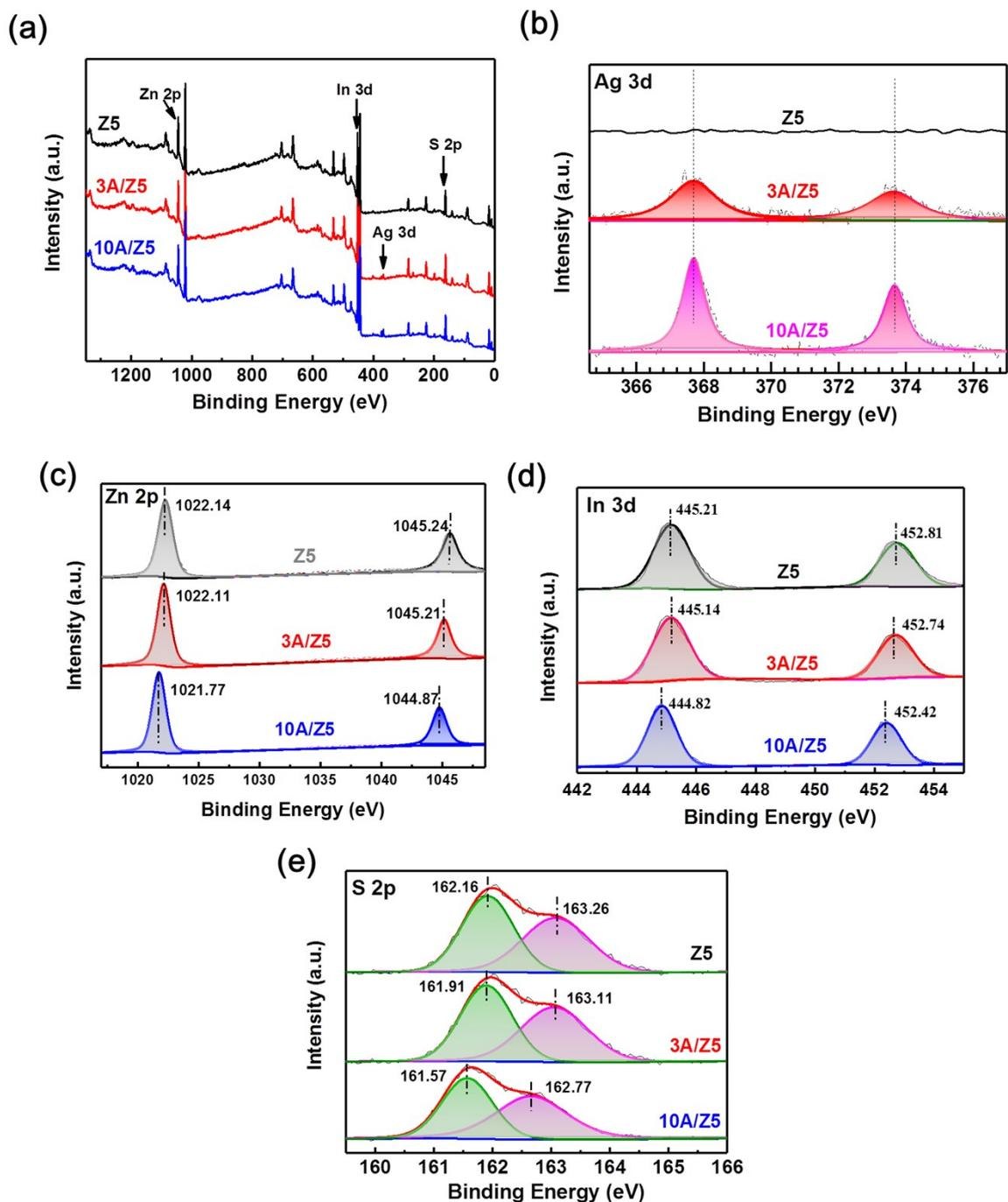
**Figure S3.** (a) XPS survey spectra, (b) Ag 3d, (c) Zn 2p, (d) In 3d and (e) S 2p of the Z5, 3A/Z5 and 10A/Z5 samples.
