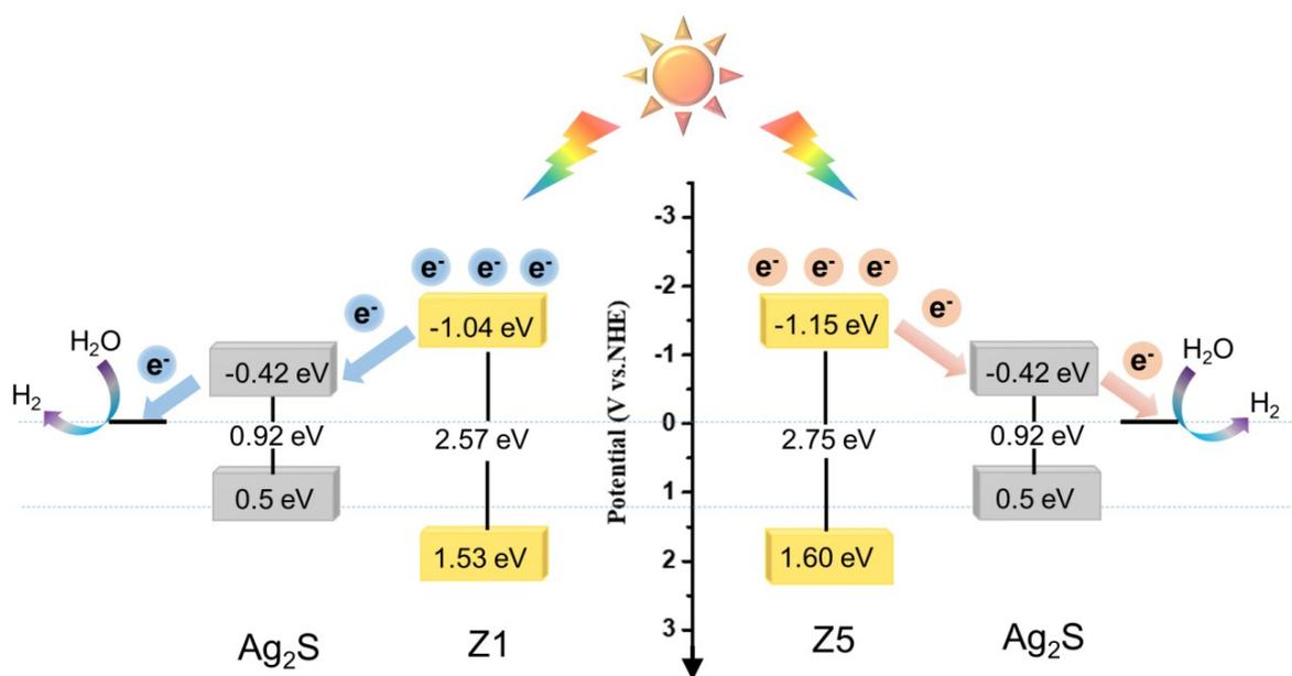
**Figure S10.** Energy band diagram of Z1, Z5 and Ag<sub>2</sub>S.
