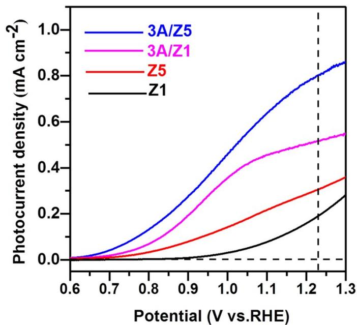
**Figure S13.** Current–potential curves for photoelectrodes made of Z1, 3A/Z1, Z5 and 3A/Z5 measured in an aqueous solution without  $\text{Na}_2\text{SO}_3$  (pH =6.8).
