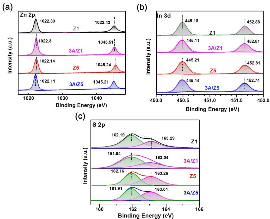
**Figure S2.** XPS spectra of the (a) Zn 2p, (b) In 3d and (c) S 2p in the Z1, 3A/Z1, Z5 and 3A/Z5 samples.
