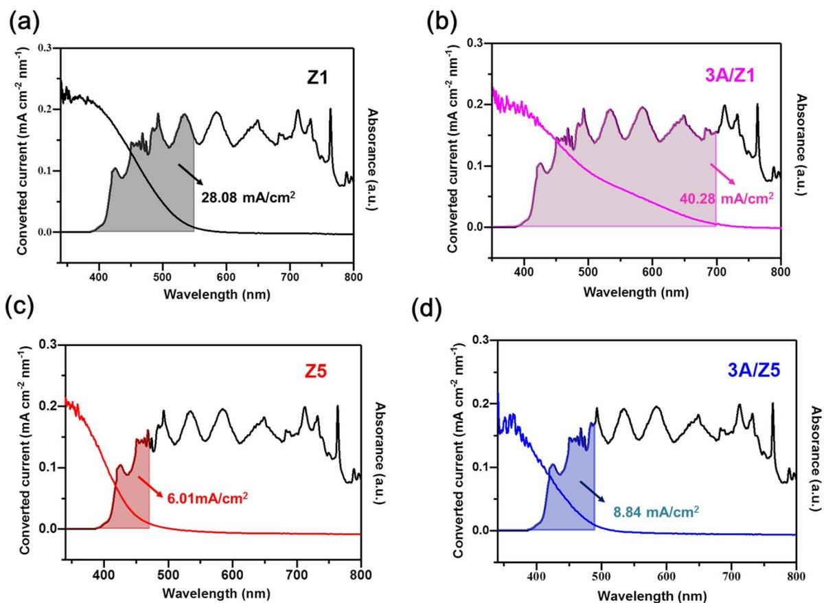
**Figure S14.** Theoretical photocurrent intensity of (a) Z1, (b) 3A/Z1, (c) Z5 and (d) 3A/Z5 according to light absorption.
