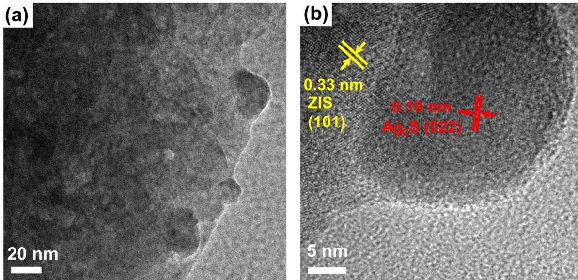
**Figure S6.** (a) TEM image and (b) HRTEM image of the 100A/Z5.
