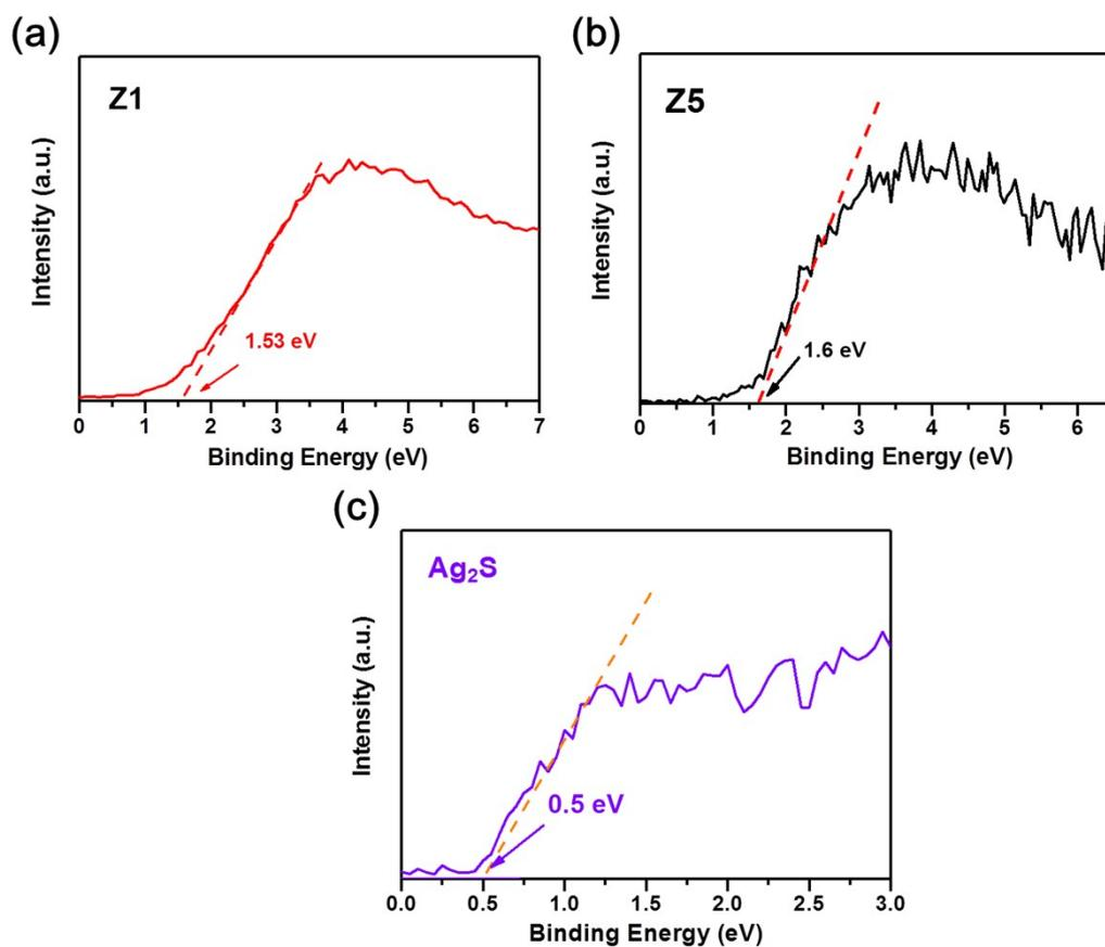
Figure S9. XPS valence spectra of (a) Z1, (b) Z5 and (c)  $\text{Ag}_2\text{S}$ .
