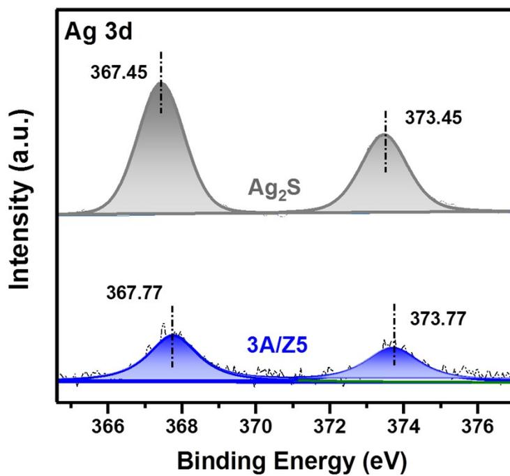
**Figure S4.** XPS spectra of Ag 3d of the Z1, 3A/Z1, Z5 and 3A/Z5 samples.
