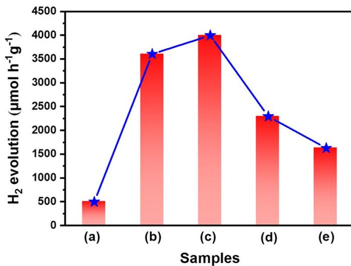
**Figure S11.** H<sub>2</sub> evolution rates of (a) Z5, (b) 1A/Z5, (c) 3A/Z5 (d) 5A/Z5 and (e) 10A/Z5.
