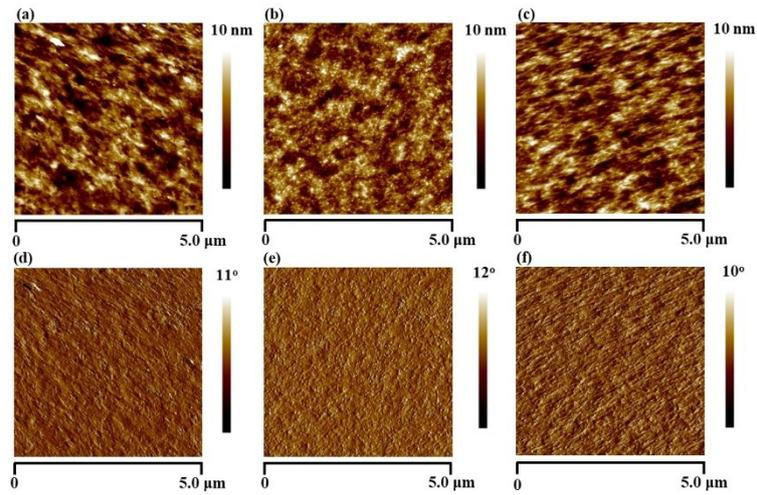
**Fig.S24** AFM height images (a), (b), (c) and phase images (d), (e), (f) for, the PBDB-T-2Cl: BDSeTICBr- $\gamma$  film, PBDB-T-2Cl: BDSeTICBr- $\delta$  film and PBDB-T-2Cl: BDSeTICBr-m film, respectively.
