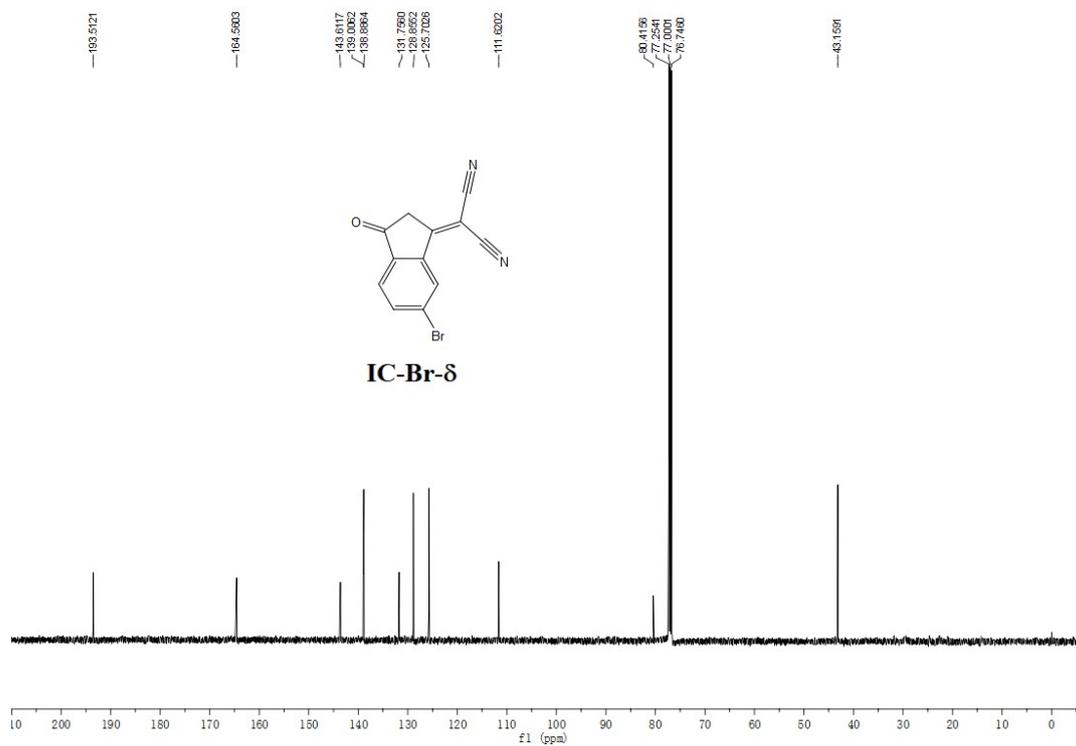
Fig.S6 The  $^{13}\text{C}$  NMR spectrum of IC-Br- $\delta$ .
