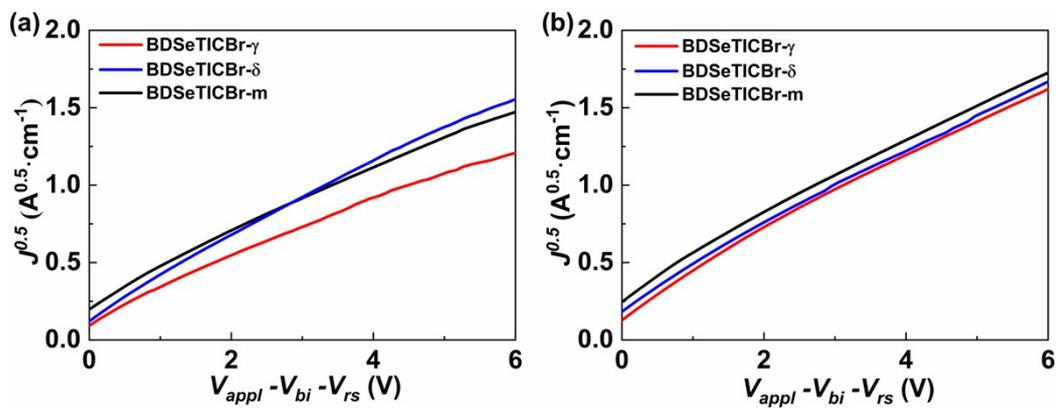
**Fig.S21**  $J^{0.5}$  vs  $V$  ( $V = V_{appl} - V_{bi} - V_{rs}$ ) plots for electron-only (a) and hole-only (b) devices of the PBDB-T-2Cl:SMA blends.
