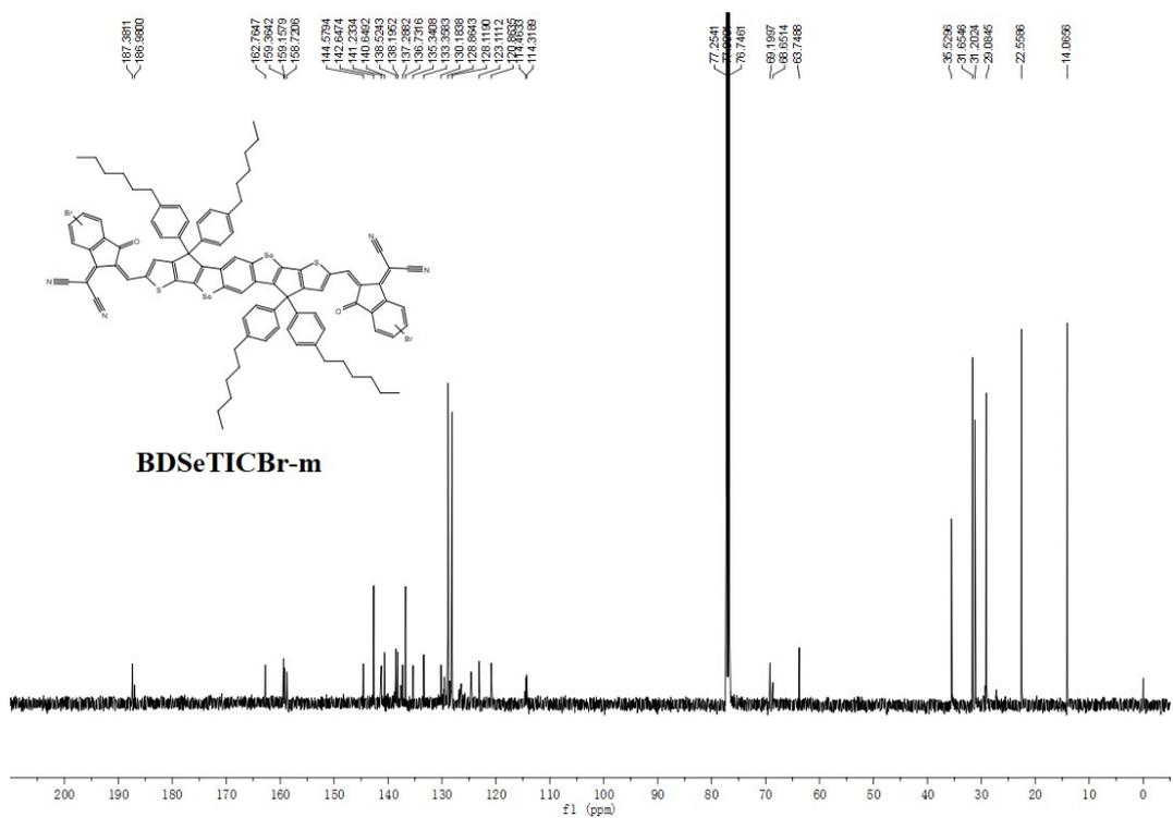
**Fig.S8** The <sup>13</sup>C NMR spectrum of BDSeTICBr-m.
