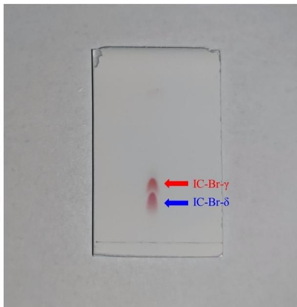
**Fig.S1** The thin layer chromatography (TLC) picture of IC-Br-m with ethyl acetate: propionic acid (v:v = 50:1) as the eluent.
