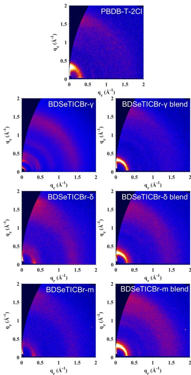
**Fig.S25** GIWAXS scattering patterns of the neat films of the PBDB-T-2Cl, BDSerTICBr- $\gamma$ , BDSerTICBr- $\delta$  and BDSerTICBr-m and their PBDB-T-2Cl:SMA blend films.
