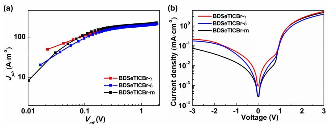
**Fig.S20** Photogenerated current density versus effective voltage curves under AM 1.5G illumination (a) and  $J$ - $V$  curves from -3 V to +3 V in dark (b).
