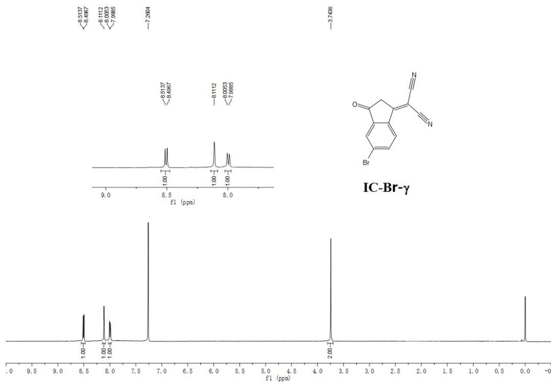
Fig.S3 The  $^1\text{H}$  NMR spectrum of IC-Br- $\gamma$ .
