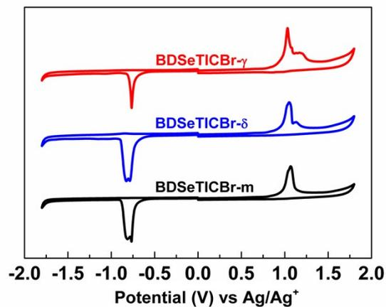
**Fig.S17** Cyclic voltammogram of the BDSeTICBr- $\gamma$ , BDSeTICBr- $\delta$  and BDSeTICBr-m film in 0.1 M  $\text{Bu}_4\text{NPF}_6$  solution in  $\text{CH}_3\text{CN}$  with a scan rate of  $80 \text{ mV}\cdot\text{s}^{-1}$ .
