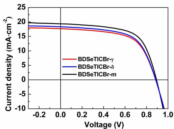
**Fig.S19** The typical  $J$ - $V$  curves of the optimized PBDB-T-2Cl: SMA PSCs under AM 1.5G irradiation.
