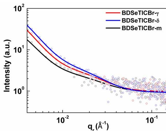
**Fig.S23** GISAXS in-plane profiles of the PBDB-T-2Cl:SMA blend films and their model fittings with the Debye-Anderson-Brumberger (DAB) model.
