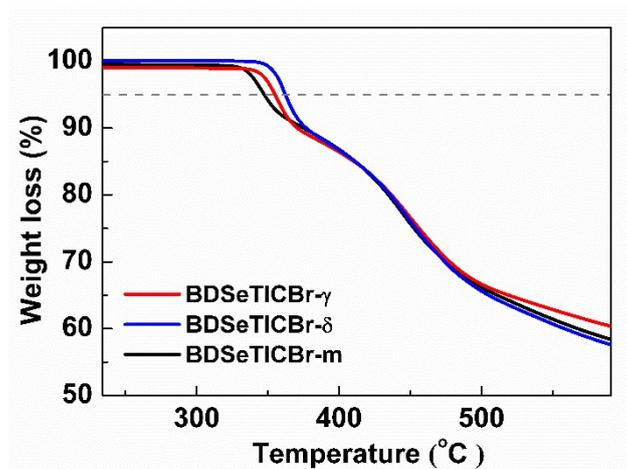
Fig.S16 Thermal gravimetric analysis (TGA) curves of BDSerTICBr- $\gamma$ , BDSerTICBr- $\delta$  and BDSerTICBr-m at a heating rate of  $10\text{ }^{\circ}C\cdot\text{min}^{-1}$  under  $N_2$ .
