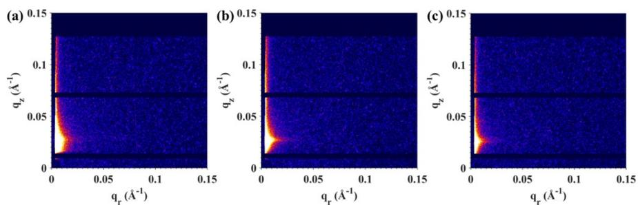
**Fig.S22** GISAXS patterns of the PBDB-T-2Cl:BDSeTICBr- $\gamma$  (a), PBDB-T-2Cl:BDSeTICBr- $\delta$  (b) and PBDB-T-2Cl:BDSeTICBr-m (c) film.
