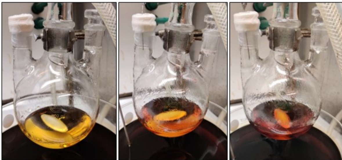
Fig. S1. Initial PEI solution (left), PEI solution after addition of 1-methyl-piperazine and 2 hours at 90°C (center), and the solution after the final heating state (2.5 hours at 110°C, right).
