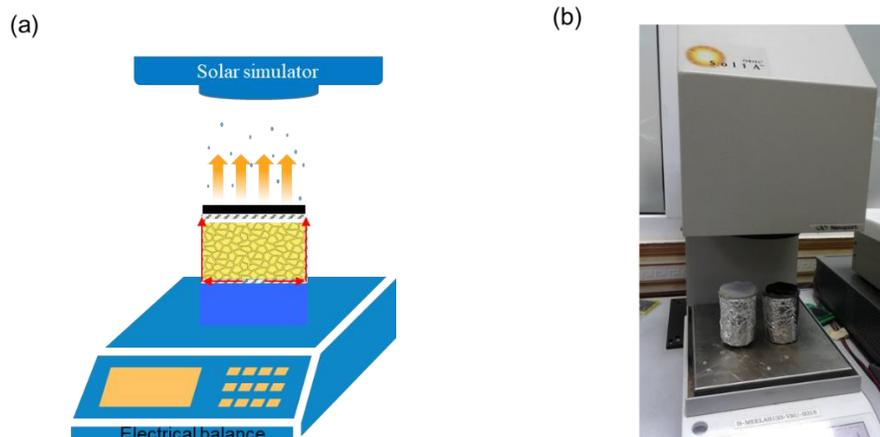
**Figure S6.** (a) schematic illustration and (b) photograph of the BTF-based SSG system.
