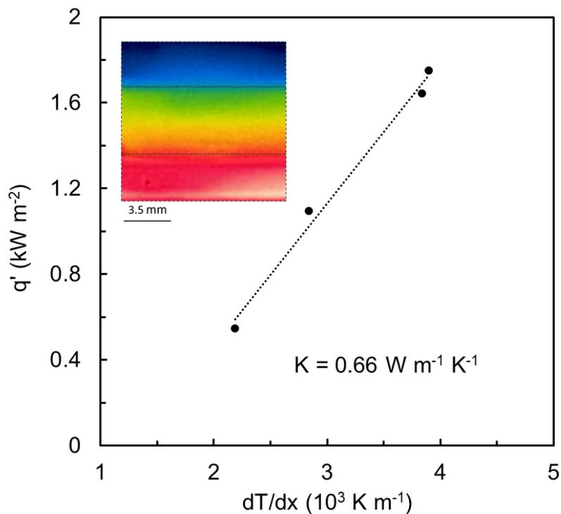
**Figure S8.** Thermal conductivity of the BTF material in wet state.
