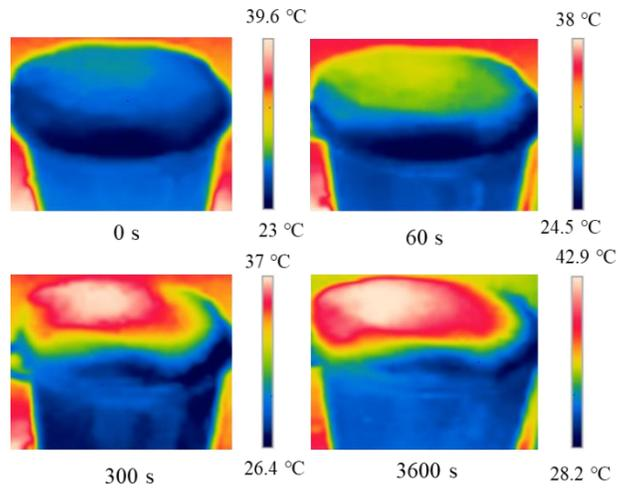
**Figure S7.** IR images of the surface of the SSG system under 1 sun illumination during evaporation process.
