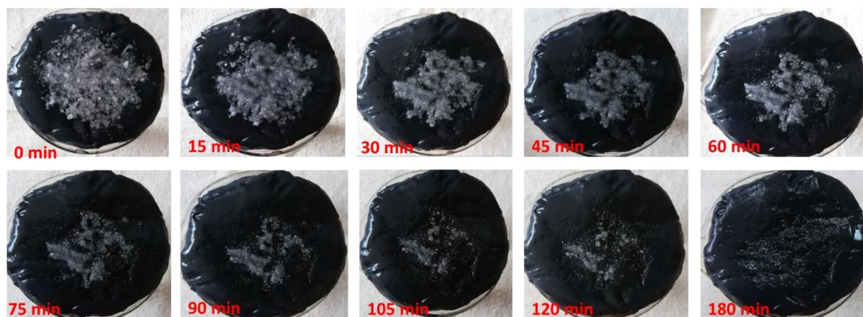
**Figure S9.** The self-cleaning process in the BTF surface over time.
